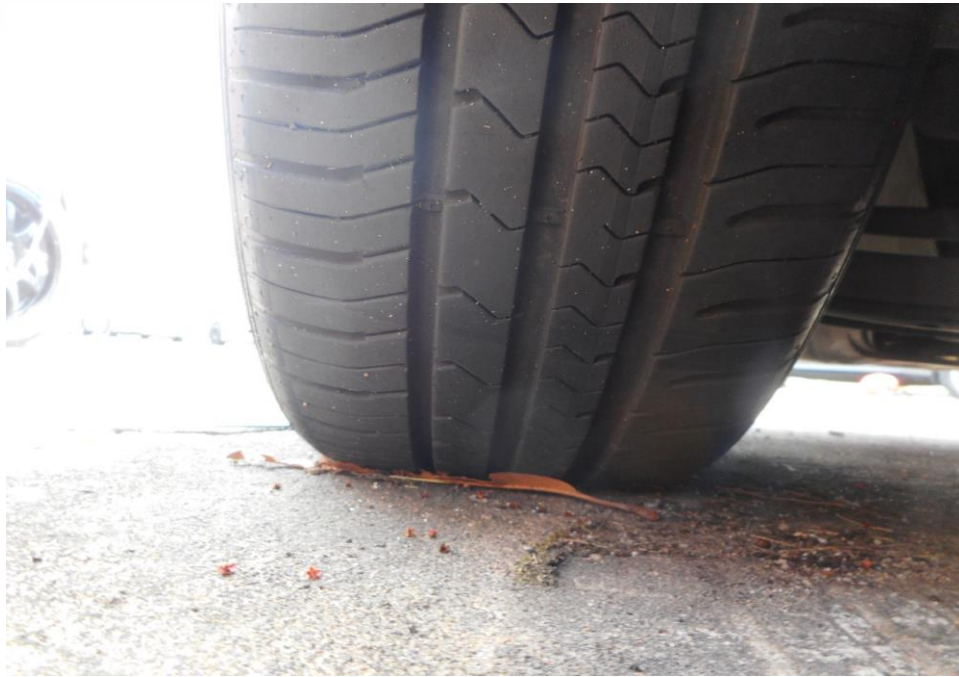
Photo 10 shows the condition of the front left tyre of the Motor Car, which was observed to be in serviceable condition with remaining tread depth of approximately 3.9mm. There was also no tear, cut or burst mark(s) on the outer and the inner sidewalls as well as across the tread of the Motor Car's 4 tyres.
