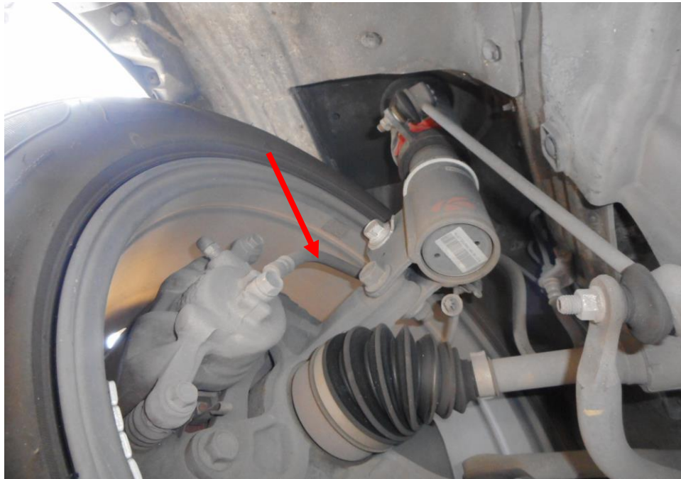
Photo 18 shows the brake hose/pipe (arrowed) at the front right wheel of the Motor Car. I did not observe any leakage of brake fluid at the time of my inspection of the Motor Car. Static tests of the Motor Car's braking system had indicated that there was no internal leakage of pressure/vacuum. The undercarriage components of the Motor Car were also all found to be intact and without any visible damage.
