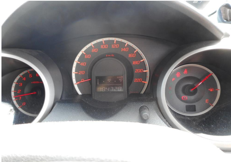
Photo 24 shows no warning lights illuminated on the instrument panel of the Motor Car after the engine was cranked. This would suggest that there was no abnormality to the electronic operating system of the Motor Car, like the ABS, EPS and SRS etc.
