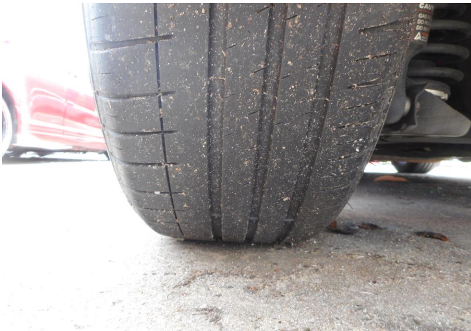
Photo 9 shows the condition of the rear left tyre of the Motor Car, which was observed to be in serviceable condition with remaining tread depth of approximately 3.7mm. The tyre, which was wrapped around steel wheel rim, was also observed to be sufficiently inflated for vehicular operation. The 4 tyres of the Motor Car were wrapped around standard steel wheel rims.
