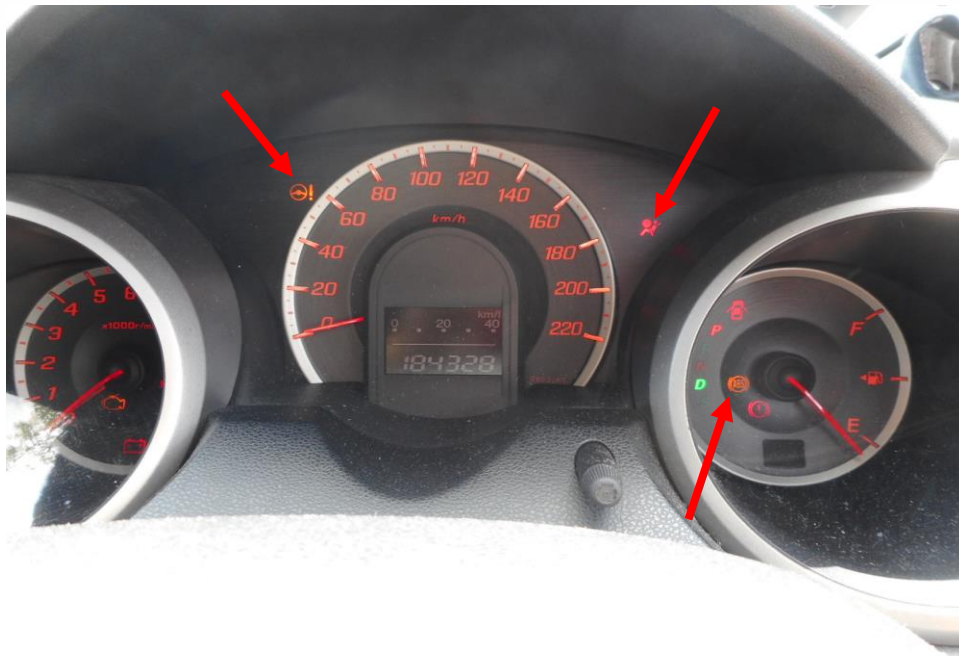
Photo 23 shows the warning light for Anti-Lock Brake System (ABS) and Power Steering System (EPS) and Supplemental Restraint System (SRS) (arrowed) appearing on the instrument panel of the Motor Car during the self-test of its various electronic operating systems when its engine was cranked.
