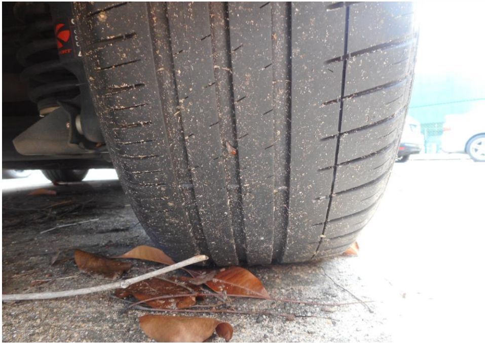
Photo 8 shows the condition of the rear right tyre of the Motor Car, which was observed to be in serviceable condition with remaining tread depth of approximately 4.3mm. The tyre was also observed to be sufficiently inflated for vehicular operation with no tear, cut or burst mark(s).
