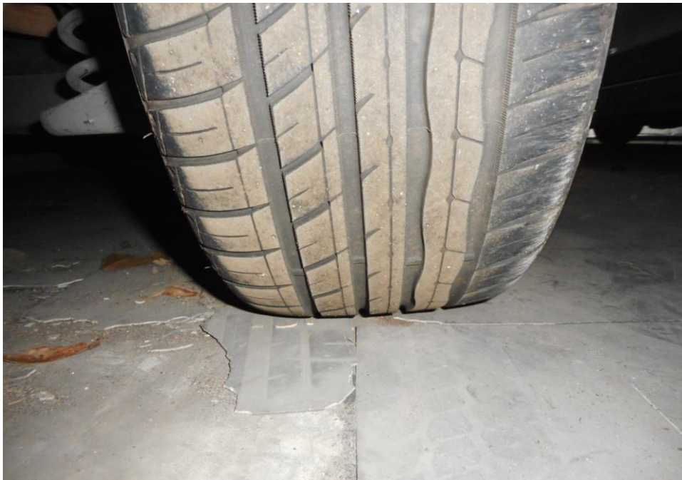
Photo 10 shows the condition of the rear right tyre of the Motor Car, which was observed to be in serviceable condition with remaining tread depth of approximately 5.1mm. The tyre was also observed to be sufficiently inflated for vehicular operation with no tear, cut or burst mark(s).
