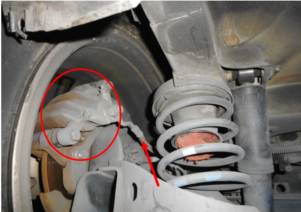
Photo 20 shows the brake caplier (circled) and brake hose/pipe (arrowed) at the rear left wheel of the Motor Car and it was observed to be intact
