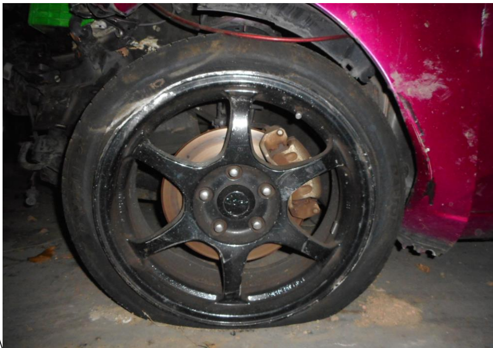
Photo 12 shows the condition of the front left tyre of the Motor Car, which was observed to be in unserviceable condition with remaining tread depth of approximately 4.7mm. The tyre was also observed to slip off the wheel rim and deflated as a result of the accident.
