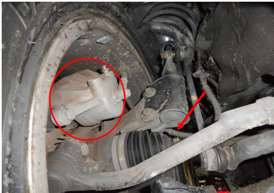
Photo 23 shows the brake hose/pipe (arrowed) at the front left wheel of the Motor Car. No leakage of brake fluid was observed. Visual examination of the various components of the braking system like the brake caliper (circled) had revealed all to be intact and without visible damage at the time of accident. There was also no sign of fluid stain(s) observed on the various undercarriage components.
