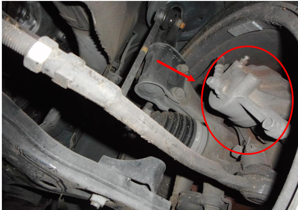
Photo 22 shows the brake hose/pipe (arrowed) at the front right wheel of the Motor Car. No leakage of brake fluid was observed. Visual examination of the various components of the braking system like the brake caliper (circled) had revealed to be intact and without visible damage at the time of accident. There was also no sign of fluid stain(s) observed on the various undercarriage components.
