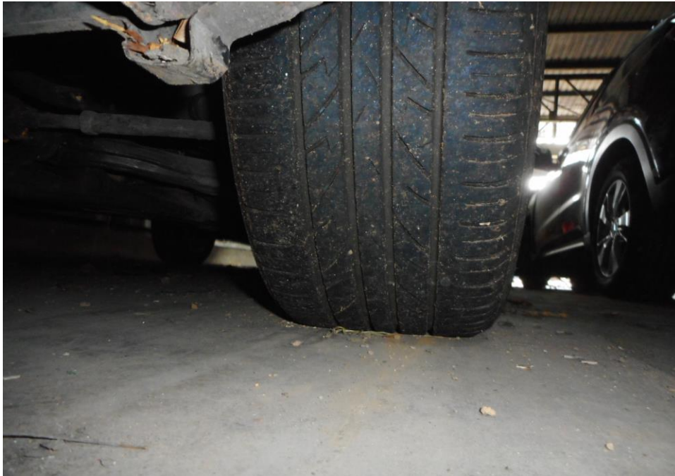
Photo 9 shows the condition of the front right tyre of the Motor Car, which was observed to be in serviceable condition with remaining tread depth of approximately 4.9mm. The tyre was also observed to be sufficiently inflated for vehicular operation with no tear, cut or burst mark(s).
