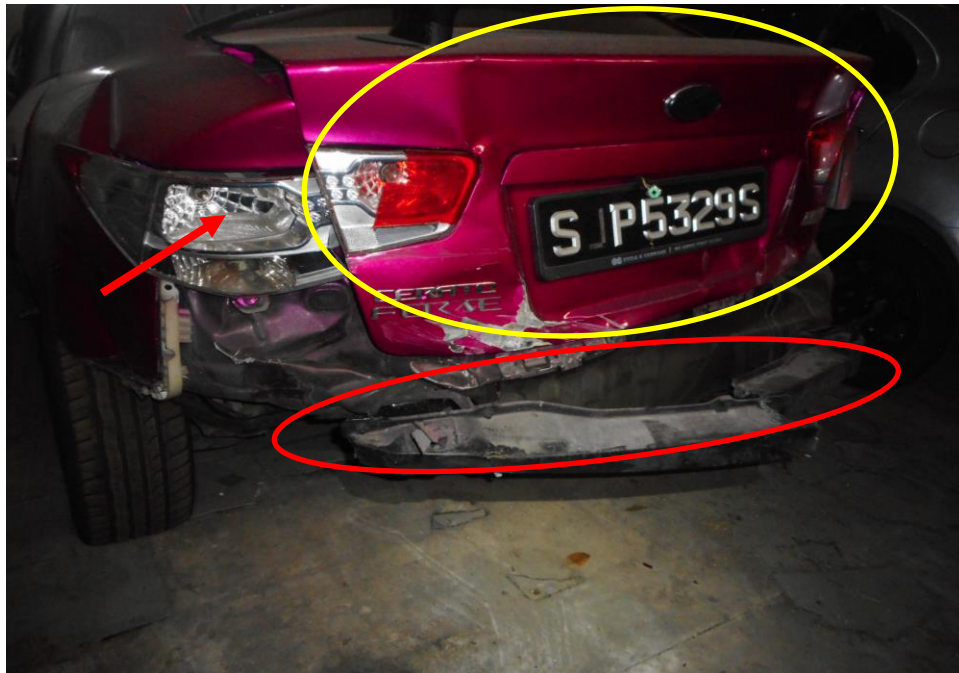
Photo 2 shows a general view of the Motor Car's rear body at the time of my inspection. Its rear bumper (red circle), rear bonnet (yellow circle) and its left right brake lamp (arrowed) was amongst the body parts that were also damaged as a result of the accident.
