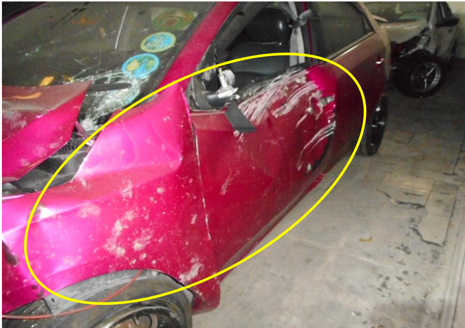
Photo 8 shows the close up view of the Motor Car's left body at the time of my inspection. The Motor car was observed to have sustained damage at its left portion. Its left body panel (circled) was damaged as a result of the accident.
