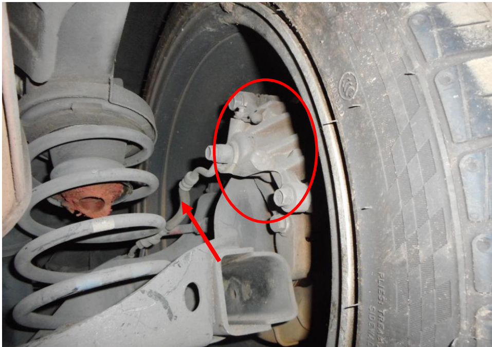
Photo 21 shows the brake caplier (circled) brake hose/pipe (arrowed) at the rear right wheel of the Motor Car and it was observed to be intact
