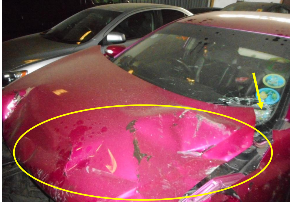
Photo 3 shows a general view of the Motor Car's front body at the time of my inspection. Its front windscreen (arrowed) and front bonnet (yellow circle) was amongst the body parts and various components in the engine compartments were also damaged as a result of the accident.
