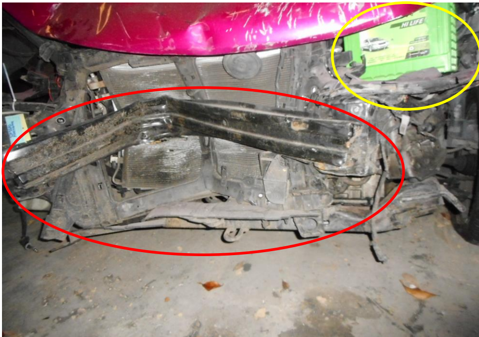
Photo 4 shows the close up view of the Motor Car's front body at the time of my inspection. The Motor car was observed to have sustained damage at its front portion. Its battery (yellow circle), front bumper and body reinforcement panel (red circle) was amongst the various components in the engine compartments were also damaged as a result of the accident.
