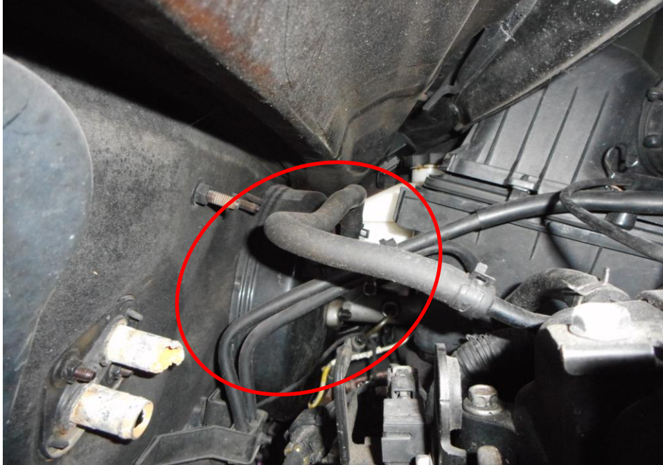
Photo 19 shows the brake booster of the Motor Car at the time of my inspection. The brake booster (circled) was observed to be crushed as a result of the induced impact from accident.
