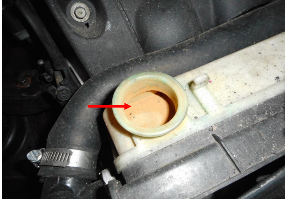
Photo 16 shows checks being carried out to the engine coolant of the Motor Car at the time of my inspection. The engine coolant was observed to be of insufficient level (arrowed) likely due to the damaged to the front radiator which caused the leakage of coolant.
