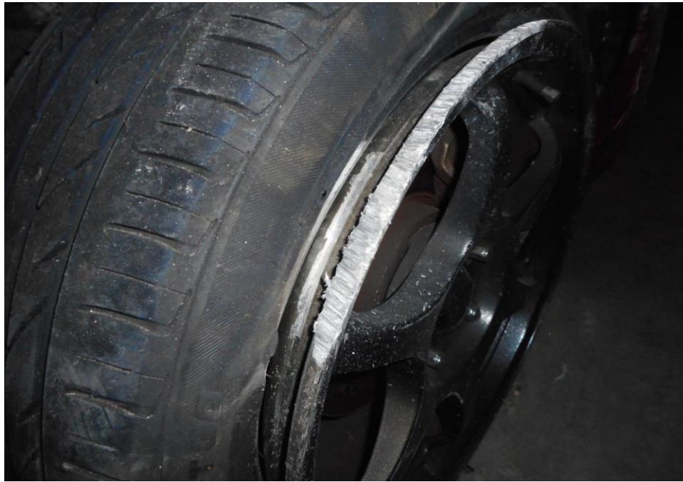
Photo 13 shows the condition of the front left tyre and rim of the Motor Car, the wheel rim was observed to slip off the wheel rim as a result of the accident
