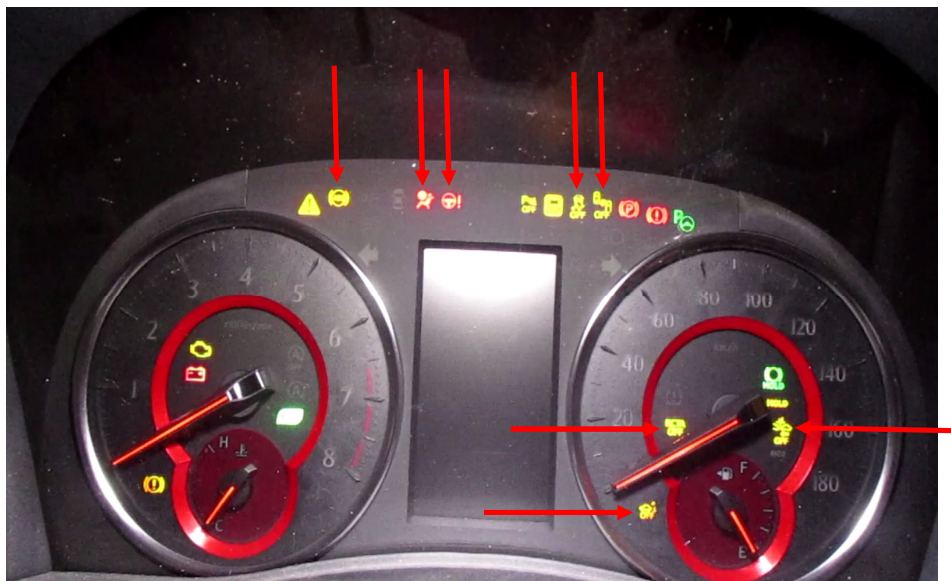
Photo 14 shows the warning lights for the various electronic safety features appearing on the instrument panel of the Motor Car during its self-test when the engine is cranked, in particular the lights for the ABS, SRS, EPS, VSC and various pre-collision systems (arrowed).
