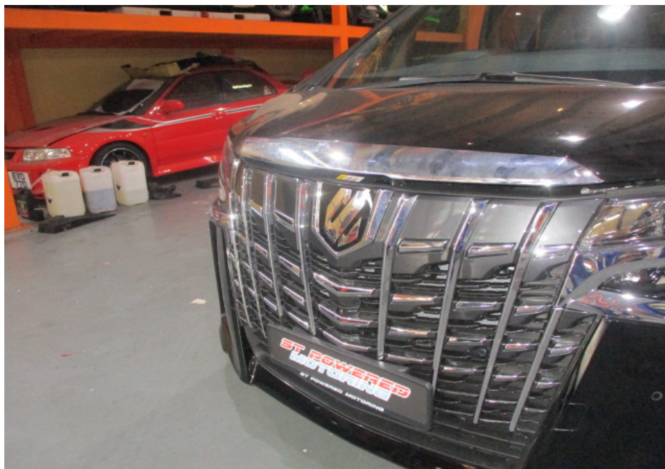
Photo 6 shows a closer view of the front bumper, front bonnet, front bonnet chrome moulding, front grille and front left headlamp of the Motor Car at the time of my inspection. The body parts at the frontal portion of the Motor Car were visually examined and it was observed that the repair/restoration works carried out to the damaged area of the Motor Car (refer to photograph 1 & 2 above) were reasonably adequate and in order.
