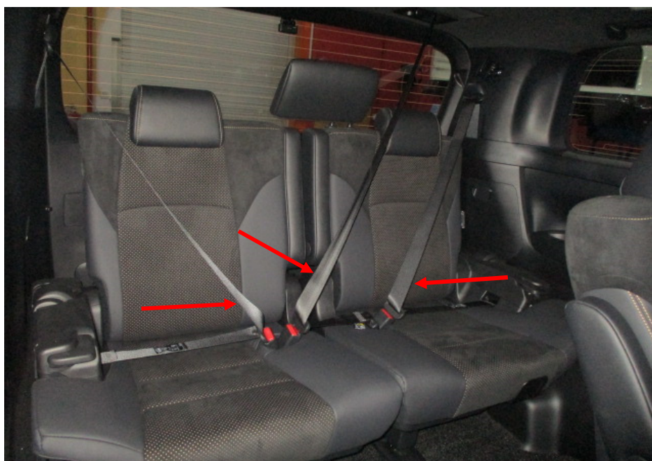
Photo 13 shows the rear seats at the 2 nd row of the Motor Car. All the seats of the Motor Car were secured via seat rails to the floorboard. They were also fitted with a retractable seat belt reel and a pre-tensioner. The seat belts (arrowed) were tested and were able to be fastened into the respective pre-tensions that were fitted on the side of each individual seat.
