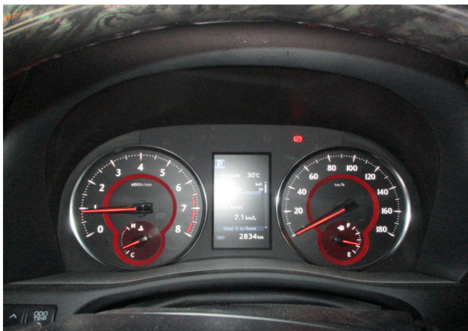
Photo 15 shows the respective warning lights no longer illuminated, indicating that there is no fault detected to the ABS, SRS, EPS, VSC and various pre-collision systems of the Motor Car during the self-test. These electronic systems were hence in working condition at the time of my inspection.
