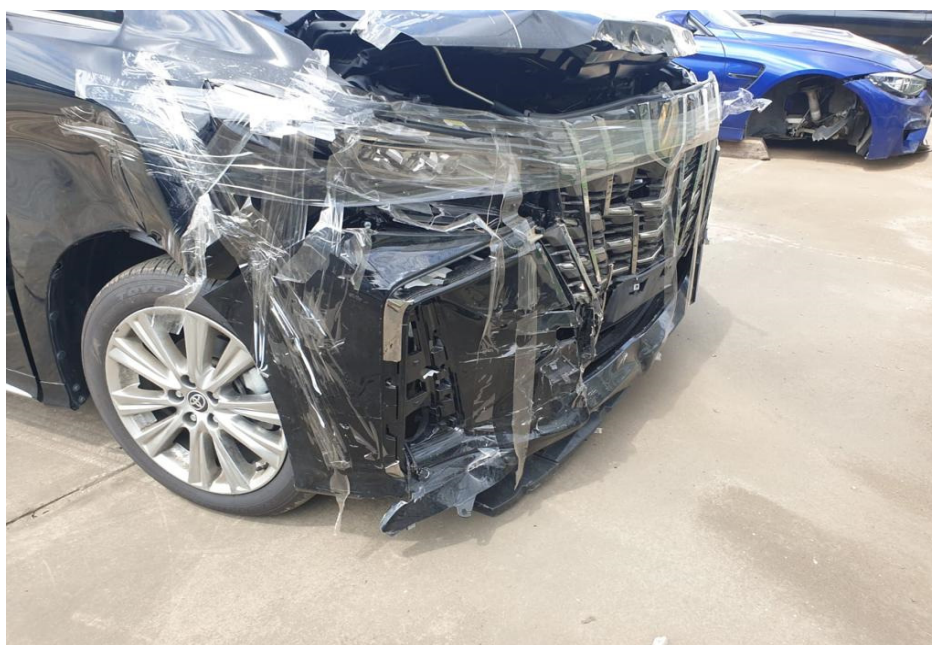
Photo 2 shows the front right body of the Motor Car (photograph provided to me). The Motor Car was observed to have sustained damage at its frontal portion. The front bumper, front bumper right lower chrome moulding, front right fog lamp, front right fog lamp garnish, front grille, front bonnet, front right fender and front right headlamp were amongst the body parts that were observed to have been damaged.
