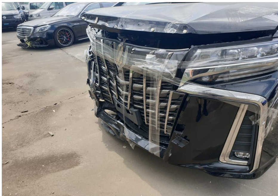
Photo 1 shows the front left body of the Motor Car (photograph provided to me). The Motor Car was observed to have sustained damage at its frontal portion. The front bumper, front bumper number plate garnish, front grille, front bonnet and front bonnet chrome moulding were amongst the body parts that were observed to have been damaged.
