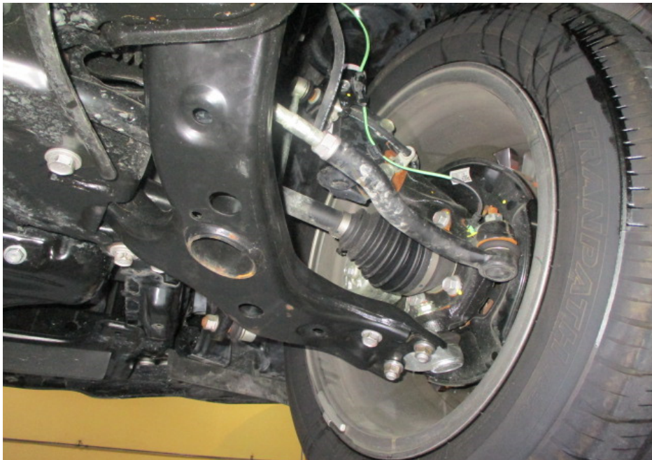
Photo 19 shows the various undercarriage components at the front right wheel of the Motor Car. The mechanical components, control arms and linkages were all found to be intact and secured in an appropriate manner. I also did not observe any fluid leak and/or fluid stain on the underside of the Motor Car.
