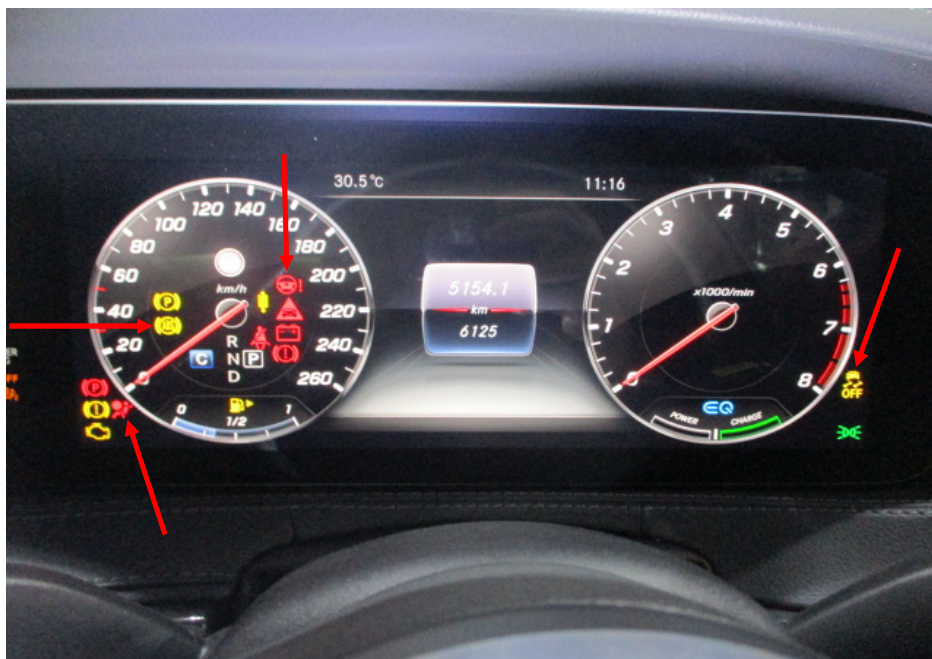
Photo 13 shows the warning lights for the various electronic safety features appearing on the instrument panel of the Motor Car during its self-test when the engine is cranked, in particular the ABS, SRS, EPS and TCS lights (arrowed).
