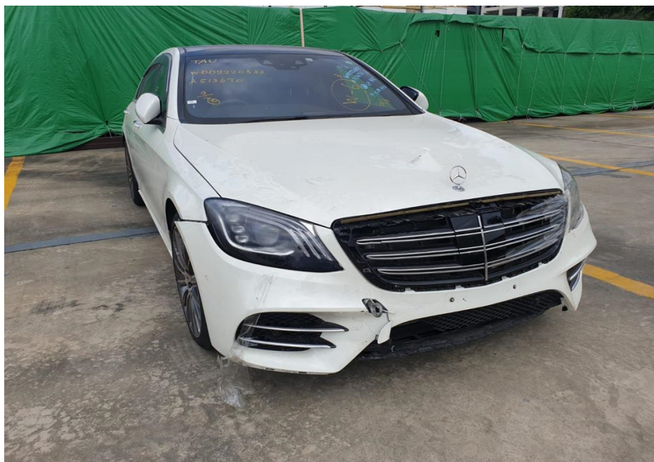
Photo 2 shows the front right body of the Motor Car (photograph provided to me). The Motor Car was observed to have sustained damage at its frontal portion. The front bumper, front bumper lower chrome moulding, front bumper centre lower grille, front grille, front bonnet and front undercover were amongst the body parts that were observed to have been damaged.
