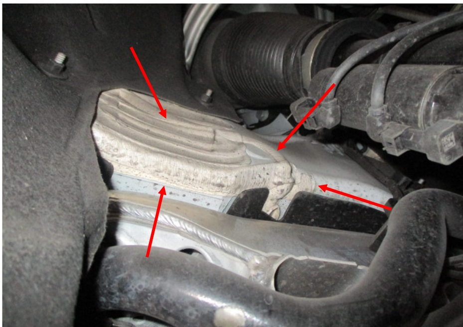
Photo 21 shows the chassis/structural body at the underside front right of the Motor Car. The original factory sealant (arrowed) at the joints along the chassis/structural body was observed to be untouched. In general, I had found no work was carried out on the chassis/structural body of the Motor Car. The chassis/structural body of the Motor Car was originally fitted.
