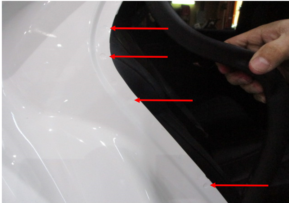
Photo 22 shows the right side "C" pillar of the Motor Car. I did not find any weld marks other than original spot weld marks (arrowed) on the right side "C" pillar of the Motor Car, which indicates that there was no re-welding works carried out. In general, I had found all the non-detachable body panels of the Motor Car to be originally fitted at the time of my inspection.
