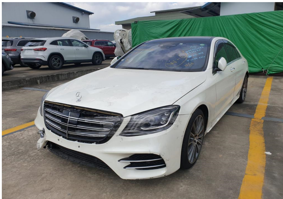
Photo 1 shows the front left body of the Motor Car (photograph provided to me). The Motor Car was observed to have sustained damage at its frontal portion. The front bumper, front bumper lower chrome moulding, front bumper centre lower grille, front bumper number plate garnish and front undercover were amongst the body parts that were observed to have been damaged.
