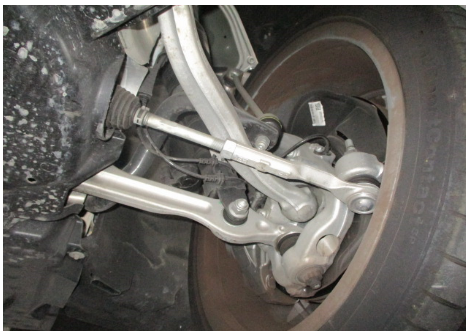
Photo 17 shows the various undercarriage components at the front left wheel of the Motor Car. The mechanical components, control arms and linkages were all found to be intact and secured in an appropriate manner.
