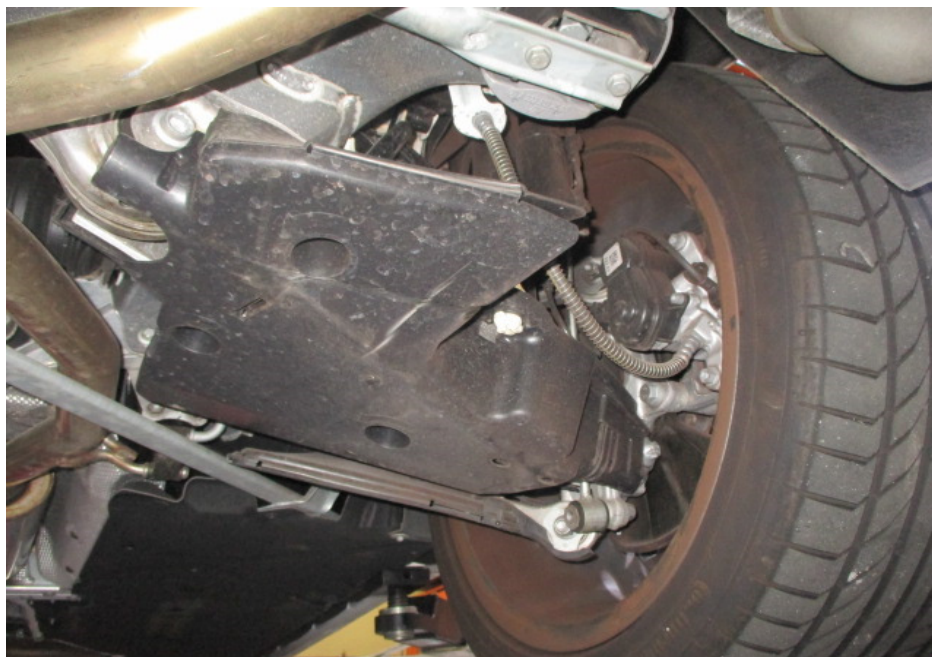
Photo 16 shows a general view of the control arms and linkages at the rear right wheel of the Motor Car. I did not observe any fluid leak and/or fluid stain on the underside of the Motor Car. All of the Motor Car's undercarriage components were observed to be intact and secured in an appropriate manner.
