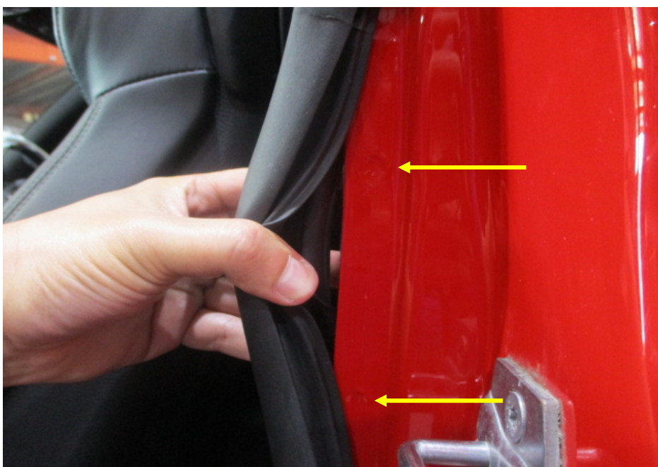
Photo 22 shows the left side rear body panel of the Motor Car. I did not find any weld marks other than original spot weld marks (arrowed) on the left side rear body panel of the Motor Car which, indicates that there was no re-welding works carried out. In general, I had found all the non-detachable body panels of the Motor Car to be originally fitted at the time of my inspection.
