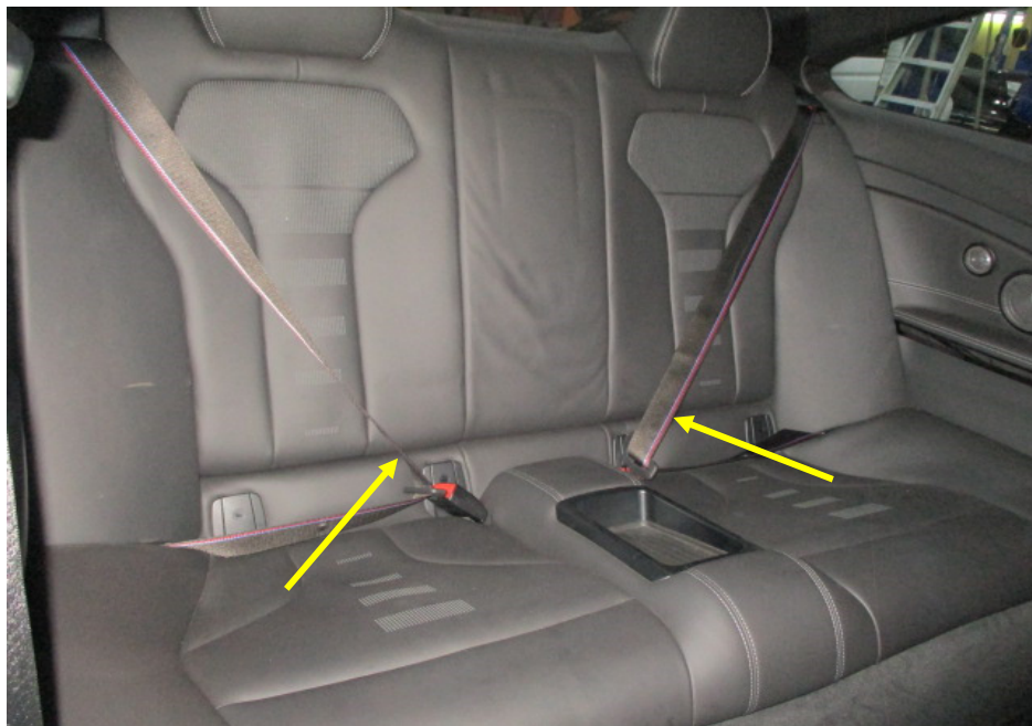
Photo 12 shows the seats of the Motor Car, which were secured via seat rails (arrowed) to the floorboard. All the seats of the Motor Car were fitted with a retractable seat belt reel and pre-tensioner. The seat belts (arrowed) were tested and were able to be fastened into the respective pre-tensions that were fitted on the side of each individual seat.
