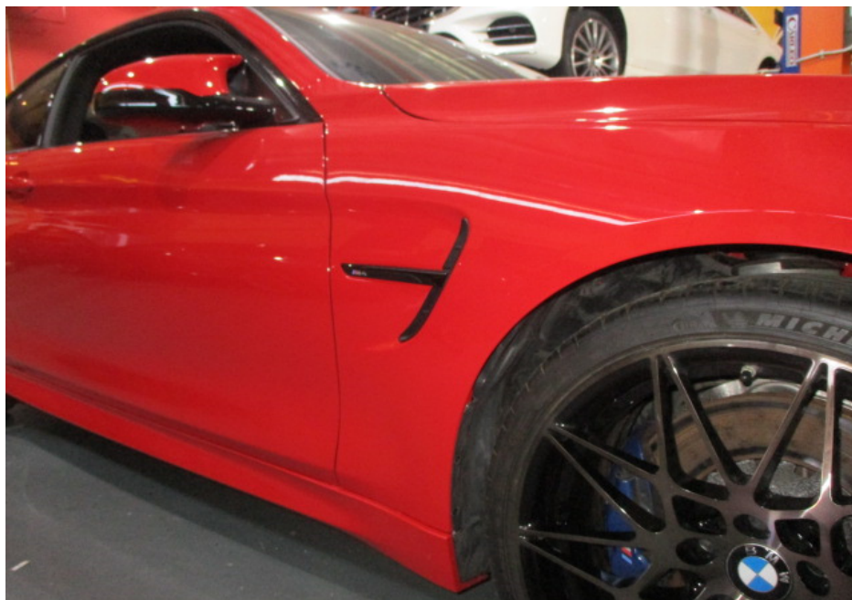
Photo 7 shows a closer view of the front right fender and front right wheel rim of the Motor Car at the time of my inspection. The body parts at the right front portion of the Motor Car were visually examined and it was observed that the repair/restoration works carried out to the damaged area of the Motor Car (refer to photograph 1 above) were reasonably adequate and in order.
