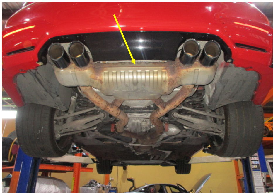
Photo 19 shows the Motor Car's rear muffler (arrowed). My examination of the Motor Car's exhaust system revealed no sign(s) or indication(s) of any cut or weld marks along its exhaust pipes and on its catalytic converters.
