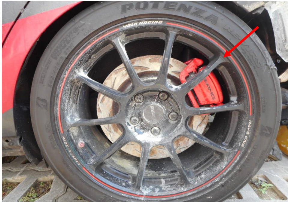
Photo 9 shows an aftermarket rim (arrowed) on the Insured Vehicle, which was observed to be unaffected by the fire.
