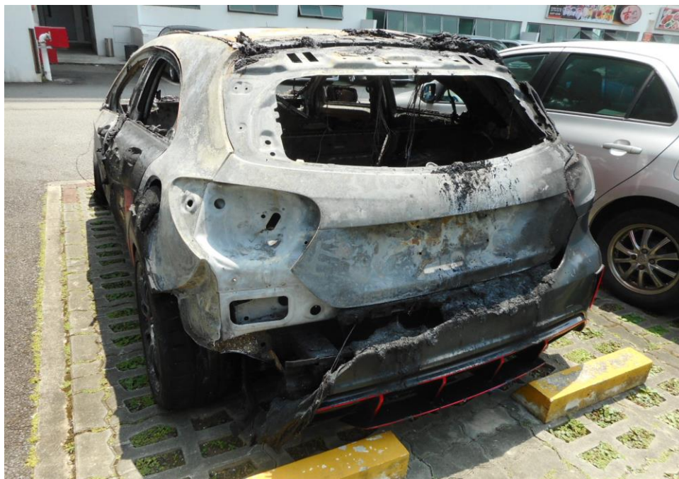
Photo 6 shows the general view of the rear portion of the Insured Vehicle which was observed to be affected heat and smoke damage at the time of our inspection as a result of the fire.
