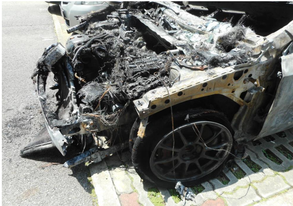
Photo 15 shows the general view of the exterior of the front left fender of the Insured Vehicle at the time of our inspection. The high heat intensity burn marks (whitish burn marks) and rust that had development found on the exterior surface of the bonnet indicates that the fire had originated from the front left portion of the Insured Vehicle.
