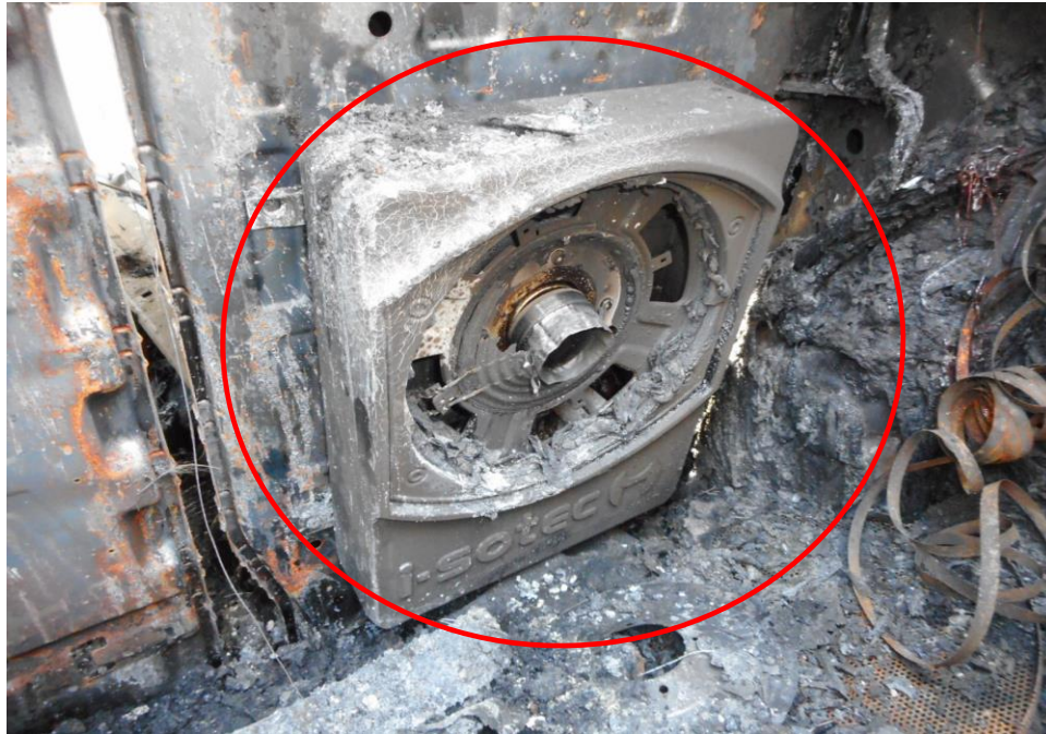
Photo 11 shows the close up view of the aftermarket subwoofer (circled) on the Insured Vehicle, which was observed to be damaged by the fire.
