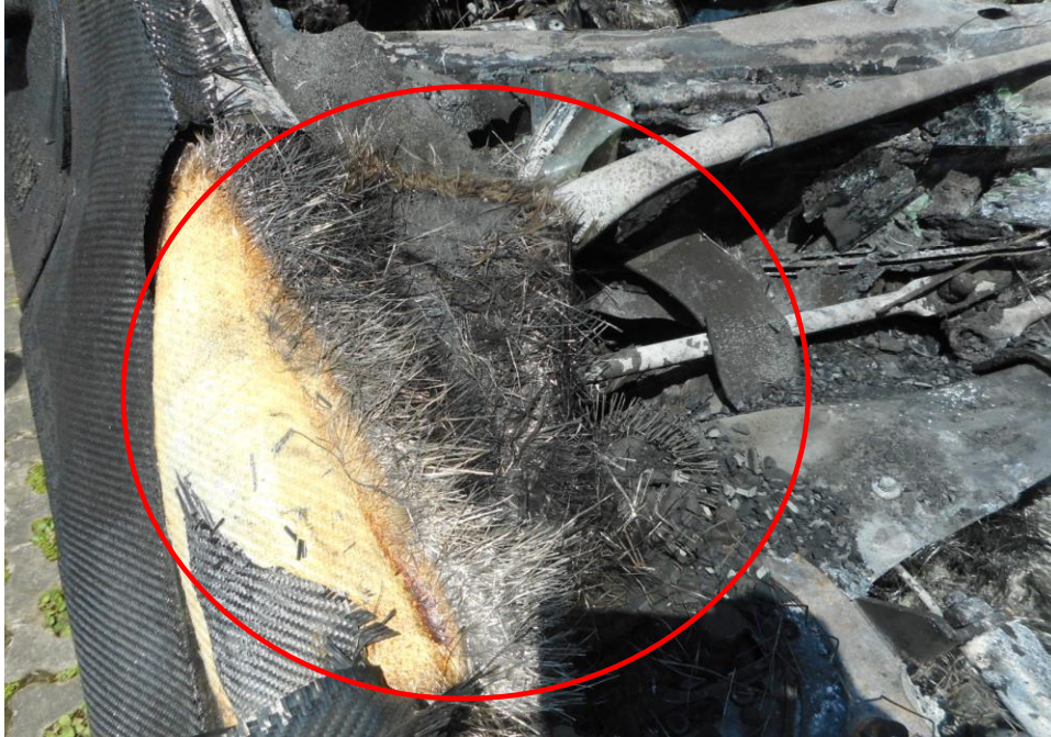
Photo 13 shows the close up view of the aftermarket carbon fibre bonnet and fenders (circled) on the Insured Vehicle, which was observed to be damaged by the fire.
