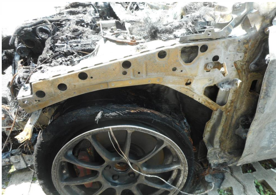
Photo 16 shows the close up view of the exterior of the front left fender of the Insured Vehicle at the time of our inspection. The high heat intensity burn marks (whitish burn marks) and rust that had development found on the exterior surface of the front left fender indicates that the fire had likely originated from the front left portion of the Insured Vehicle.
