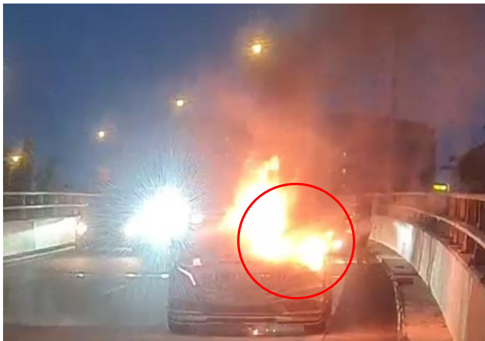
Photo 21 shows the fire started burning from the front left side of the engine compartment (circled) of the Insured Vehicle at Bartley flyover. In general, the information that could be gathered from this photograph had corresponded to the events that were related to us by Mr Lim, location when the fire broke out.
