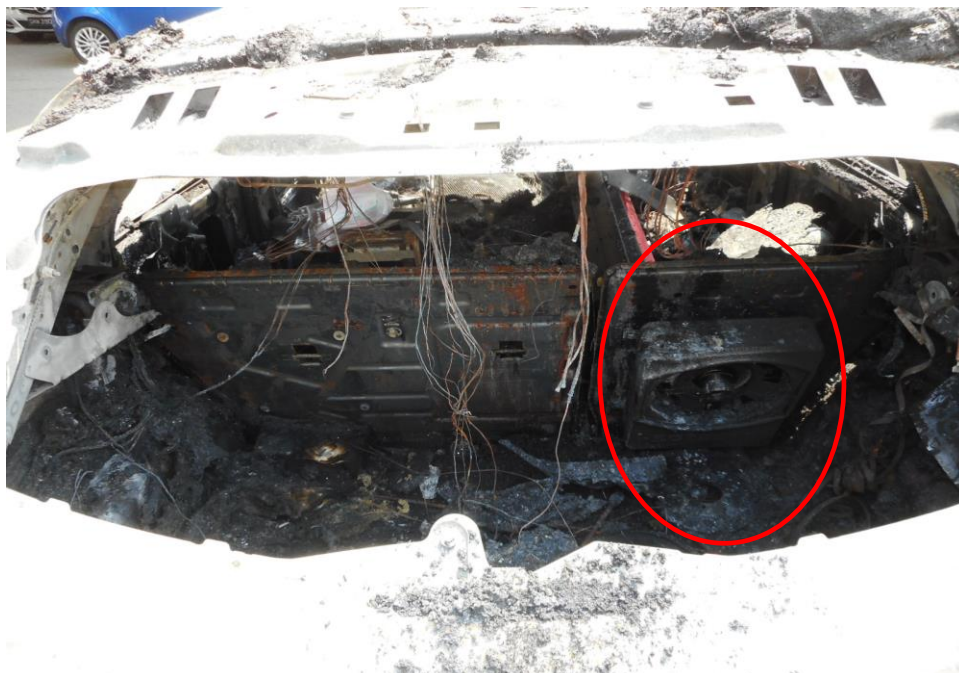
Photo 10 shows a general view of the aftermarket subwoofer (circled) on the Insured Vehicle, which was observed to be damaged by the fire.
