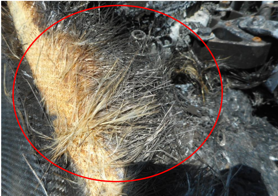
Photo 14 shows the close up view of the aftermarket carbon fibre bonnet and fenders (circled) on the Insured Vehicle, which was observed to be damaged by the fire.
