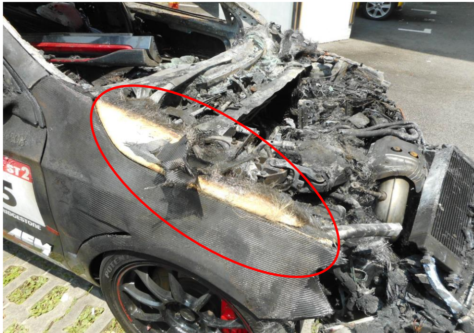
Photo 12 shows the general view of the aftermarket carbon fibre bonnet and fenders (circled) on the Insured Vehicle, which was observed to be damaged by the fire.
