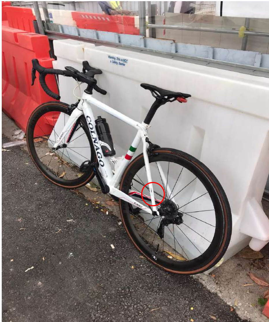
Photo 7 shows the bicycle post- accident which was taken by Mr Leow. The photographs had showed damages to the bicycle at the left portion of the rear frame (circled).
