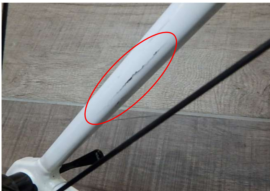
Photo 12 shows a crack on the right portion of the rear frame of the bicycle (circled).
