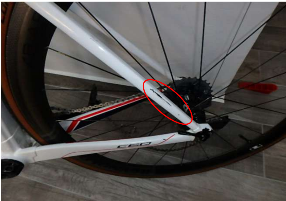
Photo 10 shows a closer view of the black marks on the left portion of the rear frame of the bicycle (circled).
