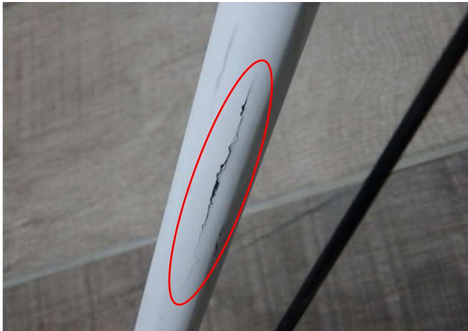
Photo 13 shows a close up view of the crack on the right portion of the rear frame of the bicycle (circled).
