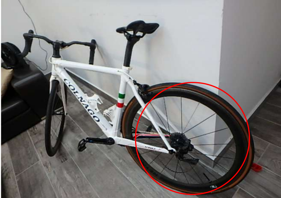
Photo 9 shows the general view of the left portion of the bicycle at the time of the Pre- Repair Survey conducted by LKK Auto Consultants Pte. Ltd. The damage to the bicycle was observed to be confined around the rear wheel rim and frame (circled).
