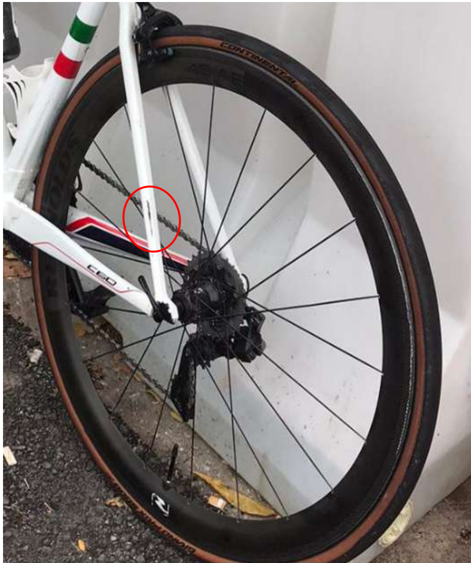
Photo 8 shows a closer view of the damages to the bicycle at the left portion of the rear frame post- accident. Upon closer examination, we observed black marks on the left portion of the rear frame of the bicycle (circled).
