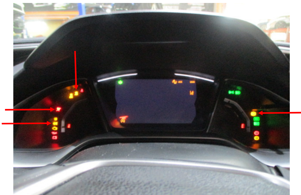
Photo 14 shows the warning lights for the various electronic safety features appearing on the instrument panel of the Motor Car during its self-test when the engine is cranked, in particular the ABS, SRS, EPS and SC lights (arrowed).
