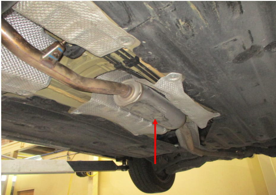
Photo 20 shows the Motor Car's centre resonator (arrowed). My examination of the Motor Car's exhaust system revealed no sign(s) or indication(s) of any cut or weld marks along its exhaust pipes, on its catalytic converter and on its rear muffler.
