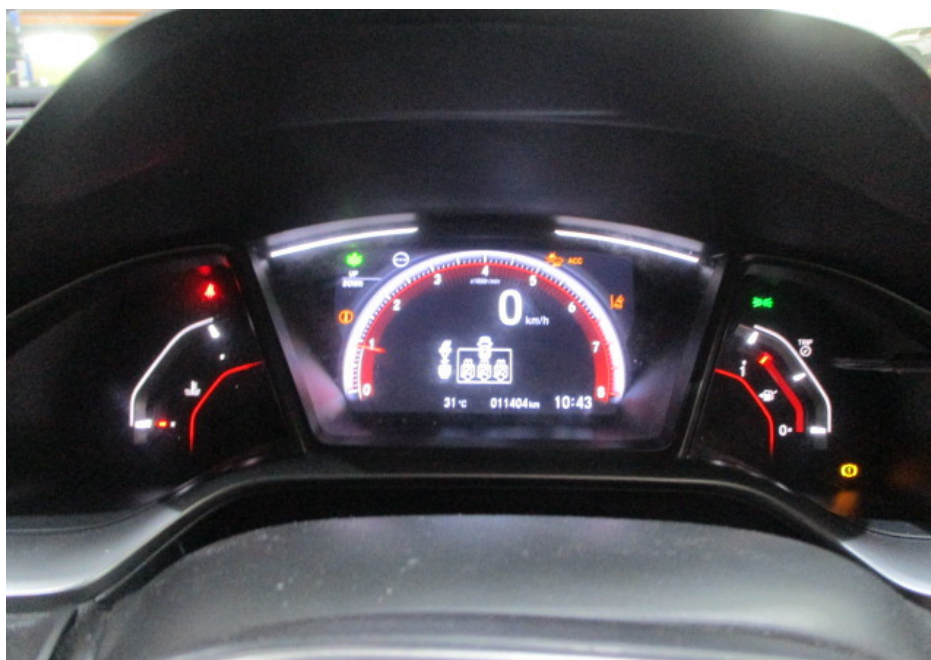
Photo 15 shows the respective warning lights no longer illuminated, indicating that there is no fault detected to the ABS, SRS, EPS and SC systems of the Motor Car during the self-test. These electronic systems were hence in working condition at the time of my inspection.
