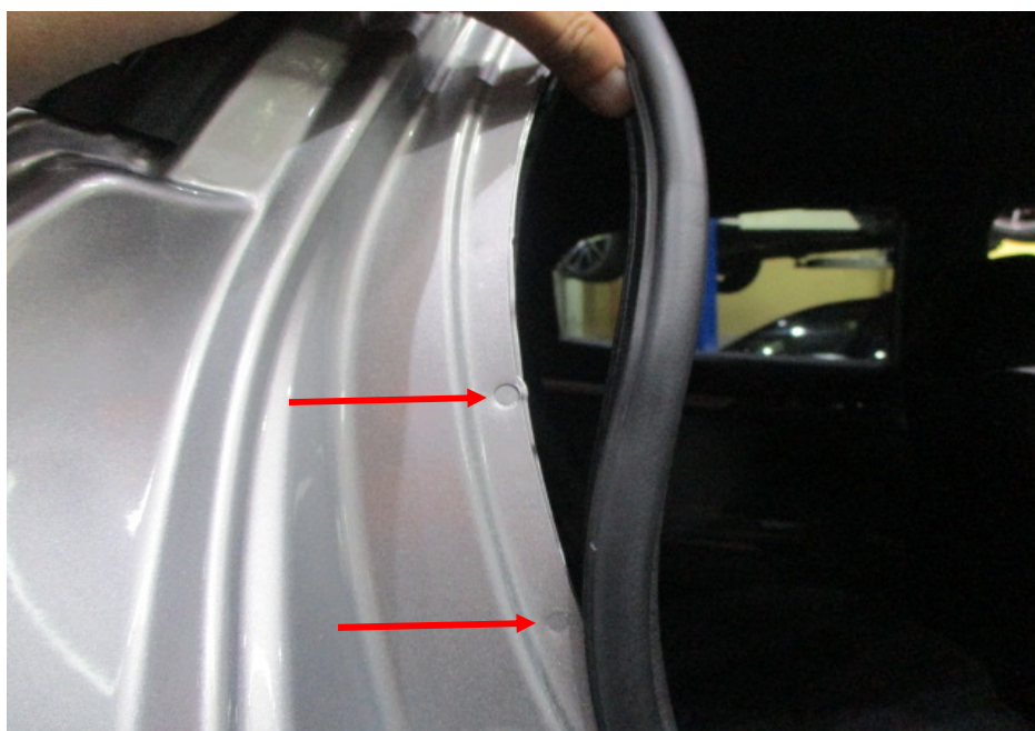
Photo 23 shows the right side "C" pillar of the Motor Car. I did not find any weld marks other than original spot weld marks (arrowed) on the right side "C" pillar of the Motor Car which, indicates that there was no re-welding works carried out. In general, I had found all the non-detachable body panels of the Motor Car to be originally fitted at the time of my inspection.
