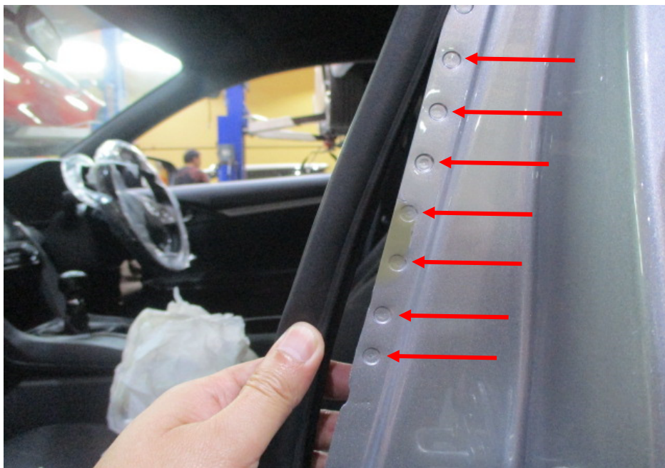
Photo 24 shows the left side "B" pillar of the Motor Car. I did not find any weld marks other than original spot weld marks (arrowed) on the left side "B" pillar of the Motor Car which, indicates that there was no re-welding works carried out. In general, I had found all the non-detachable body panels of the Motor Car to be originally fitted at the time of my inspection.
