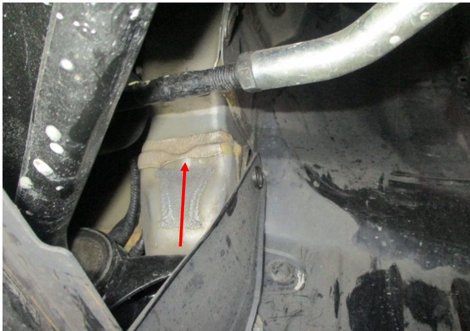
Photo 21 shows the chassis/structural body at the underside front left of the Motor Car. I did not find any weld marks other than original spot weld marks on the chassis/structural body of the Motor Car. The original factory sealant (arrowed) at the joints along the chassis/structural body was untouched, indicating no work was done on the chassis/structural body of the Motor Car and that the chassis/structural body was originally fitted.
