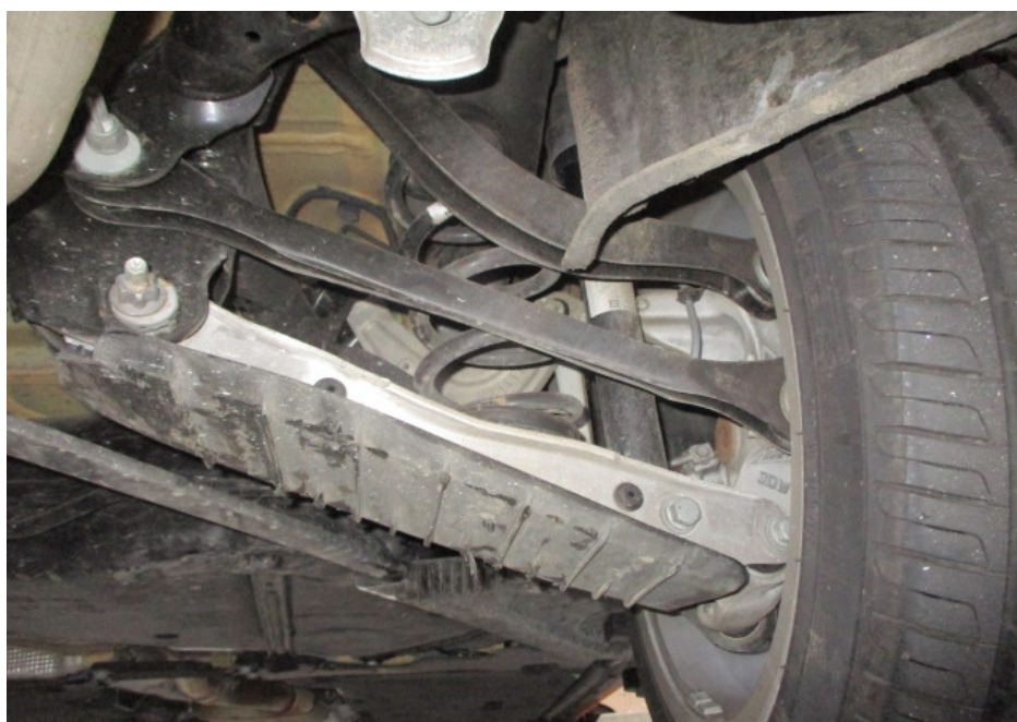
Photo 18 shows the various undercarriage components at the rear right wheel of the Motor Car. The mechanical components, control arms and linkages were all found to be intact and secured in an appropriate manner.
