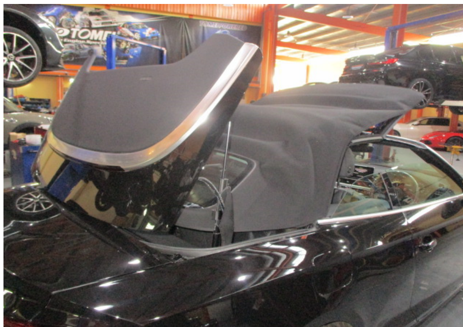
Photo 10 shows the Motor Car's soft top being tested. It was observed that as a safety feature, the soft top could only open and close when the Motor Car was in a stationary position. When opened, the soft top is completely folded into the rear boot compartment with no parts protruding out of the Motor Car's body. It was also observed that during the folding and unfolding process, the soft top roof did not extend laterally beyond the Motor Car's body.
