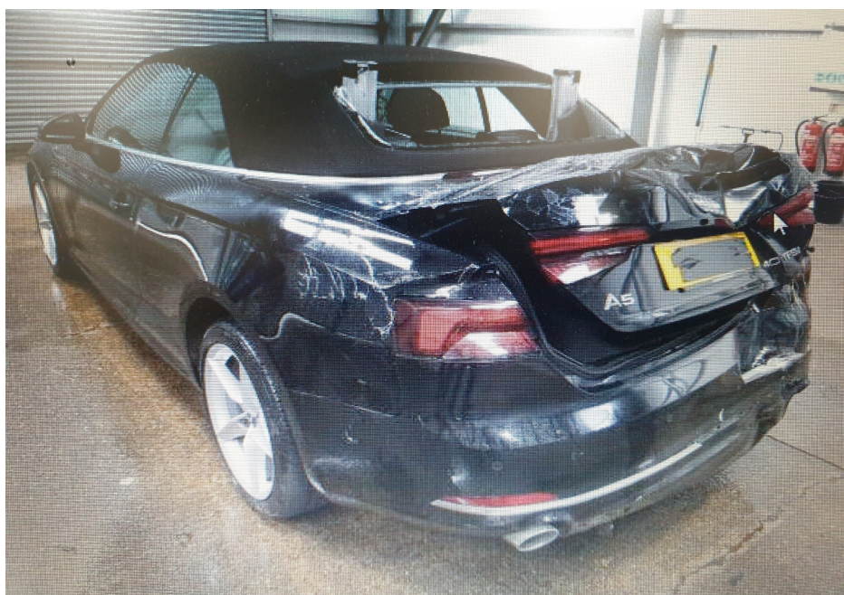
Photo 2 shows the rear left body of the Motor Car (photograph provided to me). The Motor Car was observed to have sustained damage at its rear portion. The rear bumper, rear bumper lower cover, rear left body panel, rear left taillamp, rear bootlid, rear left bootlid lamp and rear windshield were amongst the body parts that were observed to have been damaged.
