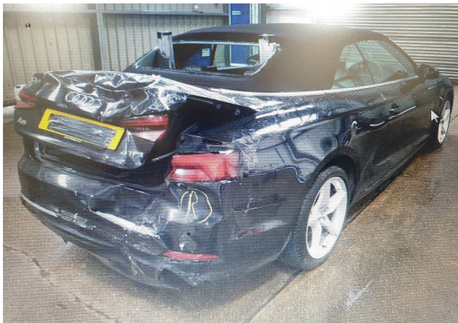
Photo 1 shows the rear right body of the Motor Car (photograph provided to me). The Motor Car was observed to have sustained damage at its rear portion. The rear bumper, rear bumper lower cover, rear bumper reinforcement, rear right taillamp, rear bootlid, rear right bootlid lamp and rear right exhaust were amongst the body parts that were observed to have been damaged.
