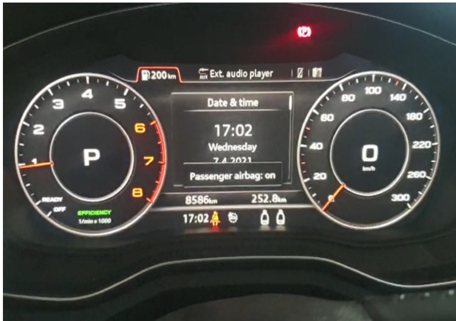
Photo 15 shows the respective warning lights no longer illuminated, indicating that there is no fault detected to the ABS, SRS, EPS, TPM and ESC systems of the Motor Car during the self-test. These electronic systems were hence in working condition at the time of my inspection.
