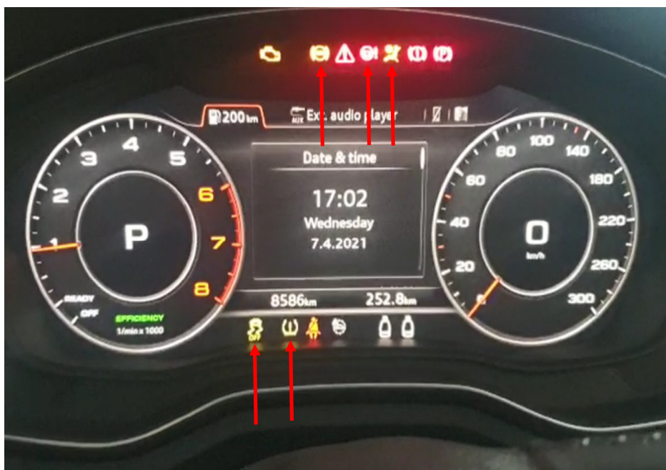
Photo 14 shows the warning lights for the various electronic safety features appearing on the instrument panel of the Motor Car during its self-test when the engine is cranked, in particular the ABS, SRS, EPS, TPM and ESC lights (arrowed).
