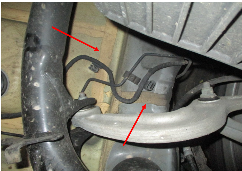
Photo 22 shows the chassis/structural body at the underside rear right of the Motor Car. The original factory sealant (arrowed) at the joints along the chassis/structural body was observed to be untouched. In general, I had found no work was carried out on the chassis/structural body of the Motor Car. The chassis/structural body of the Motor Car was originally fitted.
