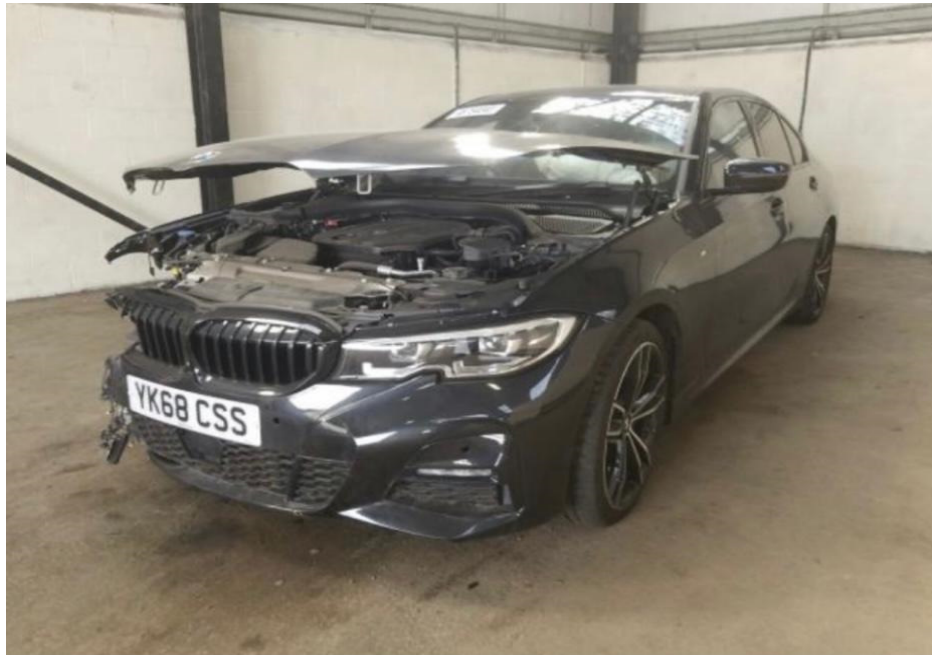
Photo 1 shows the front left body of the Motor Car (photograph provided to me). The Motor Car was observed to have sustained damage at its front right portion. The front bumper, front bonnet and bonnet hinges were amongst the body parts that were observed to have been damaged.
