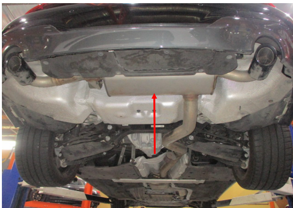
Photo 19 shows the Motor Car's rear muffler (arrowed). My examination of the Motor Car's exhaust system revealed no sign(s) or indication(s) of any cut or weld marks along its exhaust pipes and on its catalytic converter.
