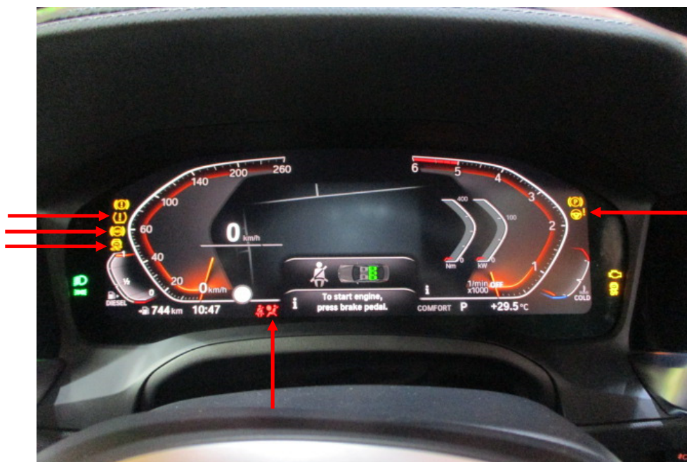
Photo 13 shows the warning lights for the various electronic safety features appearing on the instrument panel of the Motor Car during its self-test when the engine is cranked, in particular the ABS, SRS, IAS, TPM and DSC lights (arrowed).
