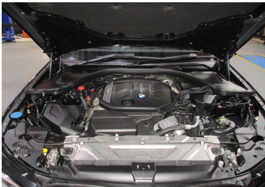
Photo 11 shows a general view of the engine compartment of the Motor Car at the time of my inspection. The various parts and components inside the engine compartment were all observed to be intact and properly fitted. There was also no sign(s) or indication(s) of fluid leak and/or fluid stain found within the engine compartment.
