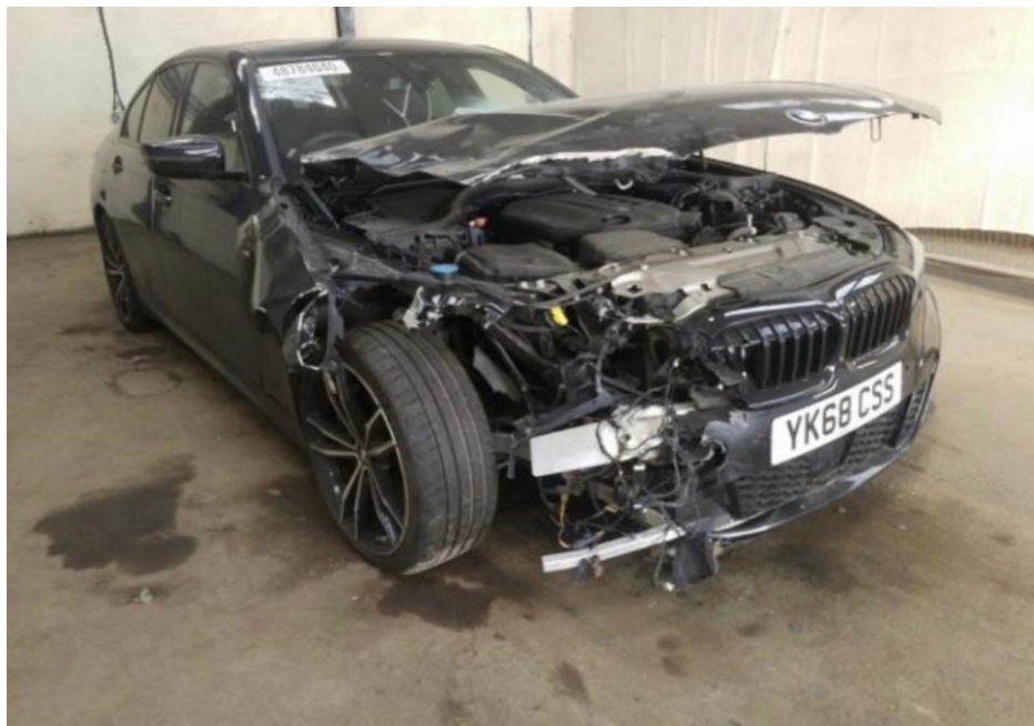
Photo 2 shows the front right body of the Motor Car (photograph provided to me). The Motor Car was observed to have sustained damage at its front right portion. The front bumper, front bumper right lower grille, front bumper reinforcement, front grilles, front right headlamp, front right headlamp top panel, front bonnet, front bonnet hinges, front support panel, air ducts and front right fender were amongst the body parts that were observed to have been damaged.
