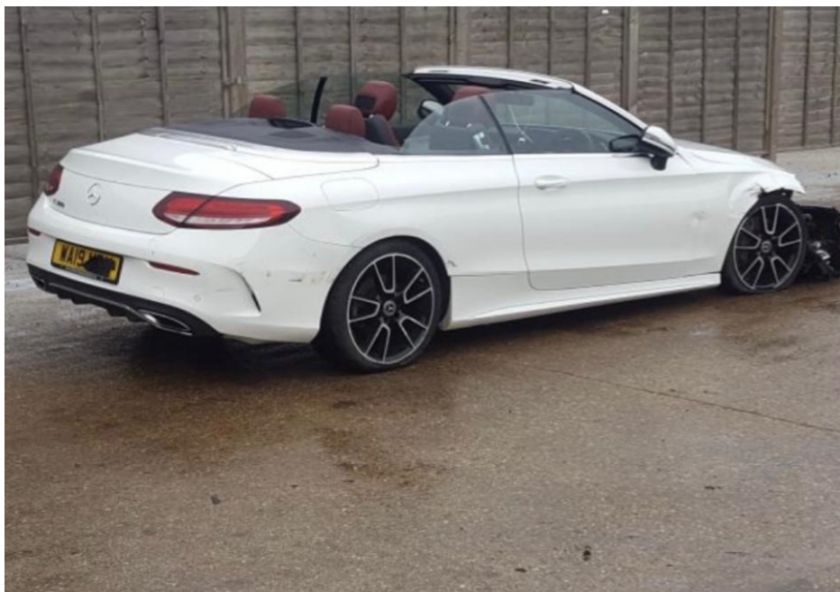
Photo 3 shows the rear right body of the Motor Car (photograph provided to me). Apart for the front right portion, there was no physical damage seen to other areas of the Motor Car. The airbags of the Motor Car were also not activated as seen from the photographs that were provided to me.
