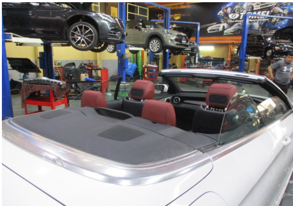
Photo 12 shows the Motor Car's with its soft top completely folded. It was observed that as a safety feature, the soft top could only open and close when the Motor Car was in a stationary position. When opened, the soft top is completely folded into the rear boot compartment with no parts protruding out of the Motor Car's body. The soft top was also found adequately secured to the "A" pillar after closing.
