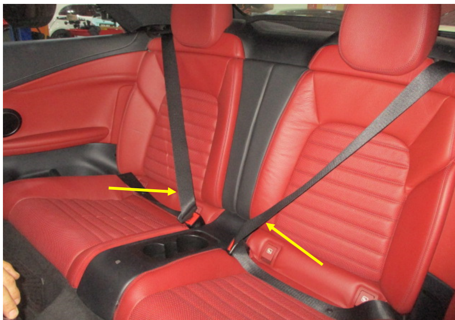
Photo 14 shows the rear seats of the Motor Car. All the seats of the Motor Car were secured via seat rails to the floorboard. They were also fitted with a retractable seat belt reel and a pre-tensioner. The seat belts (arrowed) were tested and were able to be fastened into the respective pre-tensions that were fitted on the side of each individual seat.
