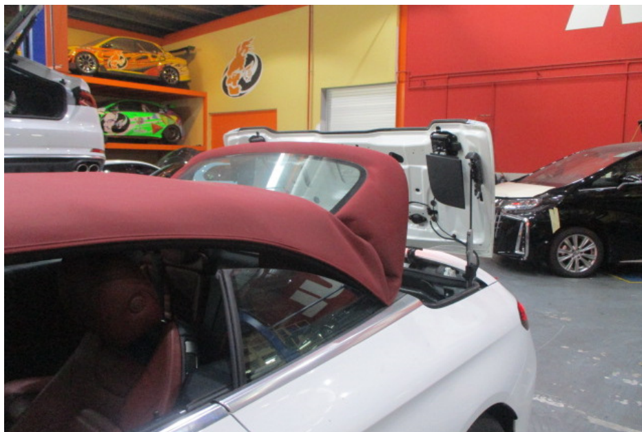
Photo 11 shows the Motor Car's soft top being tested. It was observed that as a safety feature, the soft top could only open and close when the Motor Car was in a stationary position. When opened, the soft top is completely folded into the rear boot compartment with no parts protruding out of the Motor Car's body. The soft top was also found adequately secured to the "A" pillar after closing.
