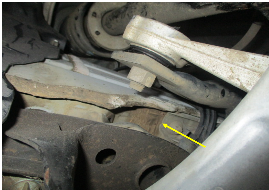
Photo 23 shows the chassis/structural body at the underside front right of the Motor Car. The original factory sealant (arrowed) at the joints along the chassis/structural body was observed to be untouched. In general, I had found no work was carried out on the chassis/structural body of the Motor Car. The chassis/structural body of the Motor Car was originally fitted.
