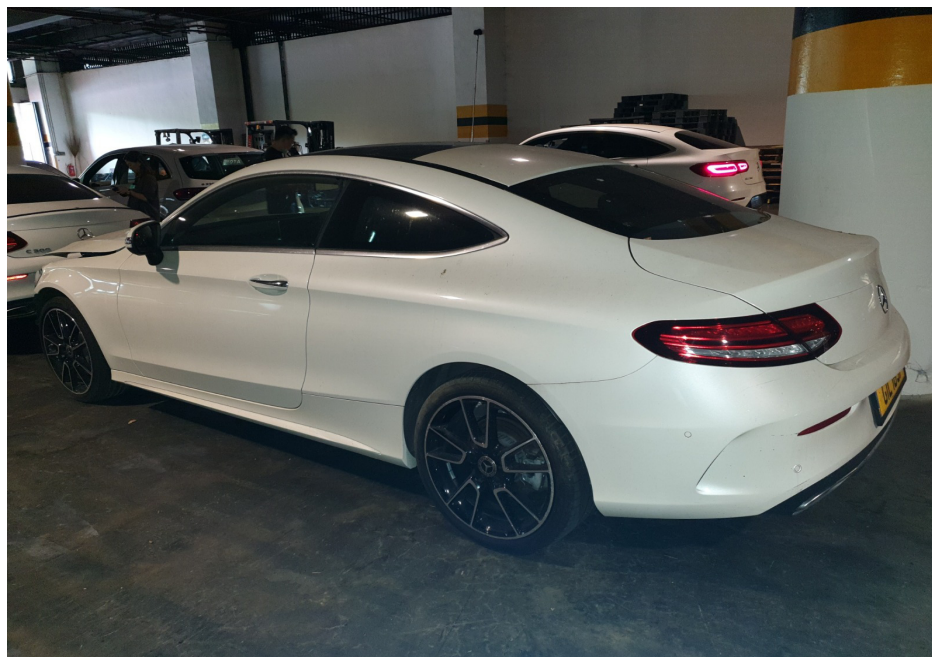
Photo 4 shows the rear left body of the Motor Car (photograph provided to me). Apart for the rear portion, there was no physical damage seen to other areas of the Motor Car. The airbags of the Motor Car were also not activated as seen from the photographs that were provided to me.
