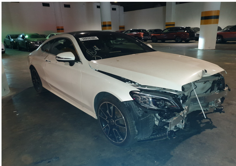
Photo 1 shows the front right body of the Motor Car (photograph provided to me). The Motor Car was observed to have sustained damage at its frontal portion. The front bumper and all its related parts and attachments, front bumper reinforcement, front bonnet, front right headlamp, aircon condenser and radiator were amongst the body parts that were observed to have been damaged.
