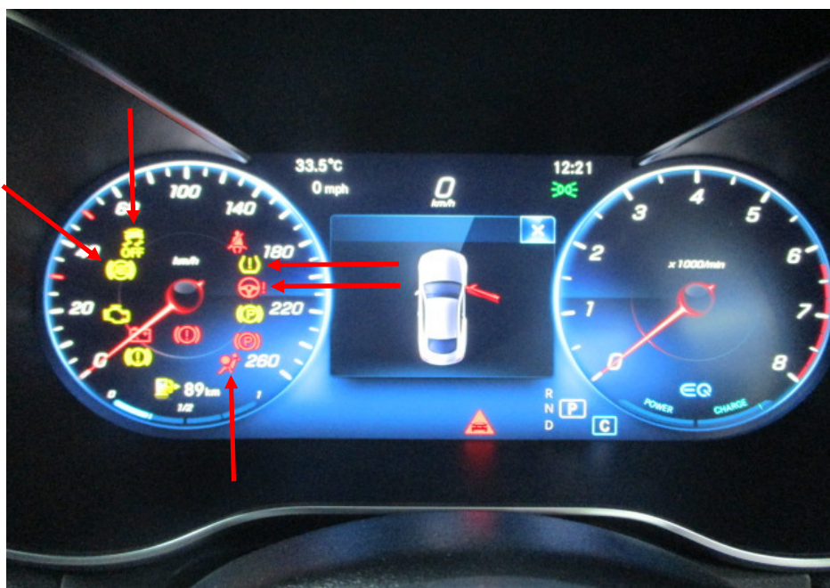
Photo 13 shows the warning lights for the various electronic safety features appearing on the instrument panel of the Motor Car during its self-test when the engine is cranked, in particular the ABS, SRS, EPS, TPM and TCS lights (arrowed).
