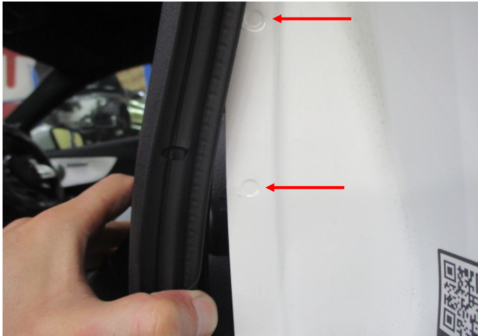
Photo 23 shows the left rear body panel of the Motor Car. I did not find any weld marks other than original spot weld marks (arrowed) on the left rear body panel of the Motor Car which, indicates that there was no re-welding works carried out. In general, I had found all the non-detachable body panels of the Motor Car to be originally fitted at the time of my inspection.
