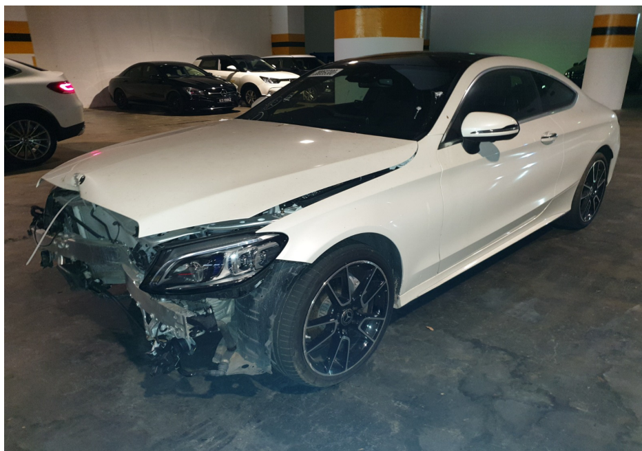
Photo 2 shows the front left body of the Motor Car (photograph provided to me). The Motor Car was observed to have sustained damage at its frontal portion. The front bumper and all its related parts and attachments, front bumper reinforcement, front bonnet, front left headlamp, aircon condenser and radiator were amongst the body parts that were observed to have been damaged.
