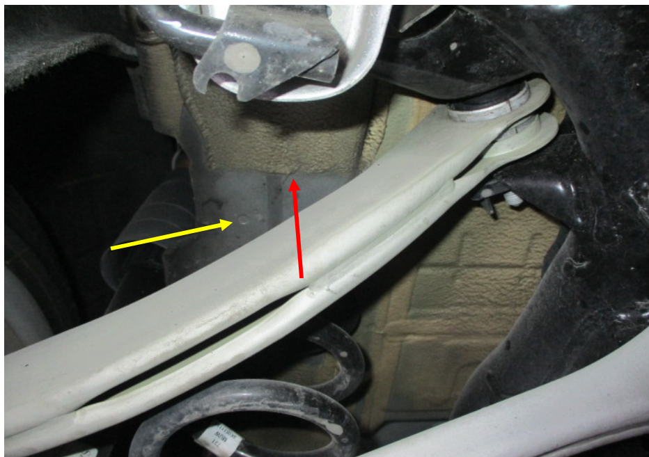
Photo 21 shows the chassis/structural body at the underside rear left of the Motor Car. I did not find any weld marks other than original spot weld marks (yellow arrow) on the chassis/structural body of the Motor Car. The original factory sealant (red arrow) at the joints along the chassis/structural body was untouched, indicating no work was done on the chassis/structural body of the Motor Car and that the chassis/structural body was originally fitted.
