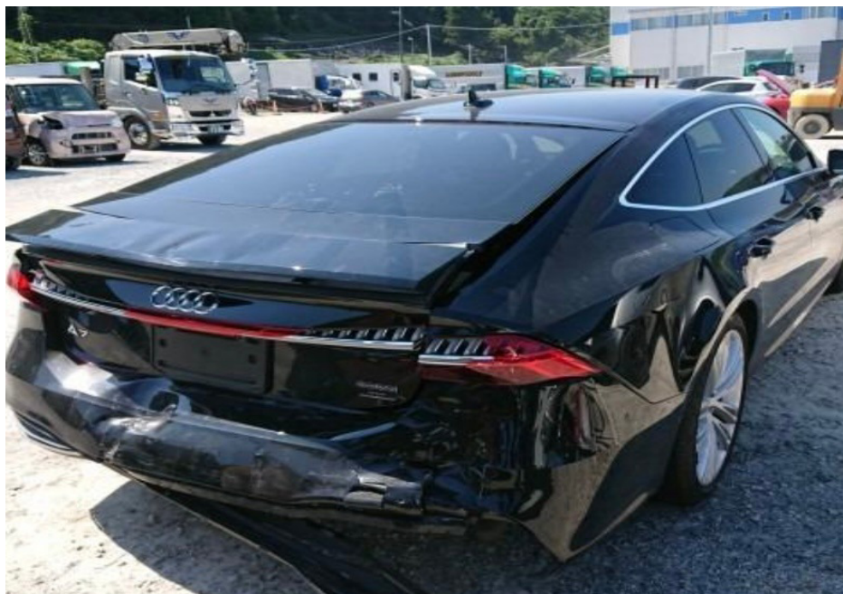
Photo 1 shows the rear right body of the Motor Car (photograph provided to me). The Motor Car was observed to have sustained damage at its rear portion. The rear bumper, rear bumper lower cover, rear taillamps, rear bootlid, rear bootlid lamp and rear bootlid spoiler were amongst the body parts that were observed to have been damaged.
