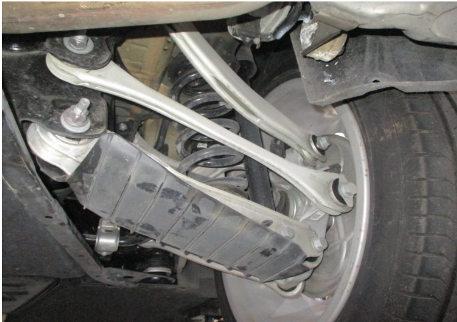
Photo 17 shows the various undercarriage components at the rear right wheel of the Motor Car. The mechanical components, control arms and linkages were all found to be intact and secured in an appropriate manner.
