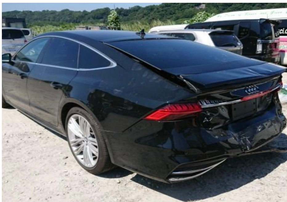
Photo 2 shows the rear left body of the Motor Car (photograph provided to me). The Motor Car was observed to have sustained damage at its rear portion. The rear bumper, rear bumper lower cover, rear taillamps, rear bootlid, rear bootlid lamp and rear bootlid spoiler were amongst the body parts that were observed to have been damaged.
