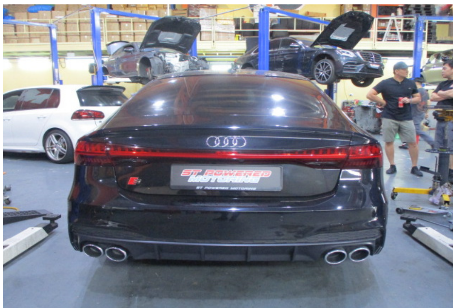
Photo 6 shows a general view of the rear body of the Motor Car at the time of my inspection. The Motor Car was observed to be in a relatively good general condition with no loose exterior fittings observed. The body parts at the rear portion of the Motor Car were visually examined and it was observed that the repair/restoration works carried out to the damaged area of the Motor Car (refer to photograph 1 & 2 above) were reasonably adequate and in order.
