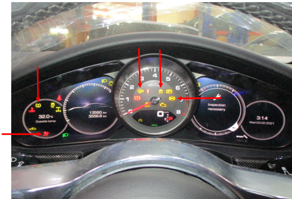
Photo 13 shows the warning lights for the various electronic safety features appearing on the instrument panel of the Motor Car during its self-test when the engine is cranked, in particular the ABS, SRS, PSS, TPM and PSM lights (arrowed).
