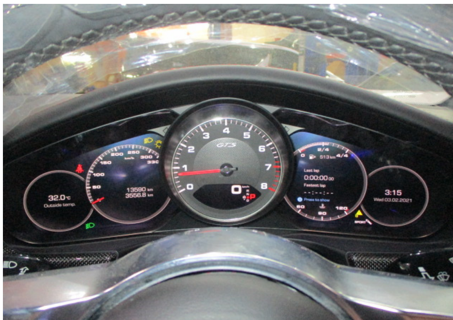
Photo 14 shows the respective warning lights no longer illuminated, indicating that there is no fault detected to the ABS, SRS, PSS, TPM and PSM systems of the Motor Car during the self-test. These electronic systems were hence in working condition at the time of my inspection.
