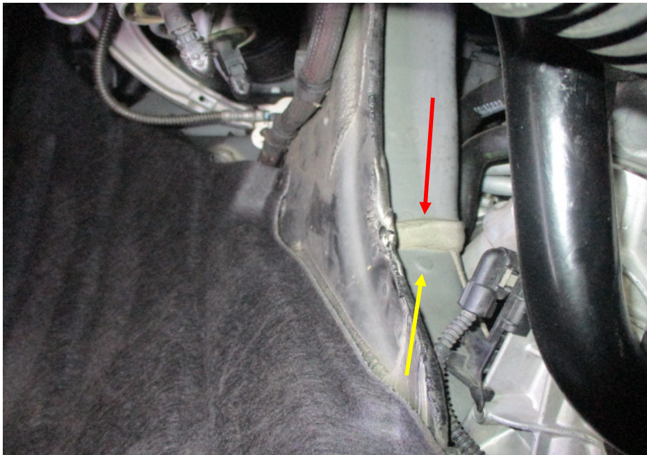
Photo 20 shows the chassis/structural body at the underside front right of the Motor Car. I did not find any weld marks other than original spot weld marks (yellow arrow) on the chassis/structural body of the Motor Car. The original factory sealant (red arrow) at the joints along the chassis/structural body was untouched, indicating no work was done on the chassis/structural body of the Motor Car and that the chassis/structural body was originally fitted.
