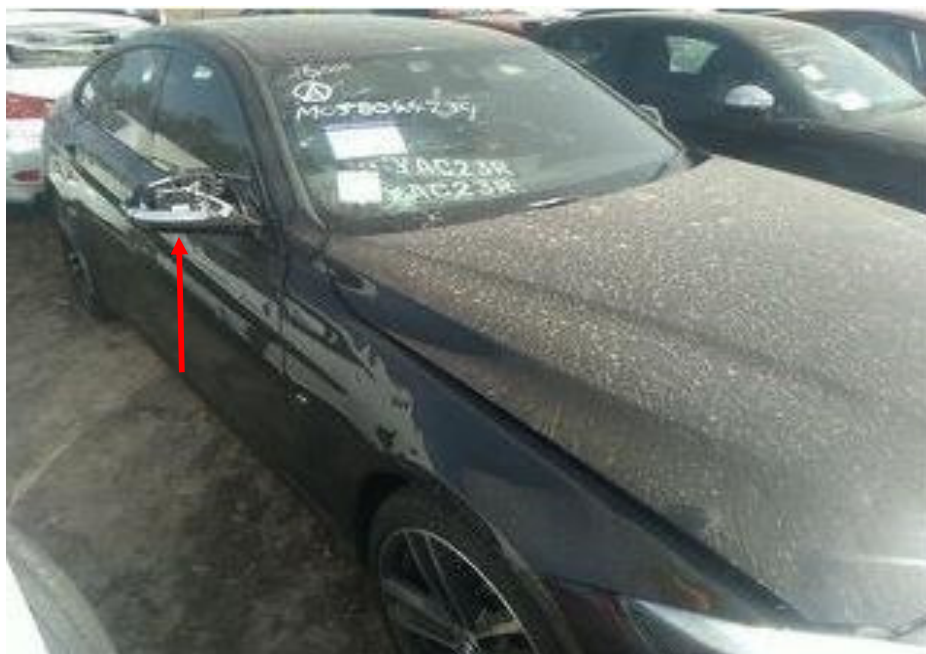
Photo 2 shows the front right body of the Motor Car prior to any repairs being carried out (photograph provided to me). The Motor Car was observed to have sustained damages of indentation nature to multiple exterior body parts like its front bonnet. As seen from the photographs provided, the indentation was relatively minor. The right side wing mirror (arrowed) was also observed to be broken.
