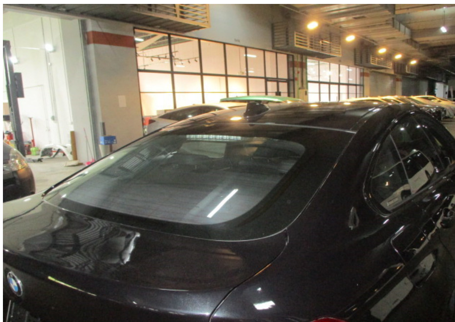
Photo 9 shows a general view of the rear body of the Motor Car at the time of my inspection. The Motor Car was observed to be in a relatively good general condition with no loose exterior fittings observed. The exterior body parts at the rear body of the Motor Car were visually examined and it was observed that the repair/restoration works carried out to the damaged area of the Motor Car (refer photograph 3 & 4 above) were reasonably adequate and in order.
