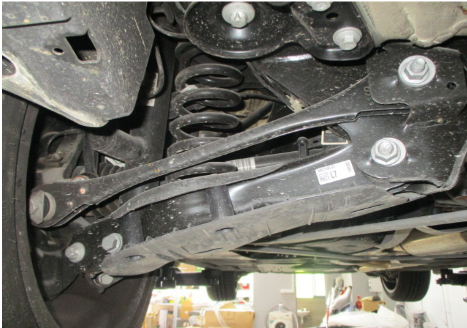
Photo 16 shows a general view of the control arms and linkages at the rear left wheel of the Motor Car. I did not observe any fluid leak and/or fluid stain on the underside of the Motor Car. All the Motor Car's undercarriage components were observed to be intact and secured in an appropriate manner.
