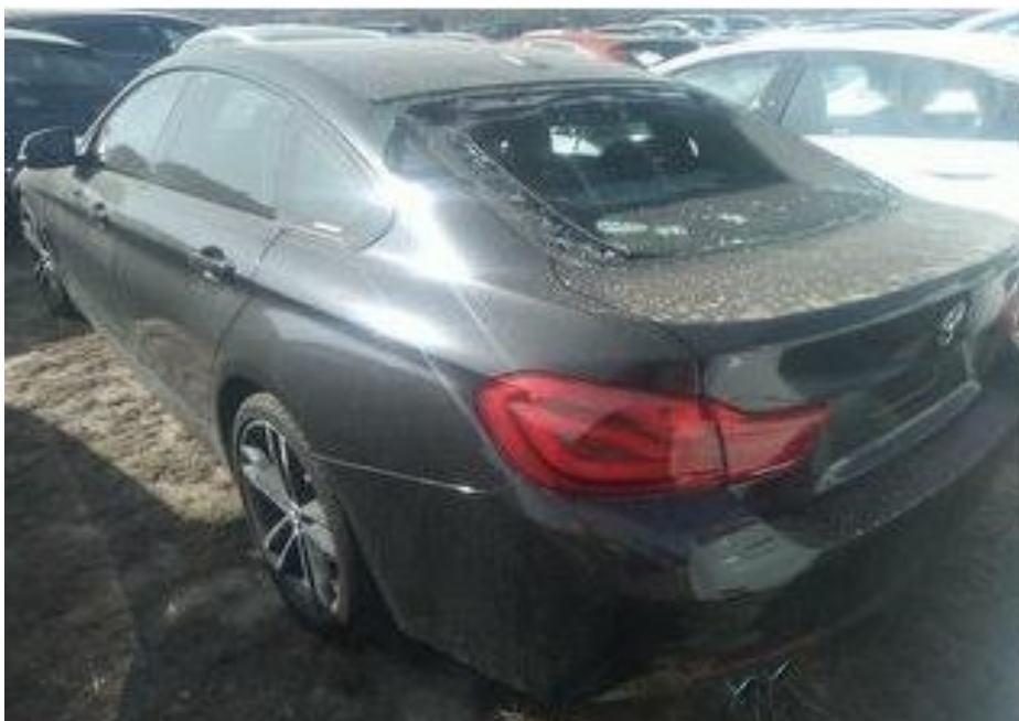
Photo 4 shows the rear left body of the Motor Car prior to any repairs being carried out (photograph provided to me). The Motor Car was observed to have sustained damages of indentation nature to multiple exterior body parts like its rear bootlid amongst others. As seen from the photographs provided, the indentation was relatively minor. The rear windscreen was also observed to be broken.
