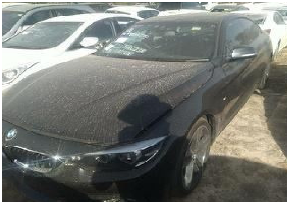
Photo 1 shows the front left body of the Motor Car prior to any repairs being carried out (photograph provided to me). The Motor Car was observed to have sustained damages of indentation nature to multiple exterior body parts like its front bonnet. As seen from the photographs provided, the indentation was relatively minor.
