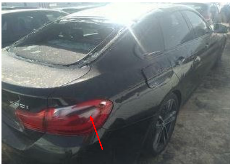
Photo 3 shows the rear right body of the Motor Car prior to any repairs being carried out (photograph provided to me). Relatively minor indentation damage was seen on the rear right fender, rear bootlid and rear roof panel amongst others. The rear right taillamp (arrowed) was also observed to be broken.
