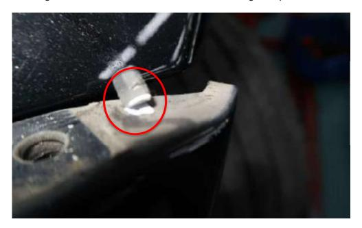
The photograph below shows the bumper and fender in perfect alignment before the car was stripped by the workshop indicating that the bumper mounting lug could not have been snapped off at this point.
