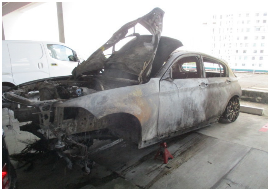
Photo 2 shows the general view of the left body of the Insured Vehicle at the time of our inspection. The Insured Vehicle was observed to have sustained extensive fire damage all around. Rust had accumulated all around the Insured Vehicle as a result of exposure to environmental condition for a period of time.
