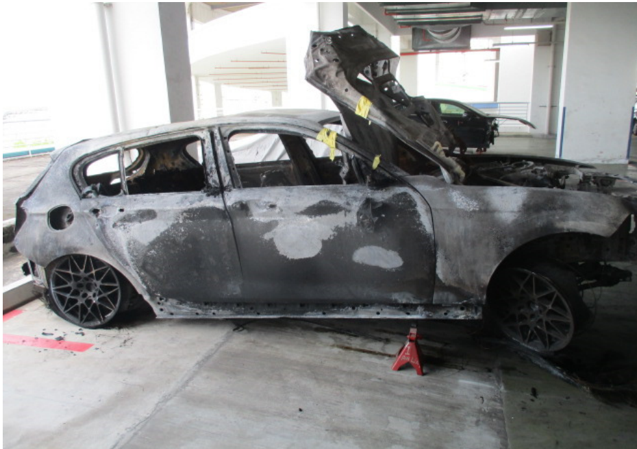
Photo 3 shows the general view of the right body of the Insured Vehicle at the time of our inspection. The Insured Vehicle was observed to have sustained extensive fire damage all around. Rust had accumulated all around the Insured Vehicle as a result of exposure to environmental condition for a period of time.
