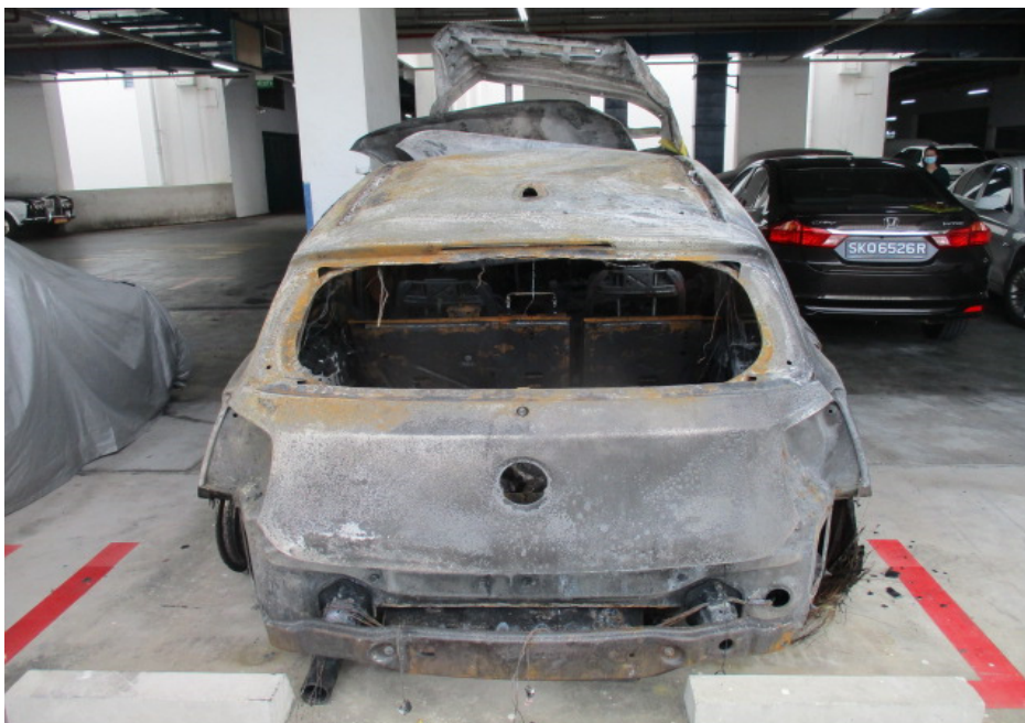
Photo 4 shows the general view of the rear portion of the Insured Vehicle at the time of our inspection. The Insured Vehicle was observed to have sustained extensive fire damage all around. Rust had accumulated all around the Insured Vehicle as a result of exposure to environmental condition for a period of time.
