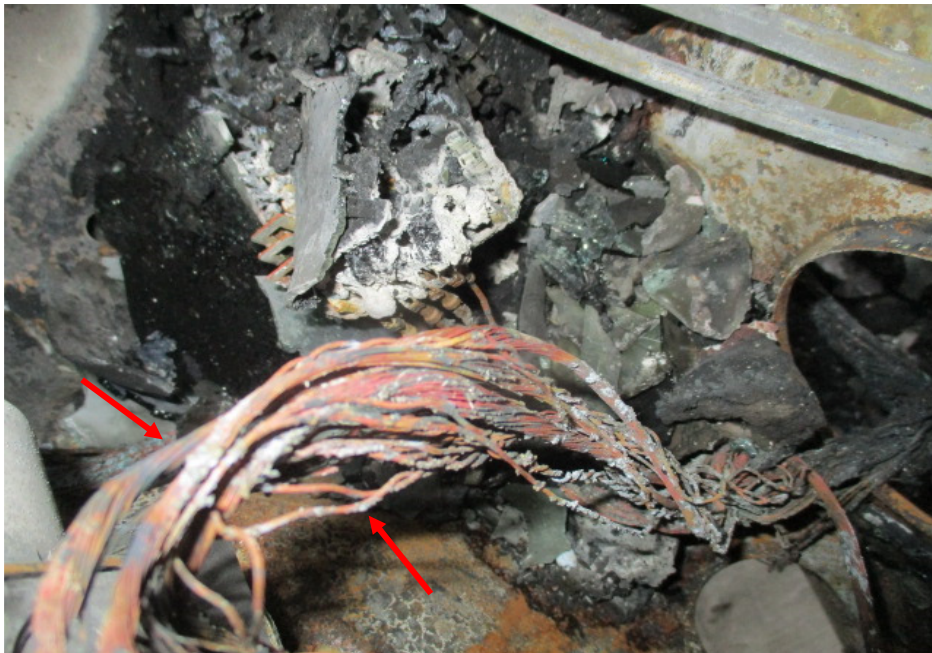
Photo 11 shows a close up view of the greenish residue on the wirings at the rear left portion of the engine compartment (arrowed). The presence of such greenish residue suggests occurrence of an electrical short circuit.
