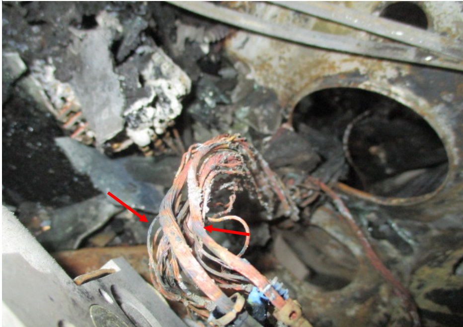
Photo 10 shows a close up view of the greenish residue on the wirings at the rear left portion of the engine compartment (arrowed). The presence of such greenish residue suggests occurrence of an electrical short circuit.
