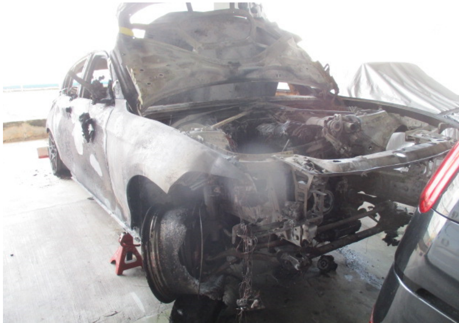
Photo 1 shows the general view of the front left portion of the Insured Vehicle at the time of our inspection. The Insured Vehicle was observed to have sustained extensive fire damage all around. Its engine compartment and interior compartment were completely burnt. Rust had accumulated all over the rear and centre portion of the Insured Vehicle as a result of exposure to environmental condition for a period of time.
