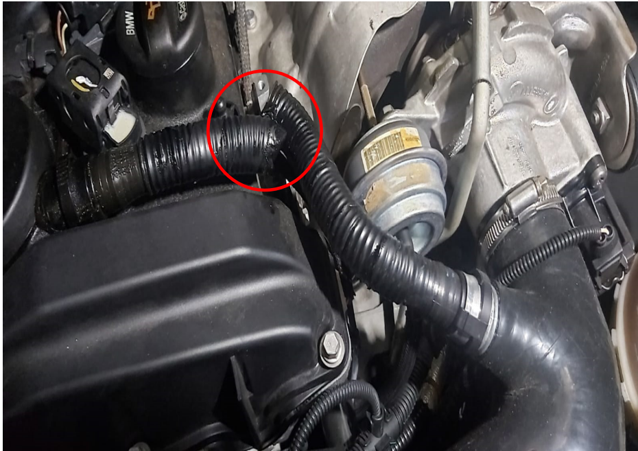
Photo 12 shows the broken breather hose of the Insured Vehicle (circled) which was later replaced by the broker as mentioned by Mr Sufiyan.
