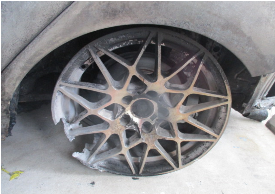
Photo 7 shows the non-standard rim (which had sustained minor fire damage) found to be fitted on the Insured Vehicle at the time of our inspection. The 18-inch alloy rims fitted on the Insured Vehicle were not the standard type for the Insured Vehicle.
