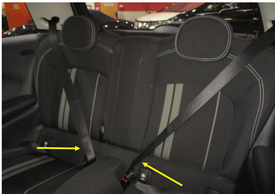
Photo 9 shows the rear seats of the Motor Car. All the seats of the Motor Car were secured via seat rails to the floorboard. They were also fitted with a retractable seat belt reel and a pre-tensioner. The seat belts (arrowed) were tested and were able to be fastened into the respective pre-tensions that were fitted on the side of each individual seat.
