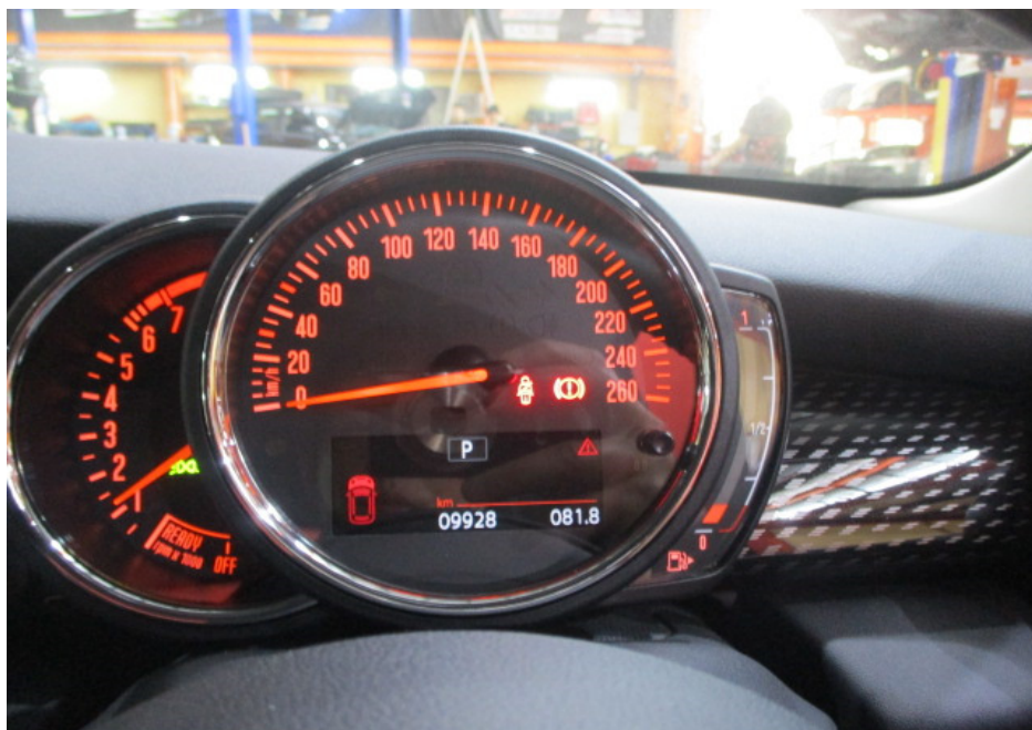
Photo 11 shows the respective warning lights no longer illuminated, indicating that there is no fault detected to the ABS, SRS, PAS, TPM and DSC systems of the Motor Car during the self-test. These electronic systems were hence in working condition at the time of my inspection.
