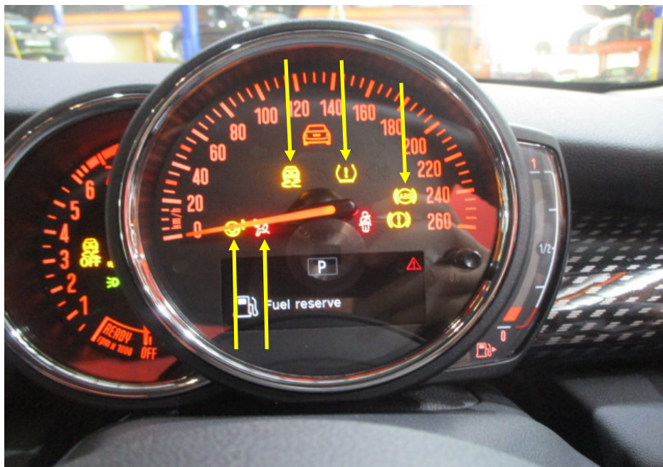
Photo 10 shows the warning lights for the various electronic safety features appearing on the instrument panel of the Motor Car during its self-test when the engine is cranked, in particular the ABS, SRS, PAS, TPM and DSC lights (arrowed).
