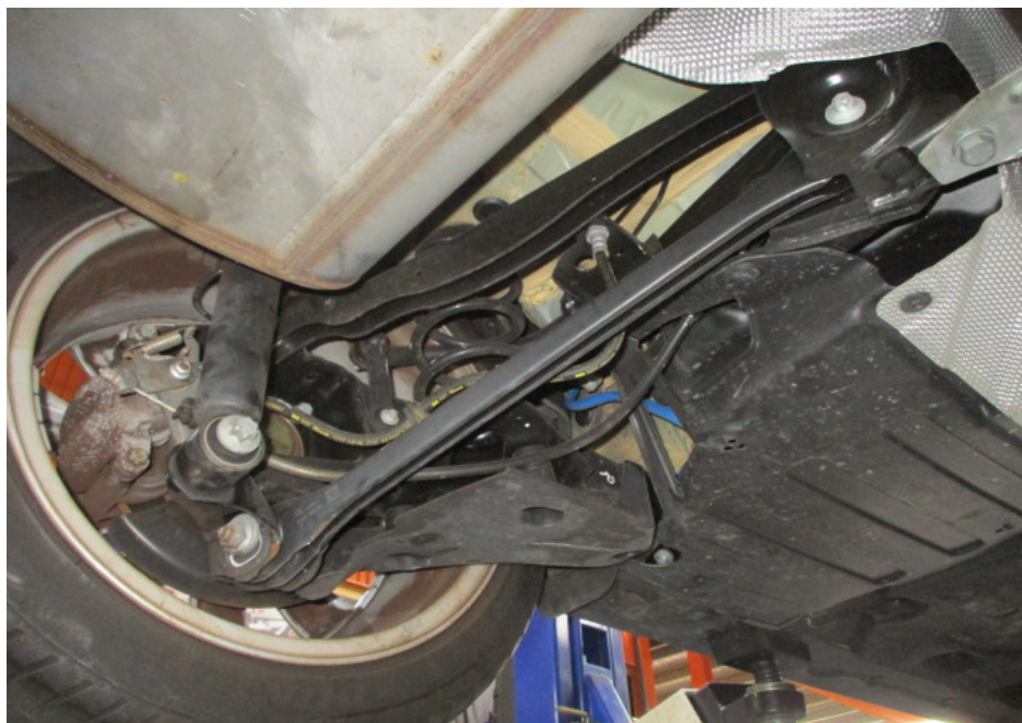
Photo 13 shows a general view of the control arms and linkages at the rear left wheel of the Motor Car. I did not observe any fluid leak and/or fluid stain on the underside of the Motor Car. All of the Motor Car's undercarriage components were observed to be intact and secured in an appropriate manner.
