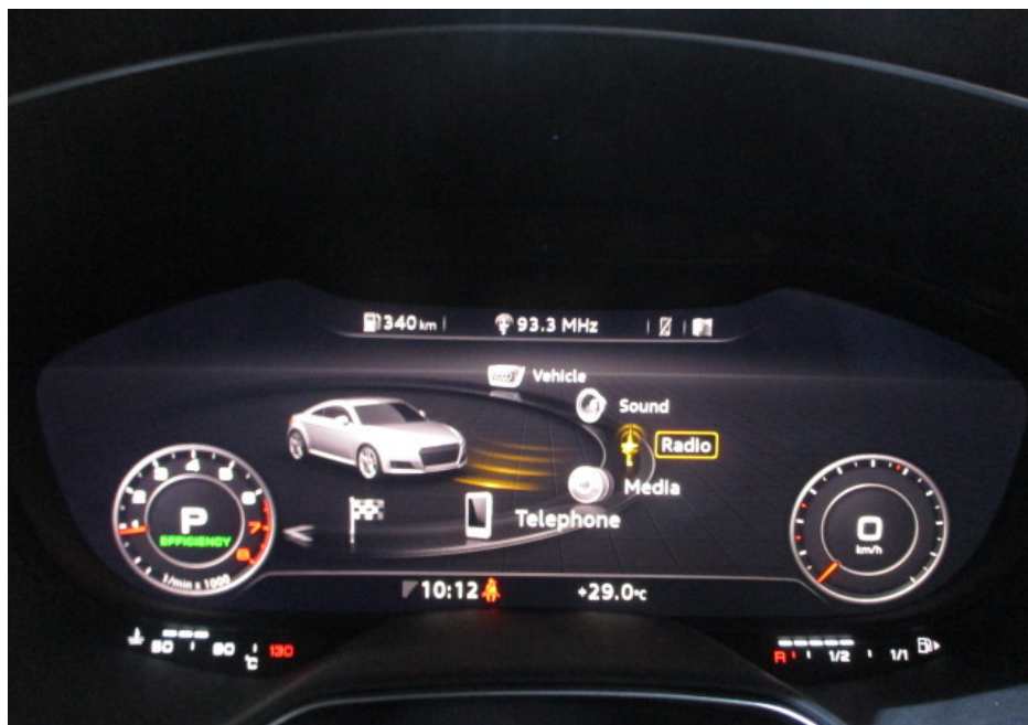
Photo 14 shows the respective warning lights no longer illuminated, indicating that there is no fault detected to the ABS, SRS, EPS, TPM and ESC systems of the Motor Car during the self-test. These electronic systems were hence in working condition at the time of my inspection.
