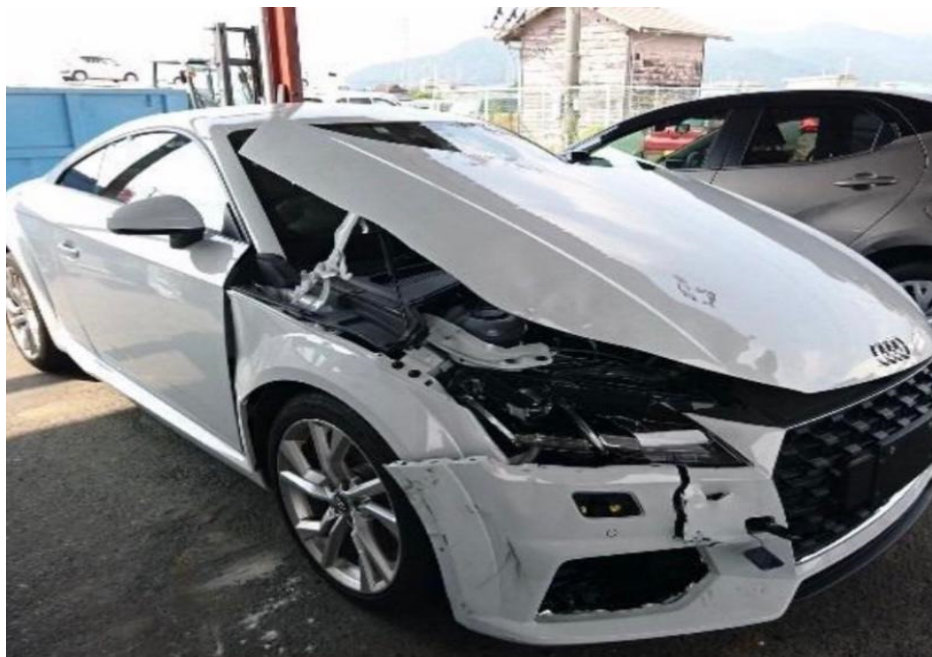
Photo 1 shows the front right body of the Motor Car (photograph provided to me). The Motor Car was observed to have sustained damage at its frontal portion. The front bumper, front right headlamp, front grille, front bumper right lower grille and front bonnet were amongst the body parts that were observed to have been damaged.
