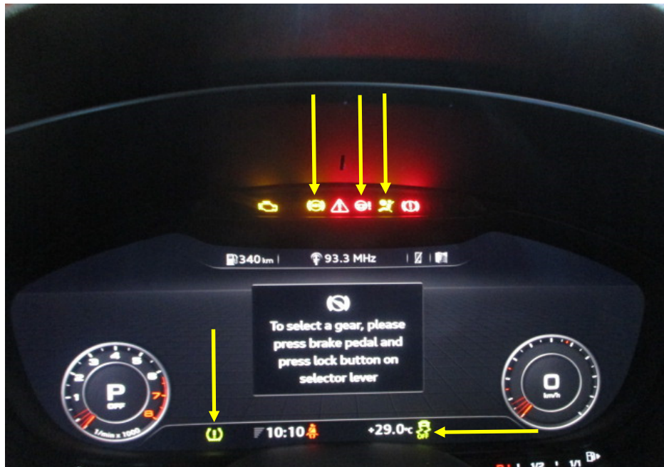
Photo 13 shows the warning lights for the various electronic safety features appearing on the instrument panel of the Motor Car during its self-test when the engine is cranked, in particular the ABS, SRS, EPS, TPM and ESC lights (arrowed).
