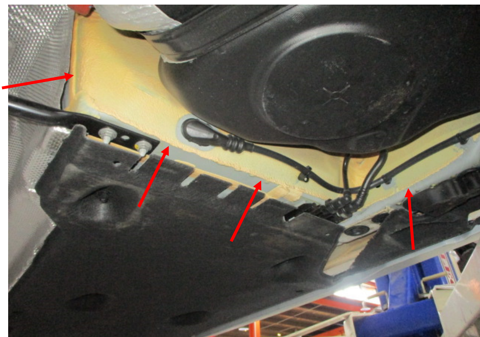
Photo 20 shows the floorboard at the underside right centre of the Motor Car. The original factory sealant (arrowed) at the joints along the floorboard (non-detachable body panel) was untouched, indicating no work was done on the floorboard of the Motor Car. In general, I had found all the non-detachable body panels of the Motor Car to be originally fitted at the time of my inspection.
