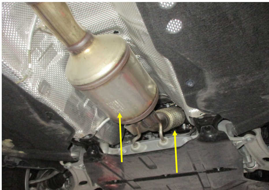
Photo 19 shows the Motor Car's catalytic converters (arrowed). My examination of the Motor Car's exhaust system revealed no sign(s) or indication(s) of any cut or weld marks along its exhaust pipes and on its rear muffler.
