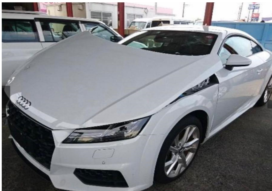
Photo 2 shows the front left body of the Motor Car (photograph provided to me). The Motor Car was observed to have sustained damage at its frontal portion. The front bonnet and front bonnet hinges were amongst the body parts that were observed to have been damaged.
