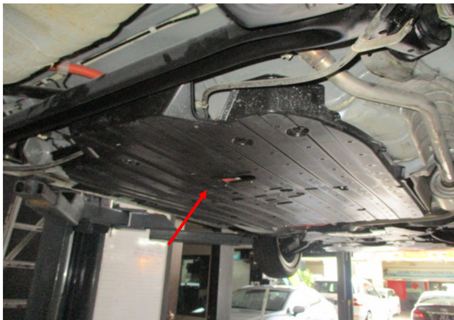
Photo 22 shows the underside of the Motor Car. I had observed that the electric cables connecting the electric motor within the engine compartment to the electric battery at the rear of the Motor Car were securely fitted into the respective connectors and protected by a dust cover (arrowed).
