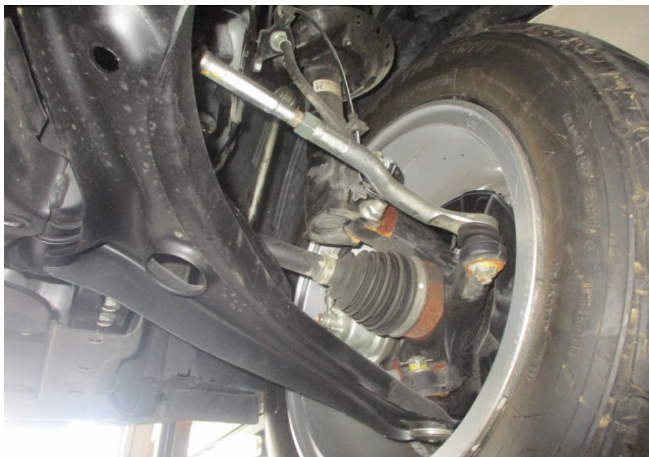
Photo 18 shows the various undercarriage components at the front right wheel of the Motor Car. The mechanical components, control arms and linkages were all found to be intact and secured in an appropriate manner.
