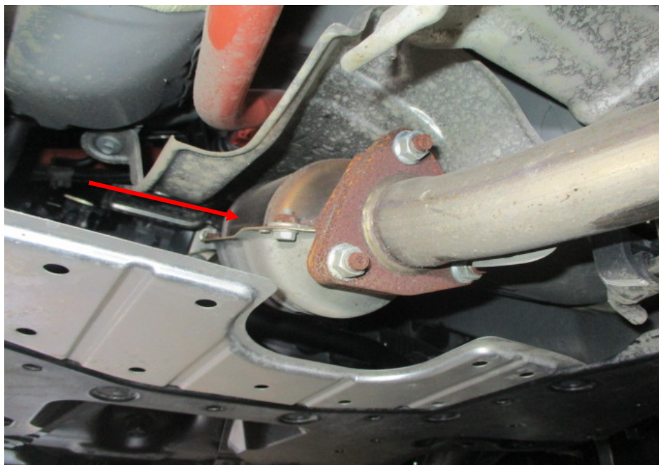
Photo 20 shows the Motor Car's catalytic convertor (arrowed). My examination of the Motor Car's exhaust system revealed no sign(s) or indication(s) of any cut or weld marks along its exhaust pipes and on its rear muffler.
