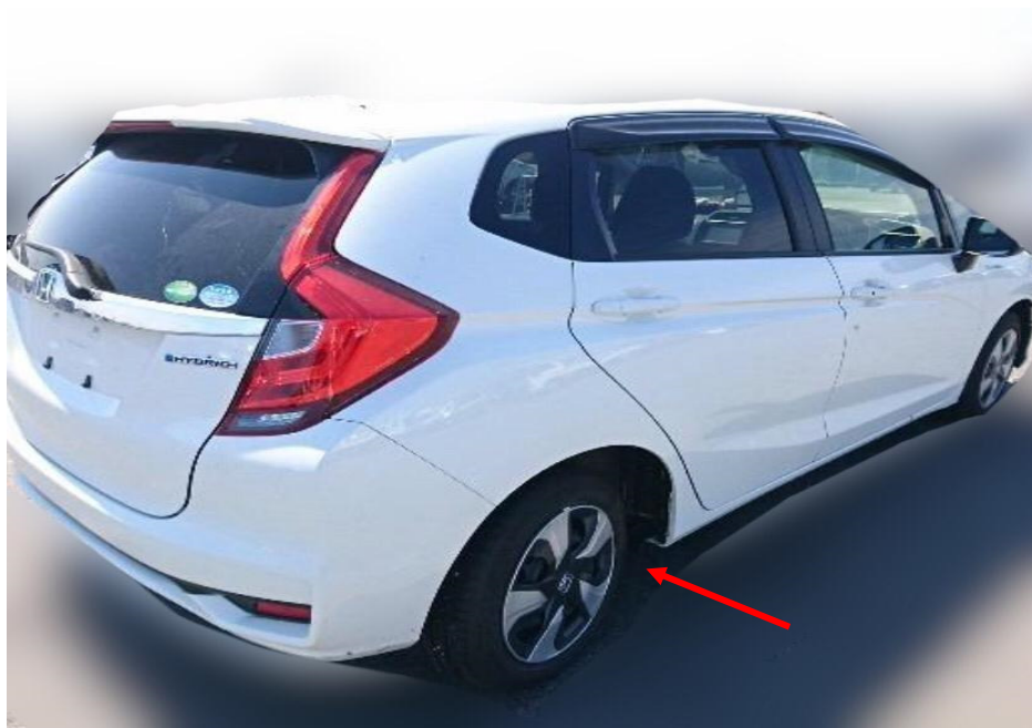
Photo 3 shows the rear right body of the Motor Car prior to any repairs being carried out (photograph provided to me). The right rear wheel was orientated inwards (arrowed), which indicates damage to the rear undercarriage parts of the Motor Car.
