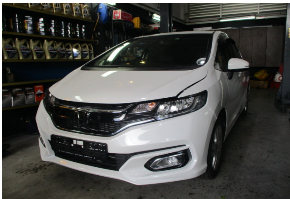
Photo 5 shows a general view of the front left body of the Motor Car at the time of my inspection. The Motor Car was observed to be in a relatively good general condition with no loose exterior fittings observed. The body parts at the front left portion of the Motor Car were visually examined and it was observed that the repair/restoration works carried out to the damaged area of the Motor Car (refer to photograph 1) were reasonably adequate and in order.
