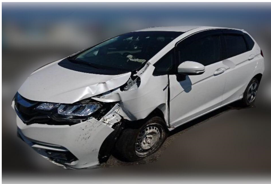
Photo 1 shows the front left body of the Motor Car prior to any repairs being carried out (photograph provided to me). The Motor Car was observed to have sustained damages at its front left portion. Body parts damaged had include its front bumper, front left headlamp, front bonnet and front left fender amongst others. The front left undercarriage parts were also damaged as seen from the orientation of the front left wheel, which was pushed backwards.
