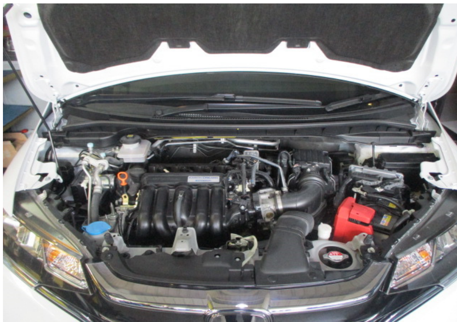
Photo 12 shows a general view of the engine compartment of the Motor Car at the time of my inspection. The various parts and components inside the engine compartment were all observed to be intact and properly fitted. There was also no sign(s) or indication(s) of fluid leak and/or fluid stain found inside the engine compartment.
