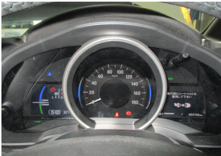
Photo 15 shows the respective warning lights no longer illuminated, indicating that there is no fault detected to the ABS, SRS, EPS, SC, LDW and CMBS systems of the Motor Car during the self-test. These electronic systems were hence in working condition at the time of my inspection.
