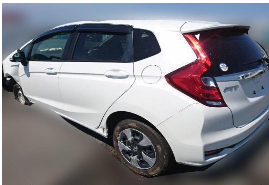
Photo 2 shows the rear left body of the Motor Car prior to any repairs being carried out (photograph provided to me). The Motor Car was observed to have also sustained damages at its rear left portion. Body parts damaged had include its rear left fender, rear left wheel and rear left door amongst others. The rear undercarriage parts were also damaged as seen from the orientation of the rear right wheel (refer to photograph 3 below).
