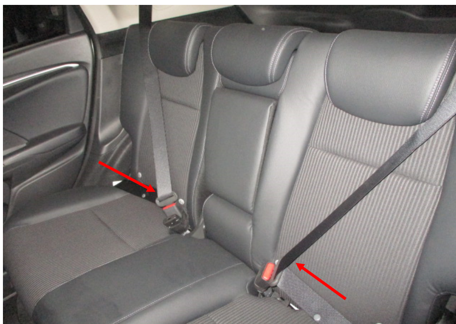
Photo 13 shows the rear seats of the Motor Car. All the seats of the Motor Car were secured via seat rails to the floorboard. They were also fitted with a retractable seat belt reel and a pre-tensioner. The seat belts (arrowed) of the Motor Car were tested and were able to be fastened into the respective pre-tensions that were fitted on the side of each individual seat.
