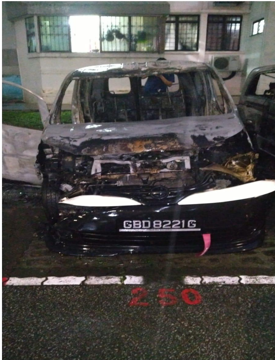
Photo 22 shows the exterior of the Insured Vehicle after the fire was put out. The high heat intensity burn marks (whitish burn marks) and rust that had development found on the exterior surface of the Insured Vehicle. In general, the information that could be gathered from this photograph had corresponded to the events that were related to us by Mr Irman, location when the fire broke out.
