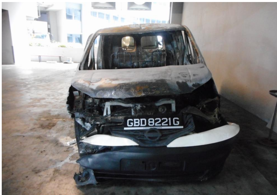
Photo 1 shows the general view of the front portion of the Insured Vehicle at the time of our inspection. The Insured Vehicle was observed to have sustained extensive fire damage all around. Its engine compartment and interior compartment were completely burnt. Rust had accumulated all over the front and centre portion of the Insured Vehicle as a result of exposure to environmental condition for a period of time.
