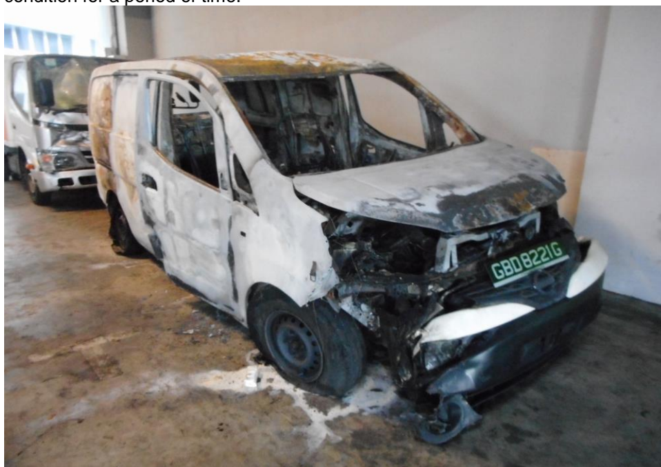
Photo 2 shows the general view of the right body of the Insured Vehicle at the time of our inspection. The Insured Vehicle was observed to have sustained extensive fire damage all around. Rust had accumulated all over the front and interior compartment of the Insured Vehicle as a result of exposure to environmental condition for a period of time.
