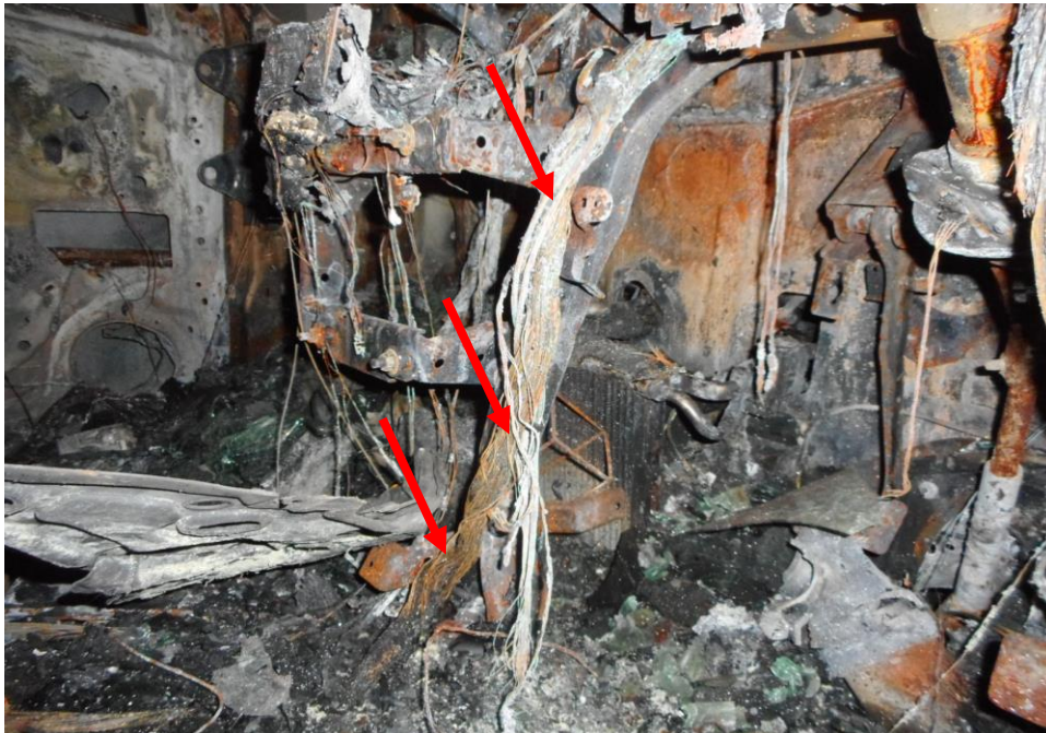
Photo 15 shows the close up view of the interior compartment of the Insured Vehicle at the time of our inspection. We had also found traces of greenish residue on the wirings harnesses and the broken copper wirings this is due to the intense heat generate from the short circuit that had likely been where the fire had started from (arrowed) leading from the battery to the electrical components in the cabin of the Insured Vehicle.
