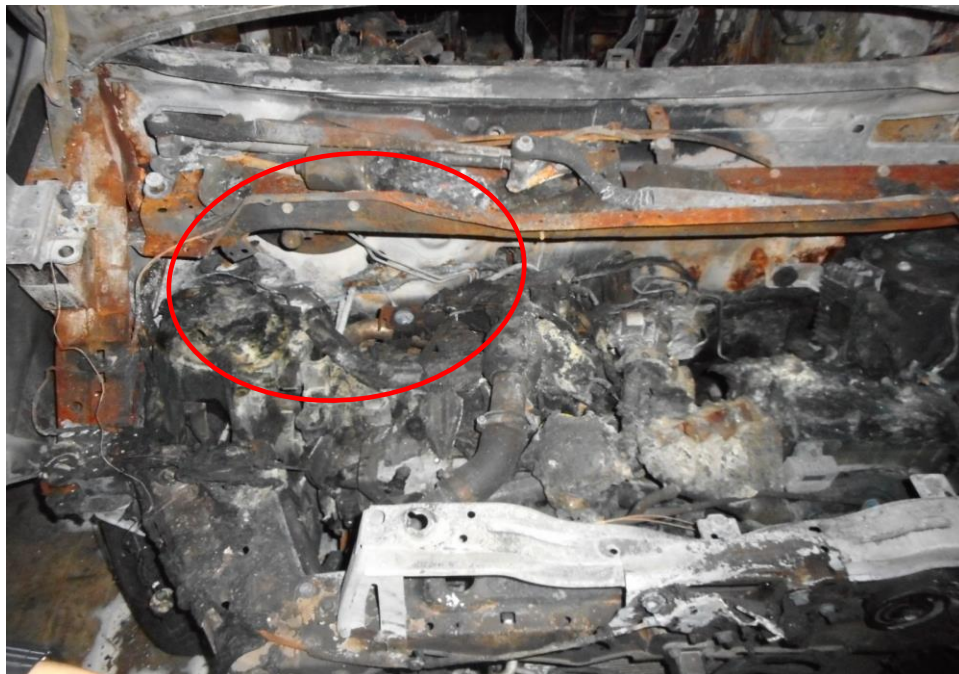
Photo 11 shows the general view of the engine compartment of the Insured Vehicle at the time of our inspection. We had observed that the front driver's portion (circled) of the engine compartment had sustained a stronger high heat intensity burn marks as compared to the surrounding areas of the engine compartment
