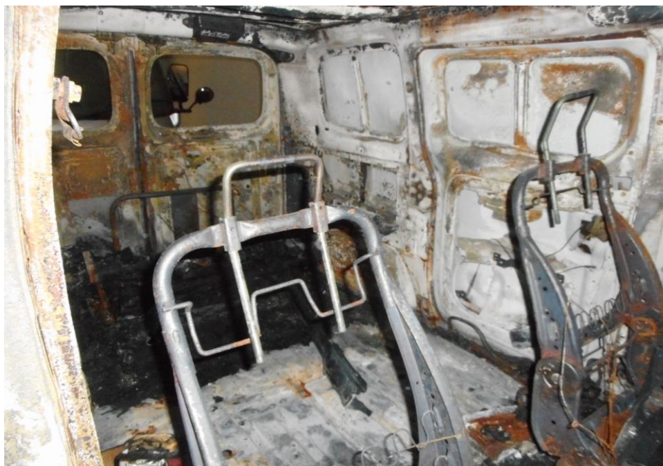
Photo 10 shows the interior of the Insured Vehicle at the time of our inspection. The High heat intensity burn marks (whitish burn marks) and rust that had developed on the interior surfaces of the Insured Vehicle due to the fire that had spread all around..
