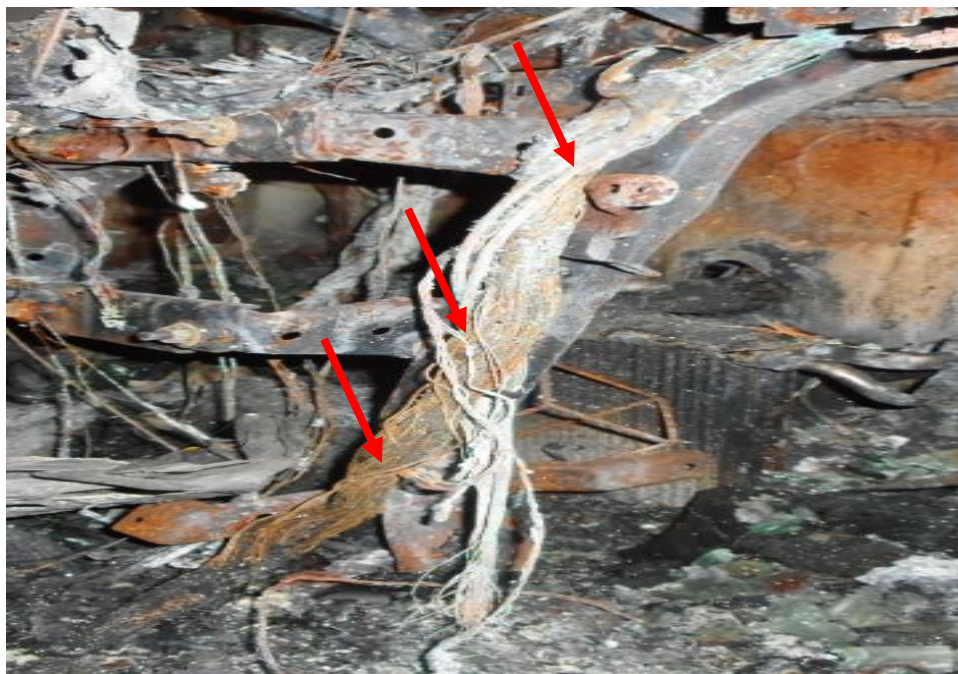
Photo 16 shows the close up view of the interior compartment of the Insured Vehicle at the time of our inspection. We had also found traces of greenish residue on the wirings harnesses and the broken copper wirings this is due to the intense heat generated from the short circuit and this had likely been where the fire had started from and spread to the whole vehicle (arrowed)
