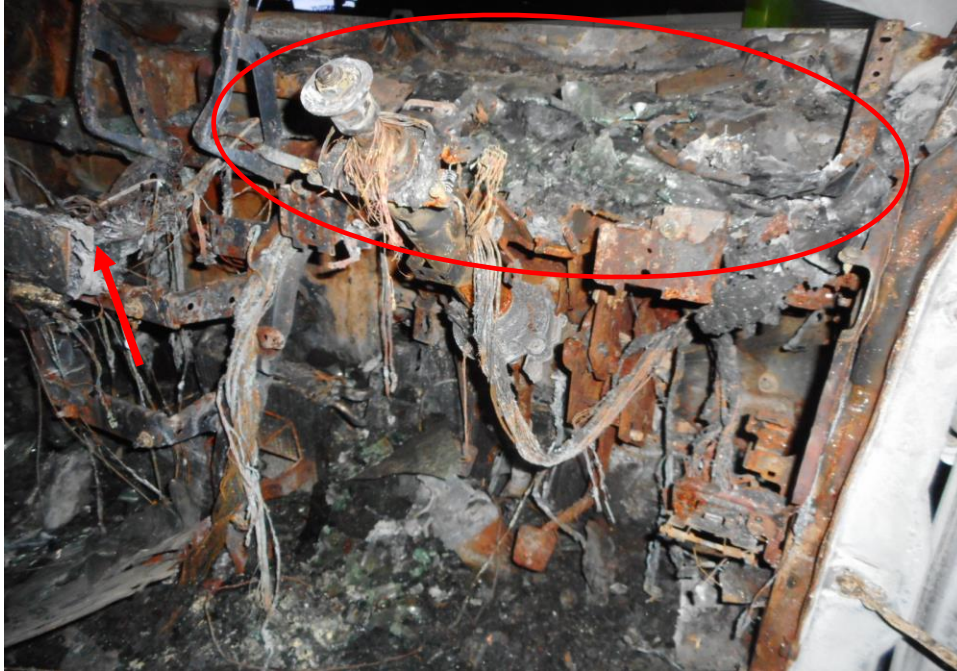
Photo 14 shows the general view of the interior compartment of the Insured Vehicle at the time of our inspection. The fire damage to the Insured Vehicle has affected its engine and interior compartment. Its interior dashboard (circled), radio head unit (arrowed), various original wiring harnesses was amongst the parts in the compartment that were found to have been affected as a result of the fire.
