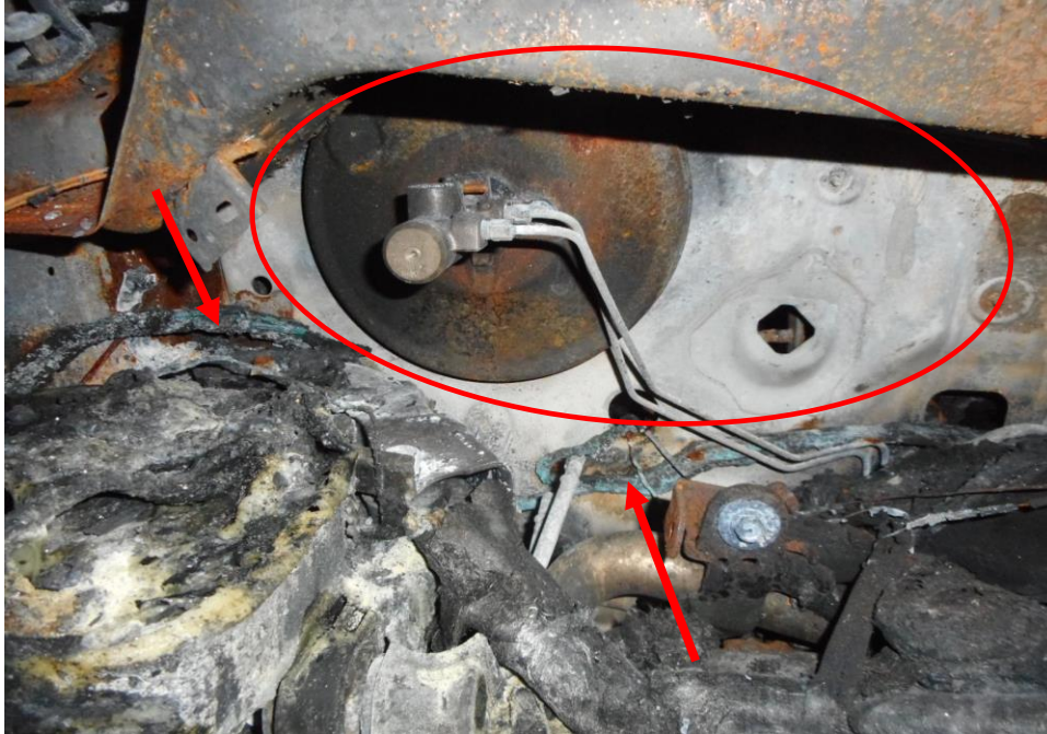
Photo 12 shows the close up view of the engine compartment of the Insured Vehicle at the time of our inspection. We had observed that the front driver's portion of the engine compartment had sustained a stronger high heat intensity burn marks as compared to the surrounding areas of the engine compartment and we had also found traces of greenish residue on the wirings harnesses (arrowed) leading from the battery to the electrical components in the cabin of the Insured Vehicle.
