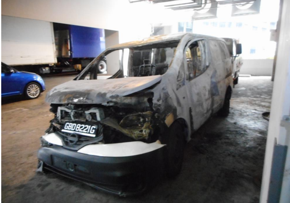
Photo 3 shows the general view of the left body of the Insured Vehicle at the time of our inspection. The Insured Vehicle was observed to have sustained extensive fire damage all around. Rust had accumulated all over the front and centre portion of the Insured Vehicle as a result of exposure to environmental condition for a period of time.
