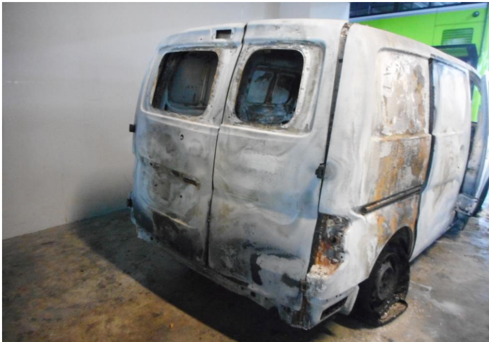
Photo 4 shows the general view of the rear portion of the Insured Vehicle. The Insured Vehicle was observed to have sustained extensive fire damage all around. Rust had accumulated all over the front and centre portion of the Insured Vehicle as a result of exposure to environmental condition for a period of time.
