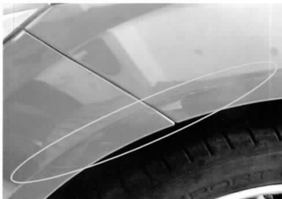
Photo 10 shows a close up view of the paint graze marks on the top portion of the Mercedes's left front tyre fender (circled).
