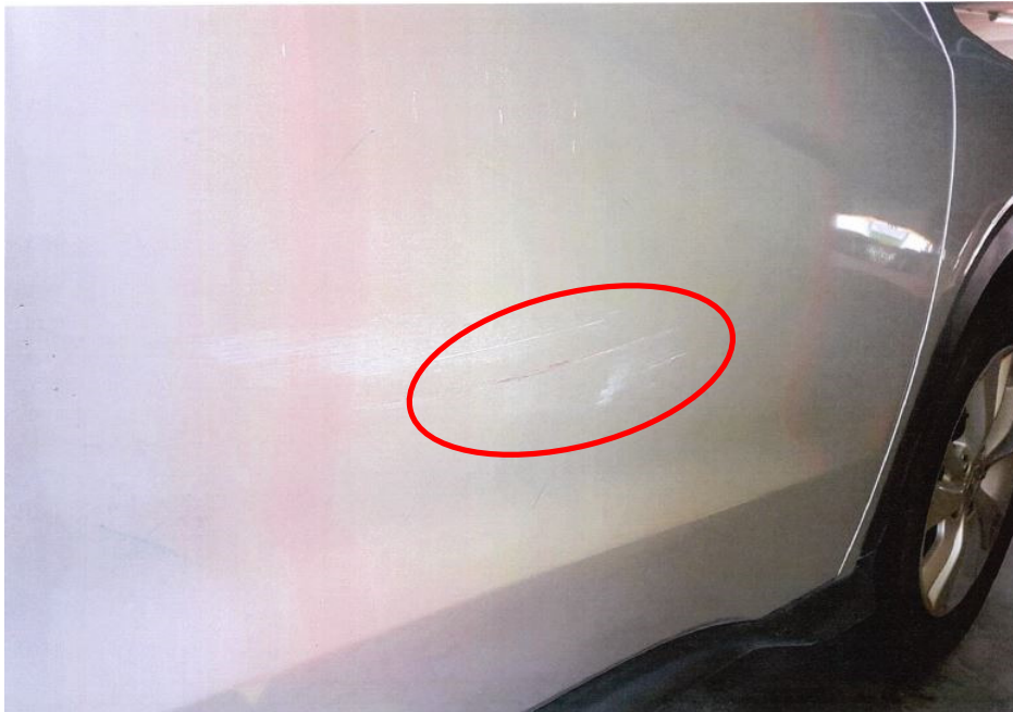
Photo 16 shows upon review of the available photographs taken at the workshop depicting the damages sustained to the right portion of Honda, we observed the same reddish paint transfer marks and paint graze marks on the driver door of the Honda as per the Pre- Repair Survey photographs (circled).
