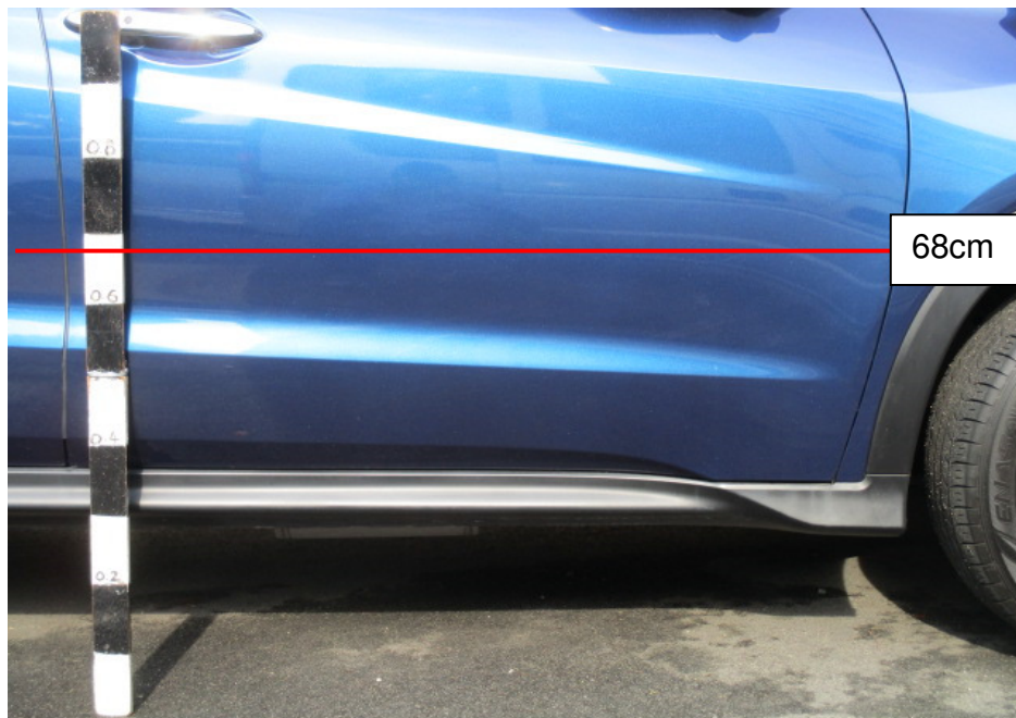
Photo 19 shows the height measurement being conducted on the right passenger door of the Honda (using a similar make and model). The height above ground level of the area where the reddish paint transfer marks were found was measured to be approximately 68cm.
