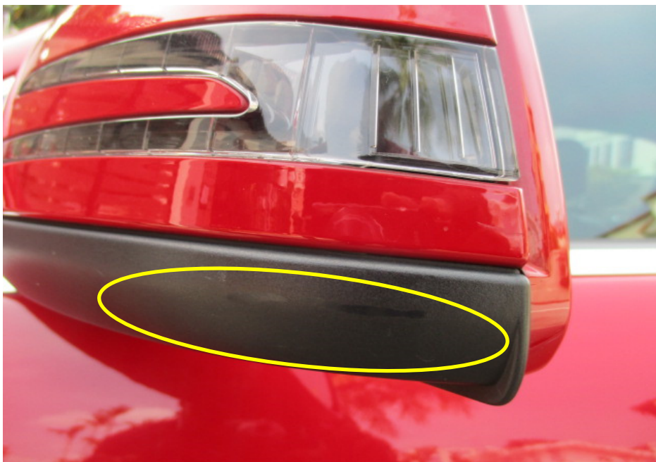
Photo 12 shows a close up view of the left side mirror of the Mercedes at the time of our inspection. We noticed scuff marks on the lower portion of the left side mirror (circled).
