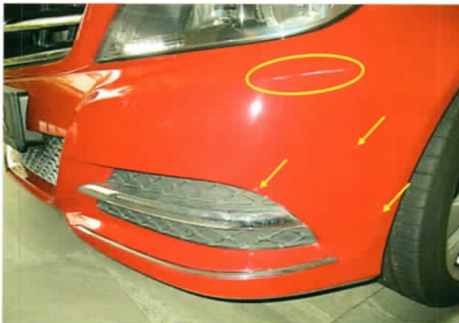
Photo 8 shows the paint graze marks (circled) and paint scuff marks (arrowed) found on the front left portion of the Mercedes.
