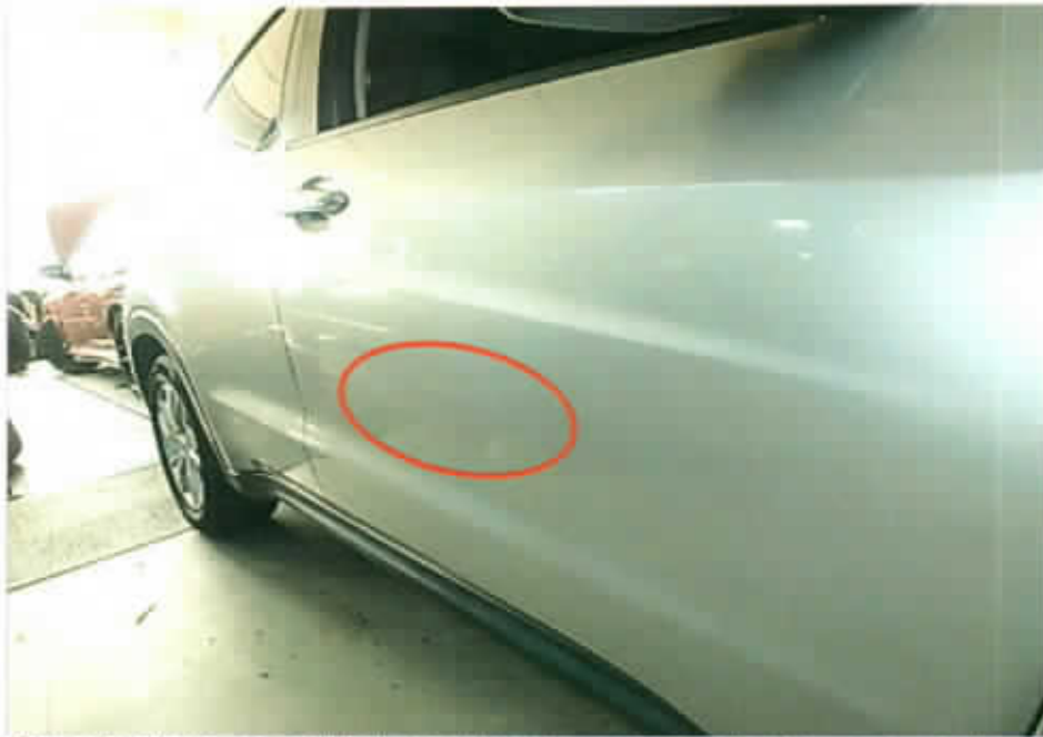
Photo 2 shows the reddish paint transfer marks and paint graze marks we observed on the driver door of the Honda (circled).
