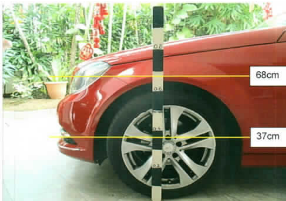
Photo 21 shows the height measurement being conducted on the left front portion of the Mercedes. The height range of the paint graze marks found on the left front portion of the Mercedes is between 37cm to 68cm above ground level.
