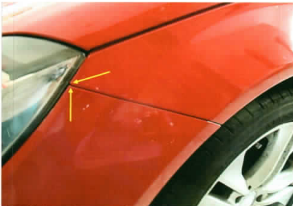
Photo 14 shows a close up view of the left corner edge of the front bumper of the Mercedes. We observed that there was no misalignment at the corner edges (arrowed).
