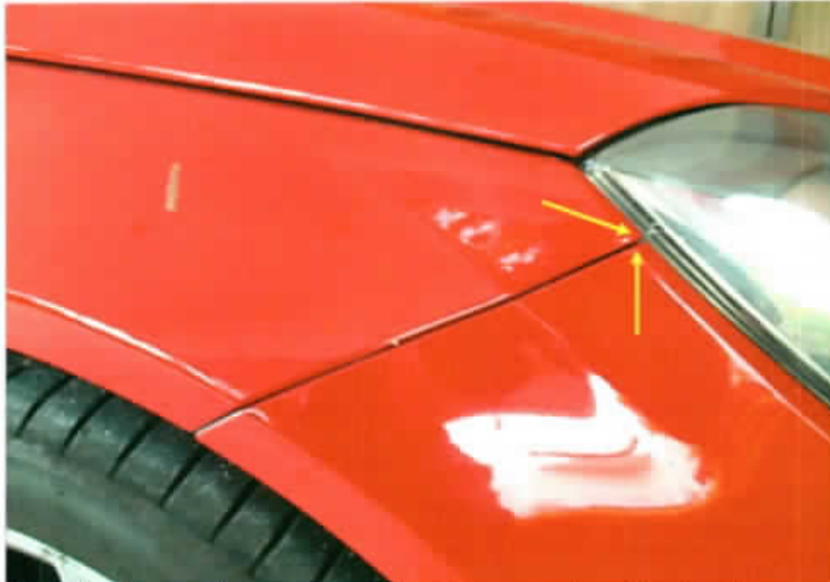
Photo 13 shows a close up view of the right corner edge of the front bumper of the Mercedes. We observed that there was no misalignment at the corner edges (arrowed).
