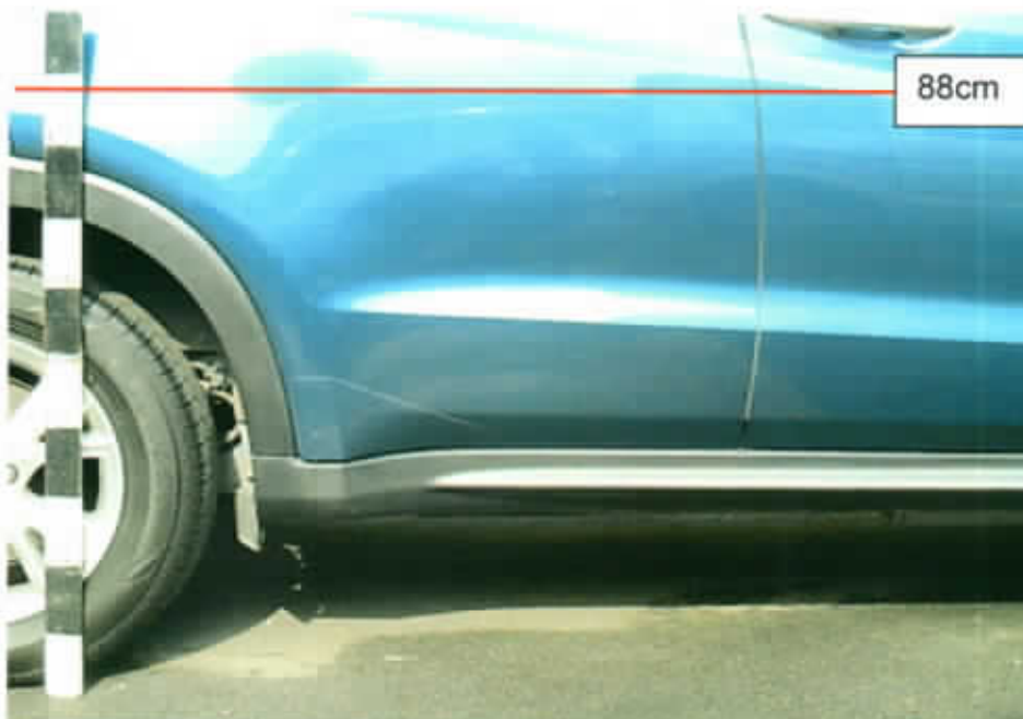
Photo 20 shows the height measurement being conducted on the right passenger door of the Honda. The height above ground level of the area where the black marks were found was measured to be approximately 88cm.
