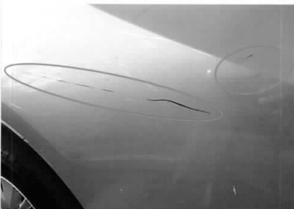
Photo 5 shows a closer view the black marks observed on the right passenger door of the Honda (circled).
