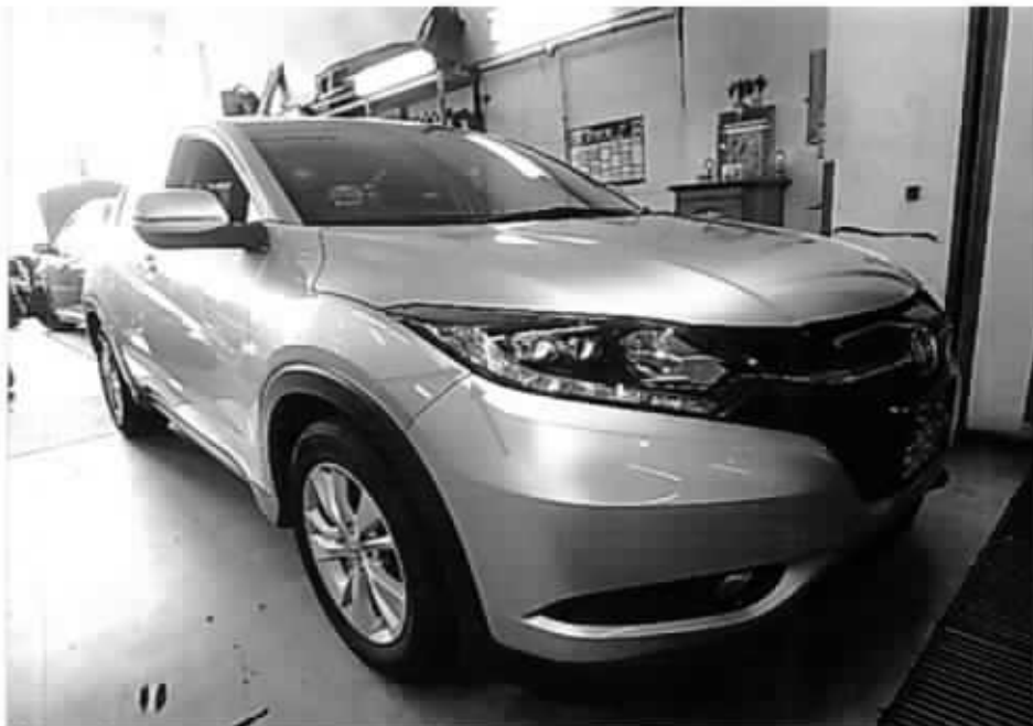
Photo 1 shows a general view of the right front portion of the Honda at the time of the Pre- Repair Survey conducted by LKK Auto Consultants Pte. Ltd. about 1 day after the accident. We noted that the front bumper was not misaligned at its right corner edge (arrowed).
