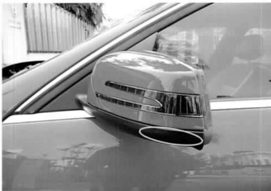
Photo 11 shows a view of the left side mirror of the Mercedes at the time of our inspection. We noticed scuff marks on the lower portion of the left side mirror (circled).
