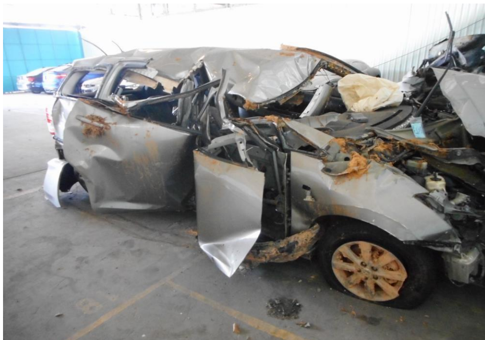
Photo 8 shows a general view of the Motor Car's right body at the time of my inspection. The Motor Car was observed to sustained damage at its right portion. Its right body panels were amongst the body parts that were damaged as a result of the accident.
