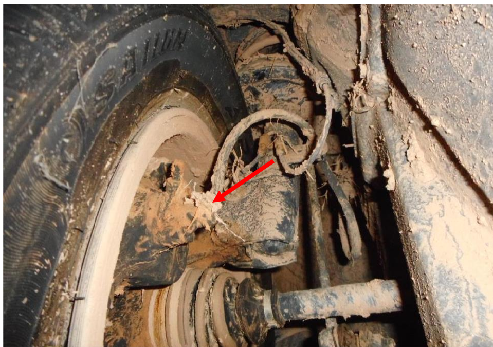
Photo 20 shows the brake hose/pipe (arrowed) at the front right wheel of the Motor Car. I did not observe any leakage of brake fluid at the time of my inspection of the Motor Car. The undercarriage components of the Motor Car were also all found to be intact and without any visible damage. The undercarriage components were cover in mud as due to the result of the accident.
