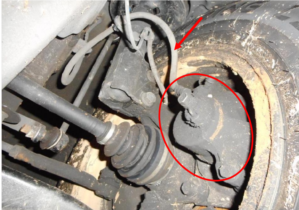
Photo 21 shows the brake hose/pipe (arrowed) at the front left wheel of the Motor Car. No leakage of brake fluid was observed. Visual examination of the various components of the braking system like the brake caliper (circled) had revealed all to be intact and without visible damage.
