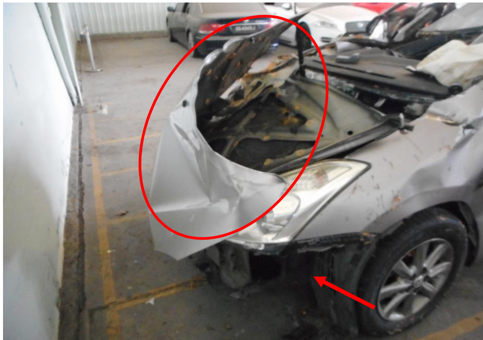
Photo 6 shows the close up view of the Motor Car's front body at the time of my inspection. The Motor Car was observed to have sustained damage at its front portion. Its front bonnet (circled) and front bumper (arrowed) were amongst the body parts that were damaged as a result of the accident.
