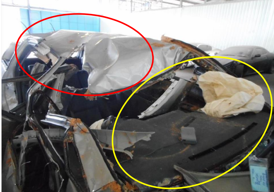
Photo 5 shows the close up view of the Motor Car's front body at the time of my inspection. The Motor Car was observed to have sustained damage at its front and roof portion. Its front windscreen (yellow circle) and roof (red circle) were amongst the body parts that were damaged as a result of the accident.
