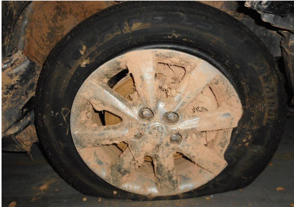
Photo 11 shows the condition of the front right tyre of the Motor Car, which was observed to slip off the rim as a result of the accident. The remaining tread depth of approximately 7.1mm. The tyre was observed to be deflated with no tear, cut or burst mark(s).
