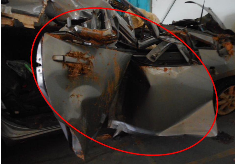
Photo 9 shows a close up view of the Motor Car's right body at the time of my inspection. The Motor Car was observed to sustained damage at its right portion. Its right body panels (circled) were amongst the body parts that were damaged as a result of the accident.
