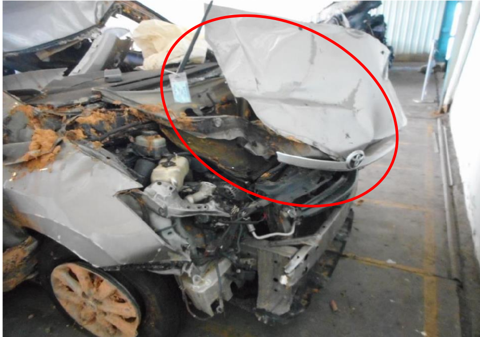
Photo 16 shows a close up view of the damaged front bonnet lock mechanism and the structure of the engine compartment of the Motor Car at the time of my inspection resulting it unable to open a result of the accident (circled) (Unable to open)
