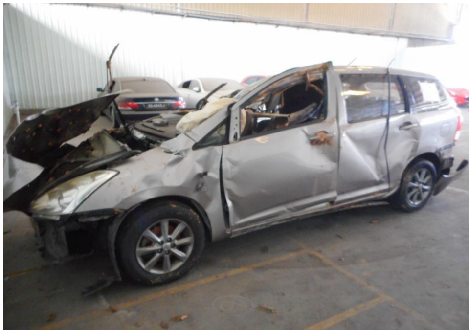
Photo 10 shows a general view of the Motor Car's left body at the time of my inspection. The Motor Car was observed to sustained damage at its left portion. Its left body panels were amongst the body parts that were damaged as a result of the accident.
