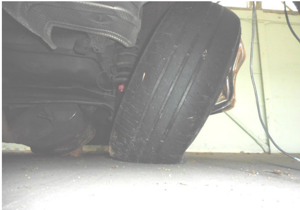
Photo 12 shows the condition of the rear right tyre of the Motor Car, which was observed to be in serviceable condition with remaining tread depth of approximately 4.6mm. The tyre, which was wrapped around alloy wheel rim, was also observed to be sufficiently inflated for vehicular operation.
