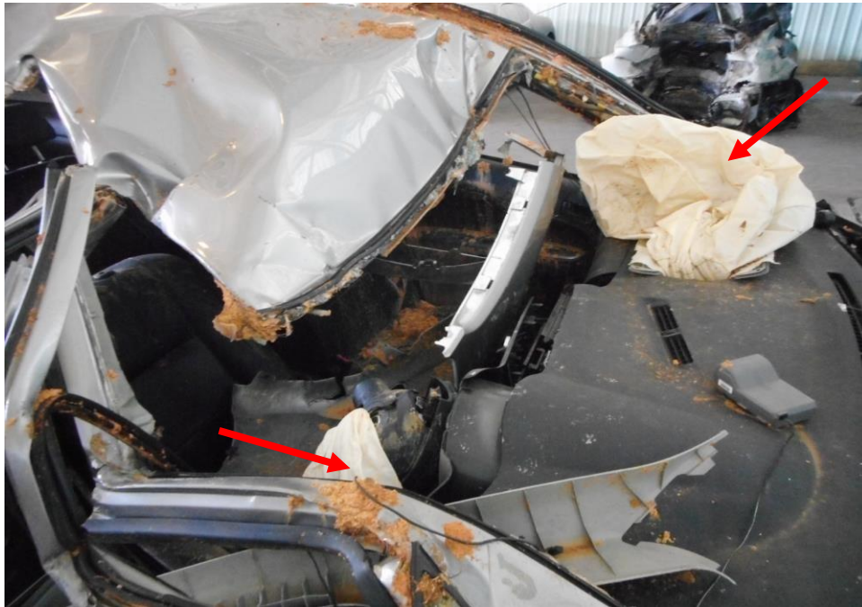
Photo 15 shows the deployment of the Supplemental Restraint System (SRS) airbags (arrowed) in the Motor Car as a result of the accident.
