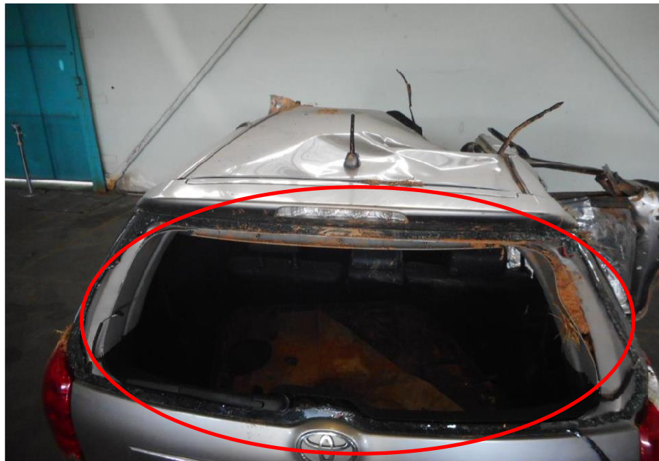
Photo 2 shows the close up view of the Motor Car's rear portion at the time of my inspection. The Motor Car was observed to sustained damage at its rear portion. Its rear windscreen (circled) were amongst the body parts that were damaged as a result of the accident.
