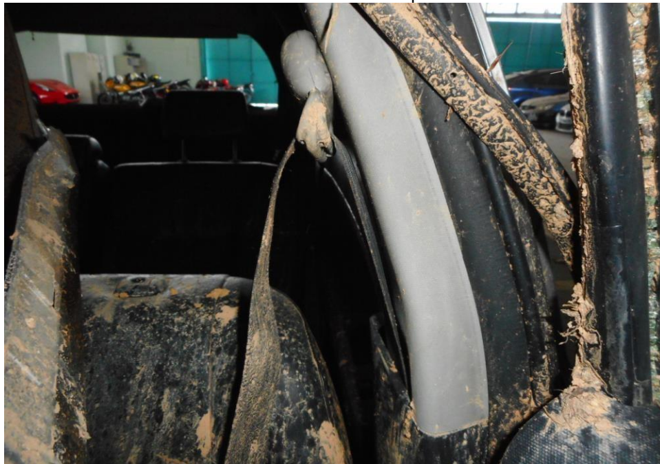
Photo 25 shows that that the seat belt on the left seat was not worn at the material time of accident as the safety pre-tensioners was activated at the moment of impact and caused the seat belt to be locked into the last position.
