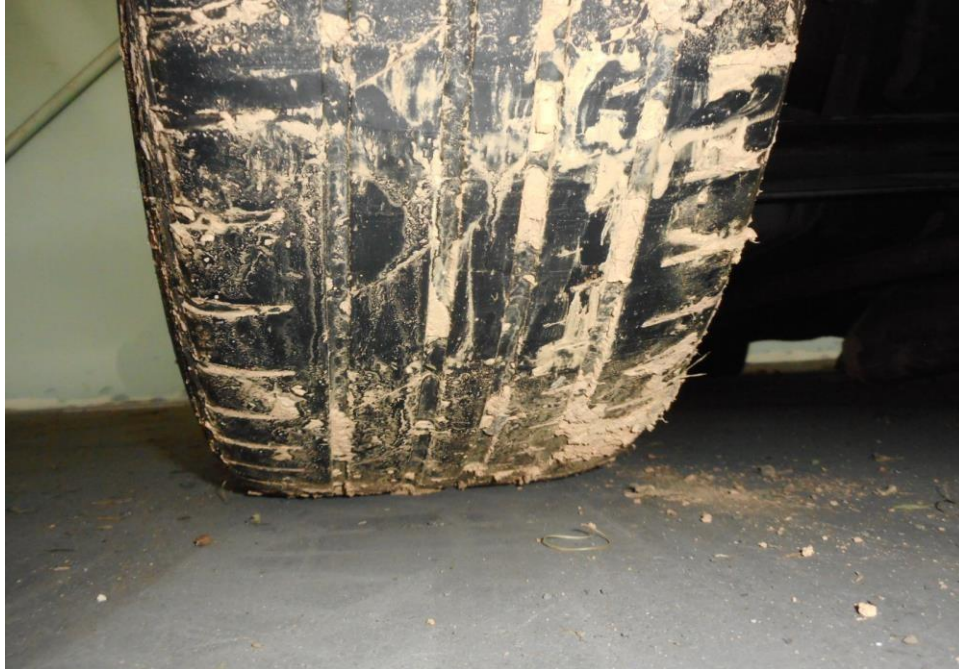
Photo 13 shows the condition of the rear left tyre of the Motor Car, which was observed to be in serviceable condition with remaining tread depth of approximately 2.4mm. The tyre, which was wrapped around alloy wheel rim, was also observed to be sufficiently inflated for vehicular operation.
