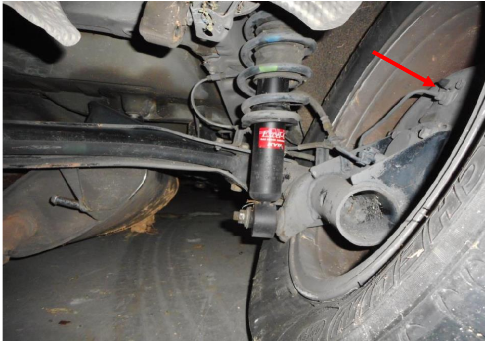
Photo 17 shows the brake hose/pipe (arrowed) at the rear right wheel of the Motor Car. No leakage of brake fluid was observed. Visual examination of the various components of the braking system like the drum brake and brake hoses had revealed to be intact and without visible damage.
