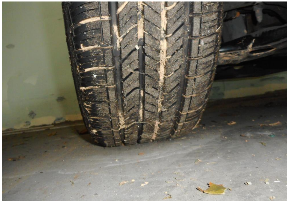
Photo 14 shows the condition of the front left tyre of the Motor Car, which was observed to be in serviceable condition with remaining tread depth of approximately 7.2mm. There was also no tear, cut or burst mark(s) on the outer and the inner sidewalls as well as across the tread of the Motor Car's 4 tyres.
