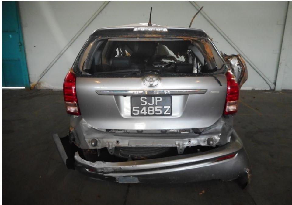
Photo 1 shows the general view of the Motor Car's rear portion at the time of my inspection. The Motor Car was observed to sustained damage at its rear portion. Its rear bumper and rear windscreen were amongst the body parts that were damaged as a result of the accident.
