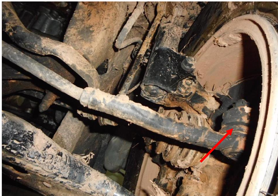
Photo 22 shows the various undercarriage components at the front right wheel of the Motor Car, in particular the steering tie rod (red arrow). The various steering components were all found to be intact, suggesting that the steering system of the Motor Car was likely to be in serviceable condition at the material time of accident. There was also no sign of fluid stain observed on the various undercarriage components at the front right wheel of the Motor Car. The undercarriage components were cover in mud as due to the result of the accident.
