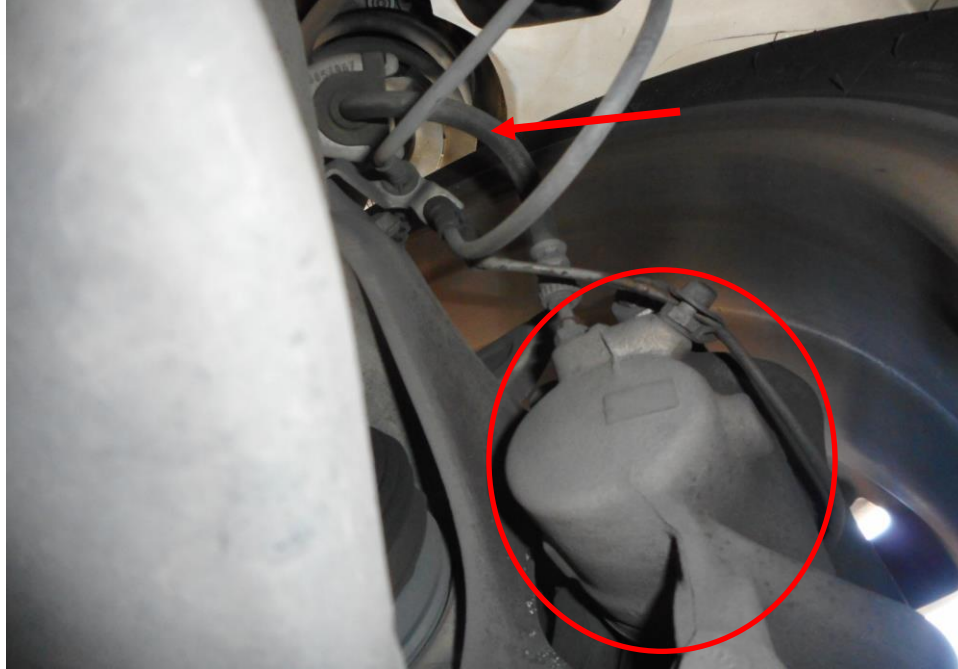
Photo 16 shows the brake hose/pipe (arrowed) at the front left wheel of the Motor Car. No leakage of brake fluid was observed. Visual examination of the various components of the braking system like the brake caliper (circled), brake booster, brake pedal etc had revealed all to be intact and without visible damage at the time of accident. There was also no sign of fluid stain(s) observed on the various undercarriage components.
