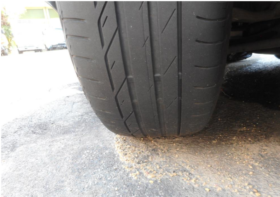
Photo 10 shows the condition of the front left tyre of the Motor Car, which was observed to be in serviceable condition with remaining tread depth of approximately 3.5mm. The tyre was also observed to be sufficiently inflated for vehicular operation with no tear, cut or burst mark(s).
