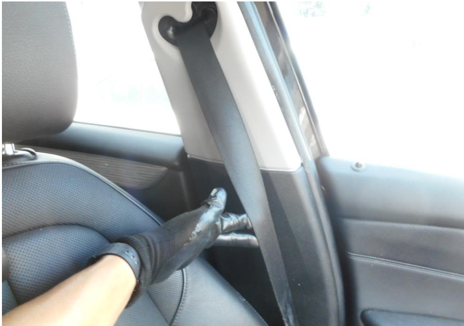
Photo 20 shows that the seat belt on the left seat was not worn at the material time of accident as the safety pre-tensioners was activated at the moment of impact and caused the seat belt to be locked into the last position.
