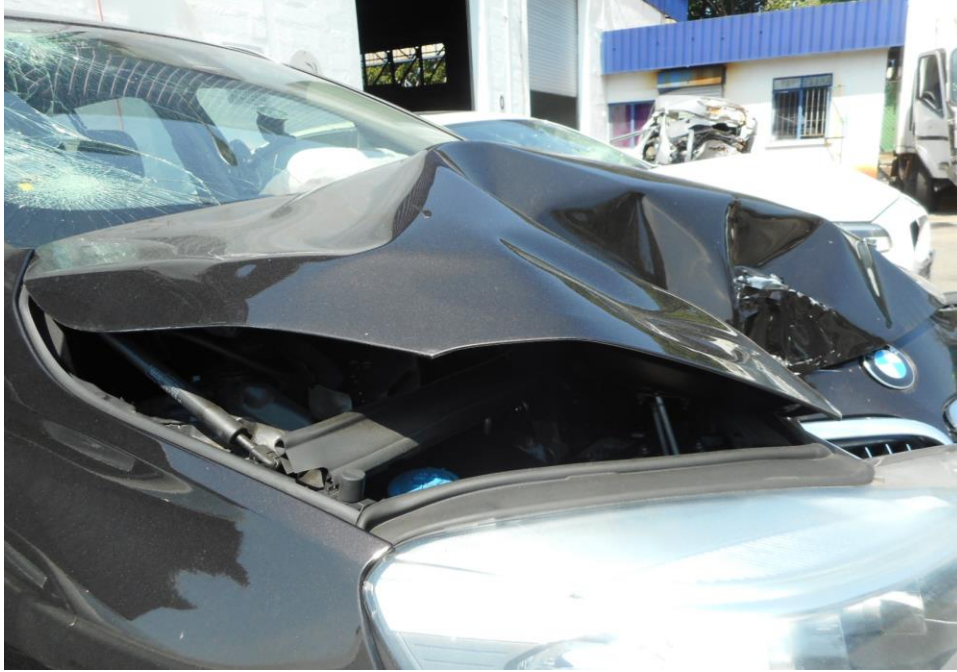
Photo 12 shows a close up view of the damaged front bonnet lock mechanism and the structure of the engine compartment of the Motor Car at the time of my inspection resulting it unable to open a result of the accident. (Unable to open)
