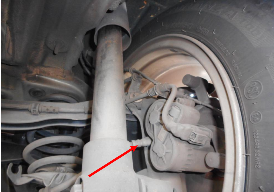
Photo 14 shows the brake hose/pipe (arrowed) at the rear right wheel of the Motor Car. No leakage of brake fluid was observed. Visual examination of the various components of the braking system like the drum brake, brake booster, brake pedal etc. had revealed all to be intact and without visible damage.
