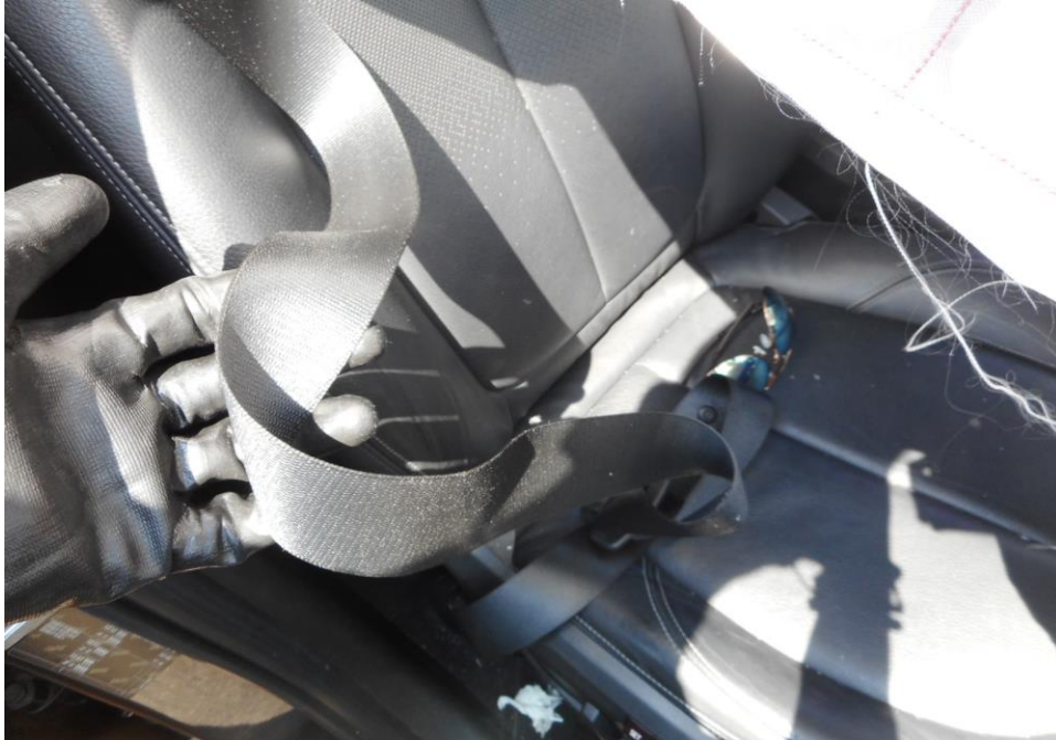
Photo 19 shows that the seat belt on the right seat was worn at the material time of accident as the safety pre-tensioners was activated at the moment of impact and caused the seat belt to be locked into the last position.
