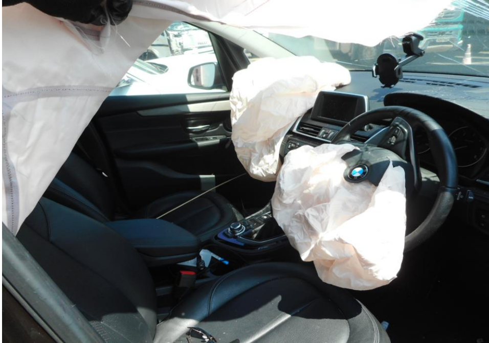
Photo 11 shows the deployment of the Supplemental Restraint System (SRS) airbag in the Motor Car as a result of the accident.
