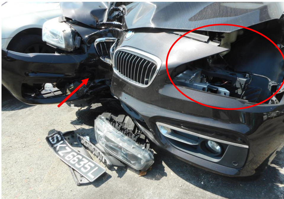
Photo 4 shows the close up view of the Motor Car's front body at the time of my inspection. The Motor car was observed to have sustained damage at its front portion. Its front left headlamp (circled) and front bumper (arrowed) was amongst the body parts and various components in the engine compartments were also damaged as a result of the accident.
