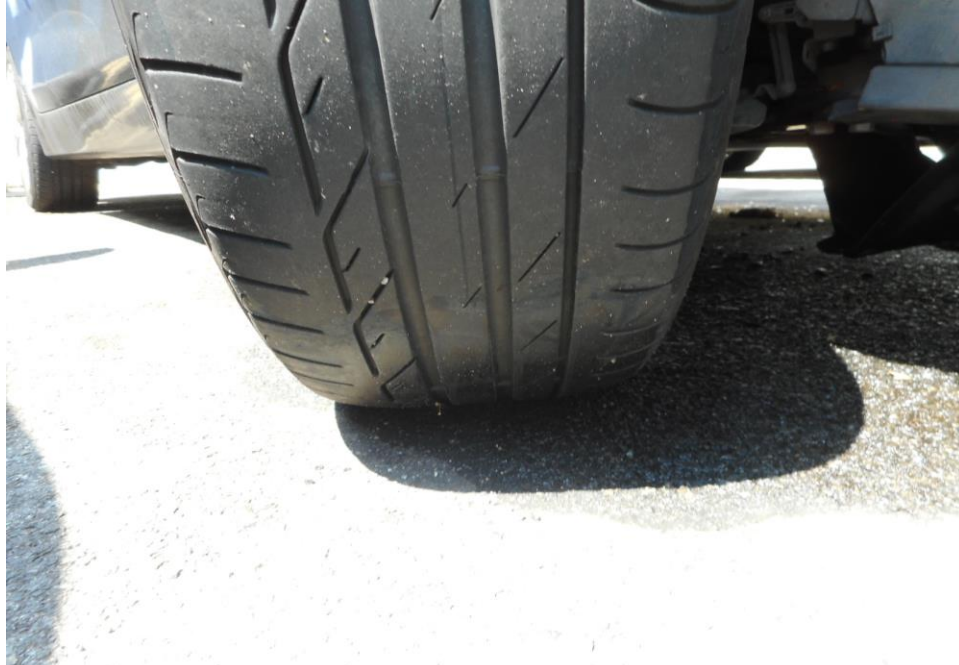
Photo 7 shows the condition of the front right tyre of the Motor Car, which was observed to be in serviceable condition with remaining tread depth of approximately 3.8mm. The tyre, which was wrapped around alloy wheel rim, was also observed to be sufficiently inflated for vehicular operation.
