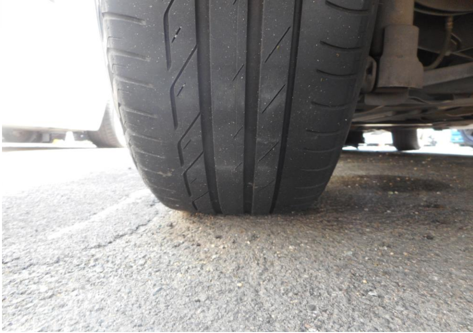
Photo 9 shows the condition of the rear left tyre of the Motor Car, which was observed to be in serviceable condition with remaining tread depth of approximately 4mm. The tyre was also observed to be sufficiently inflated for vehicular operation with no tear, cut or burst mark(s).
