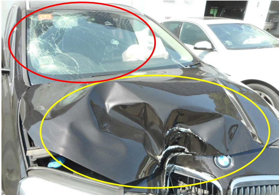
Photo 3 shows the close up view of the Motor Car's front body at the time of my inspection. The Motor car was observed to have sustained damage at its front portion. Its front windscreen (red circle) and front bonnet (yellow circle) was damaged as a result of the accident.
