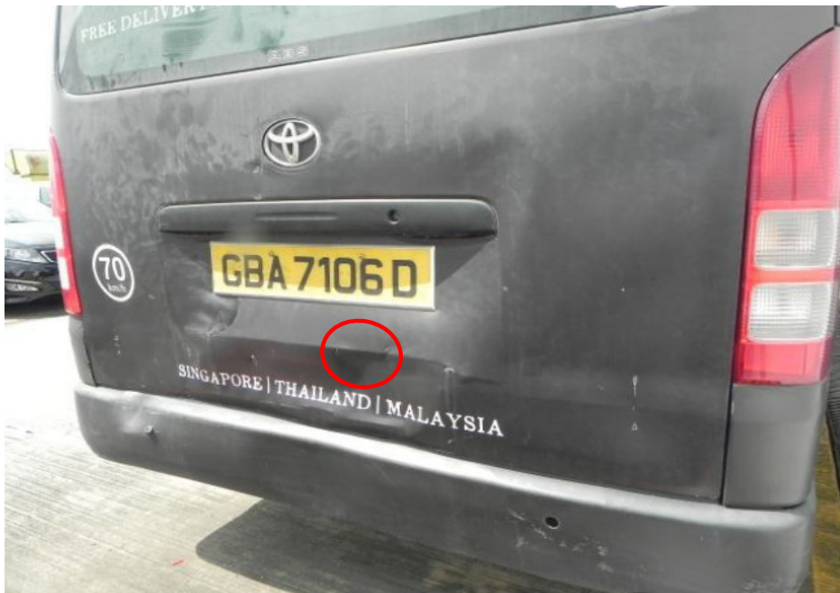
Photo 4 shows a horizontal indentation found below the rear number plate of the Toyota (circled).
