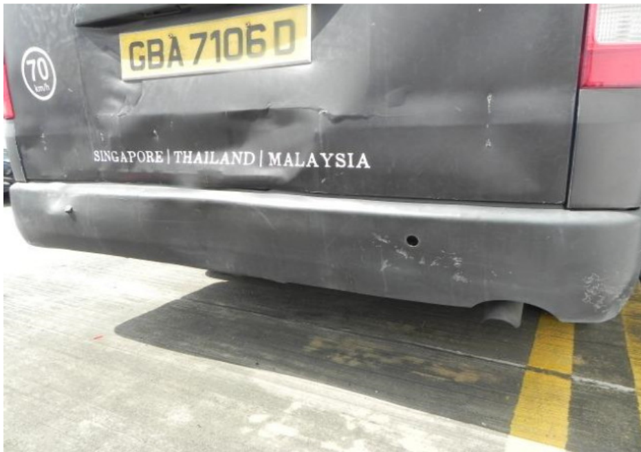
Photo 2 shows a closer view of the damages observed on the rear bumper and tail gate of the Toyota.
