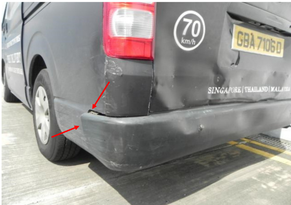
Photo 6 shows a closer view of the left corner edge of the rear bumper of the Toyota. We observed a dislodgement of the left corner edge of the rear bumper of the Toyota (arrowed).
