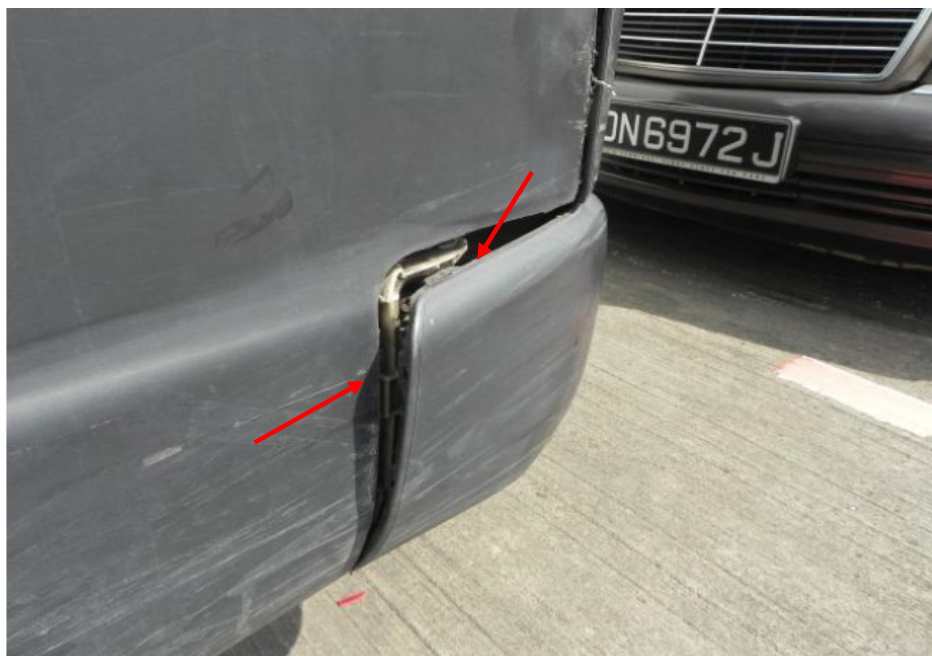
Photo 7 shows a close up view of the dislodgement observed at the left corner edge of the rear bumper of the Toyota (arrowed).
