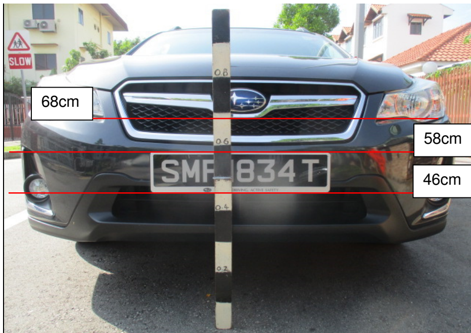
Photo 18 shows the height measurement being conducted on the front portion of the Subaru. The height range above ground level of the damages found on the front number plate and front number plate frame of the Subaru, was measured to be approximately between 46cm to 58cm. The body part at the height of 68cm above ground level was the top centre portion of the Subaru's front grille, which corresponds to the horizontal indentation found on the Toyota's tail gate.
