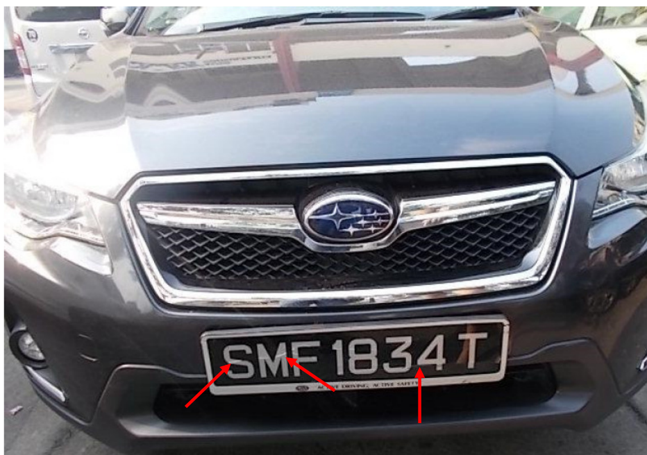
Photo 9 shows a closer view of the cracked front number plate of the Subaru at the time of reporting, which was 1 day after the accident (red arrows).
