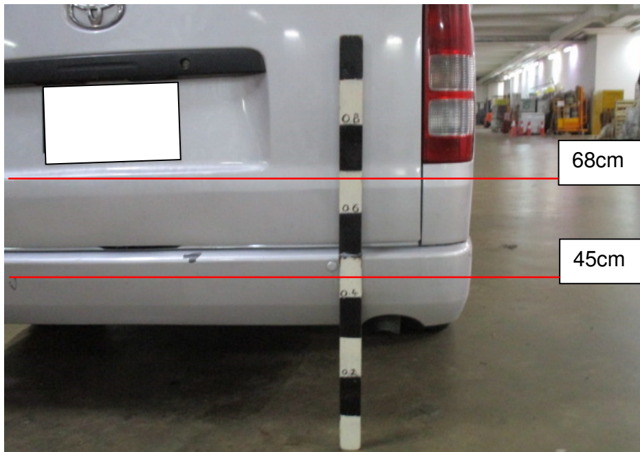
Photo 17 shows the height measurement being conducted on the rear portion of the Toyota (using a similar make and model). The height range above ground level of the damages found on the Toyota, was measured to be approximately between 45cm to 68cm.
