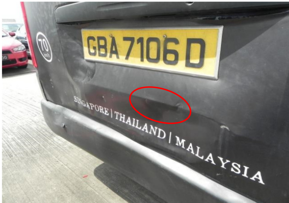
Photo 5 shows a close up view of the horizontal indentation found below the rear number plate of the Toyota (circled).
