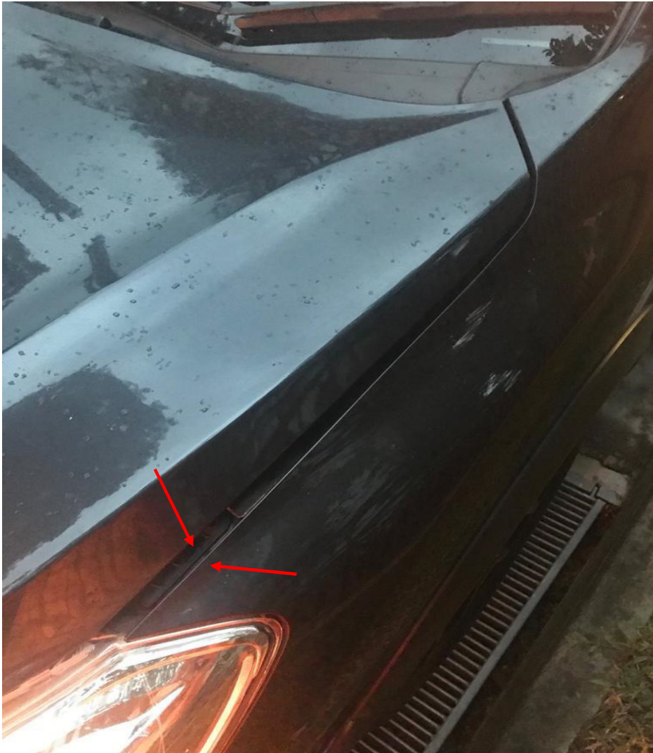
Photo 16 shows the slight misalignment of the front bonnet and left front fender of the Subaru post- accident (arrowed) which indicates there was damage to the front bonnet of the Subaru.
