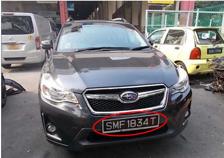
Photo 8 shows the general view of the front of the Subaru at the time of reporting, which was 1 day after the accident. The damage to the Subaru was observed to be confined to its front number plate. The front number plate appears to be cracked (circled).
