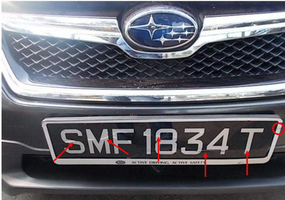
Photo 10 shows a close up view of the cracked front number plate of the Subaru (red arrows). Upon closer examination, we also observed scuff marks on the left corner of the front number plate frame (circled).
