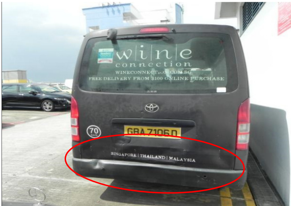
Photo 1 shows the general view of the rear portion of the Toyota at the time of the Pre- Repair Survey conducted by STA Inspection Pte. Ltd. The damage to the Toyota was observed to be confined to the rear bumper and tail gate (circled).
