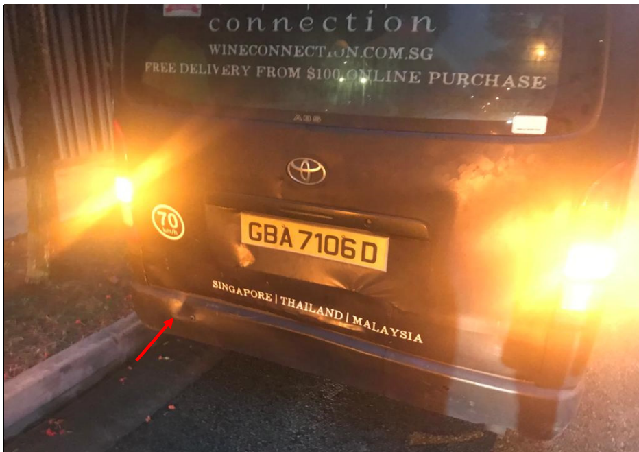
Photo 13 shows a closer view of the rear portion of the Toyota post- accident. Upon closer examination, we observed a dent on the left portion of the Toyota's rear bumper (arrowed).
