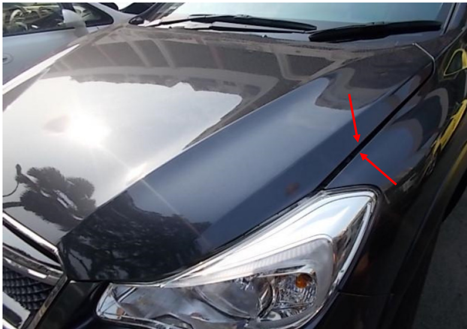
Photo 11 shows a closer view of the left corner edge of the front bonnet and left front fender of the Subaru. We observed that there was a slight misalignment at the corner edges (red arrows) which indicates there was damage to the front bonnet of the Subaru.
