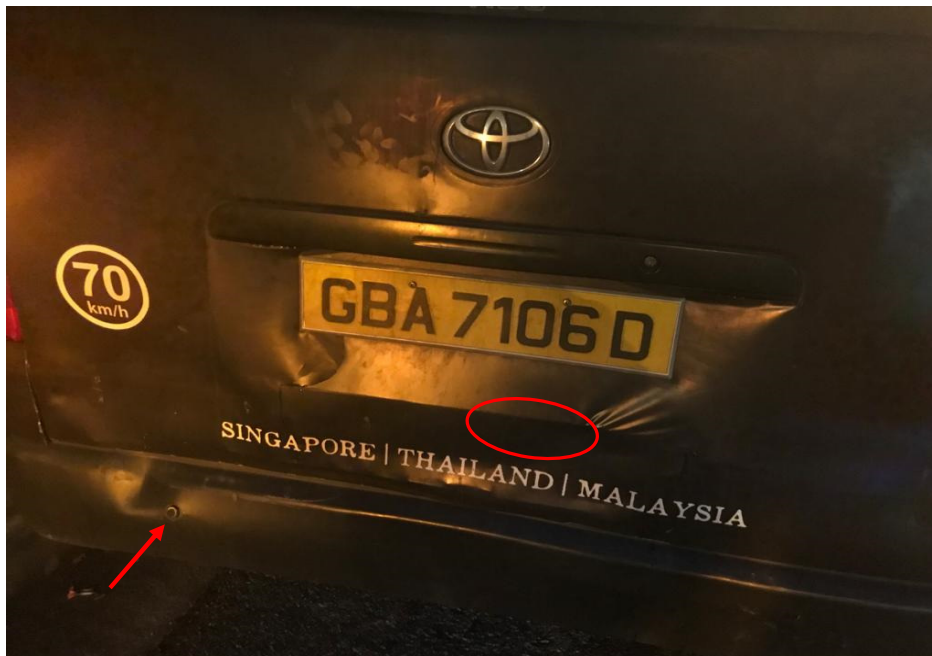
Photo 14 shows a close up view of the rear portion of the Toyota post- accident. Upon closer examination, we also observed the dislodged reverse sensor on the left portion of the Toyota's rear bumper (arrowed) as well as a horizontal indentation which resembled the top centre portion of the Subaru's front grille (circled).
