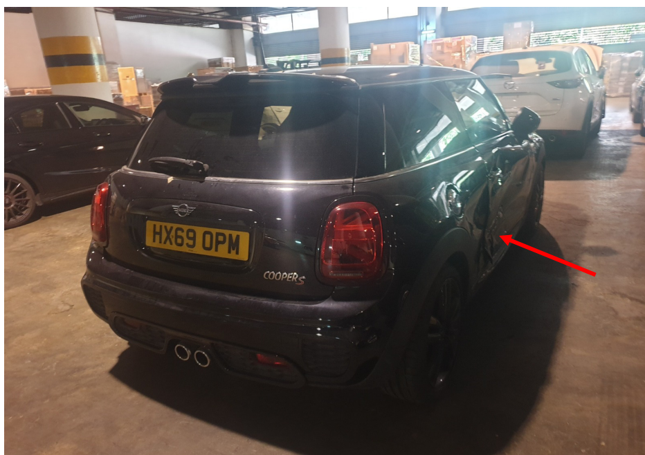
Photo 2 shows the rear right body of the Motor Car (photograph provided to me). The Motor Car was observed to have sustained damage at its right side centre portion (arrowed). The front right door, right side rocker panel garnish and rear right body panel were amongst the body parts that were observed to have been damaged.
