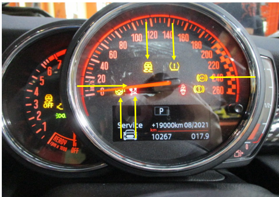
Photo 12 shows the warning lights for the various electronic safety features appearing on the instrument panel of the Motor Car during its self-test when the engine is cranked, in particular the ABS, SRS, PAS, TPM and DSC lights (arrowed).
