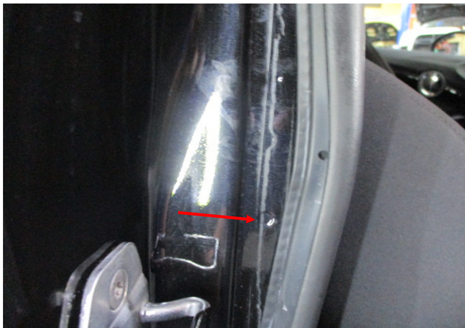
Photo 21 shows the rear right body panel of the Motor Car. I did not find any weld marks other than original spot weld marks (arrowed) on the rear right body panel of the Motor Car which, indicates that there was no re-welding works carried out. In general, I had found all the non-detachable body panels of the Motor Car to be originally fitted at the time of my inspection.
