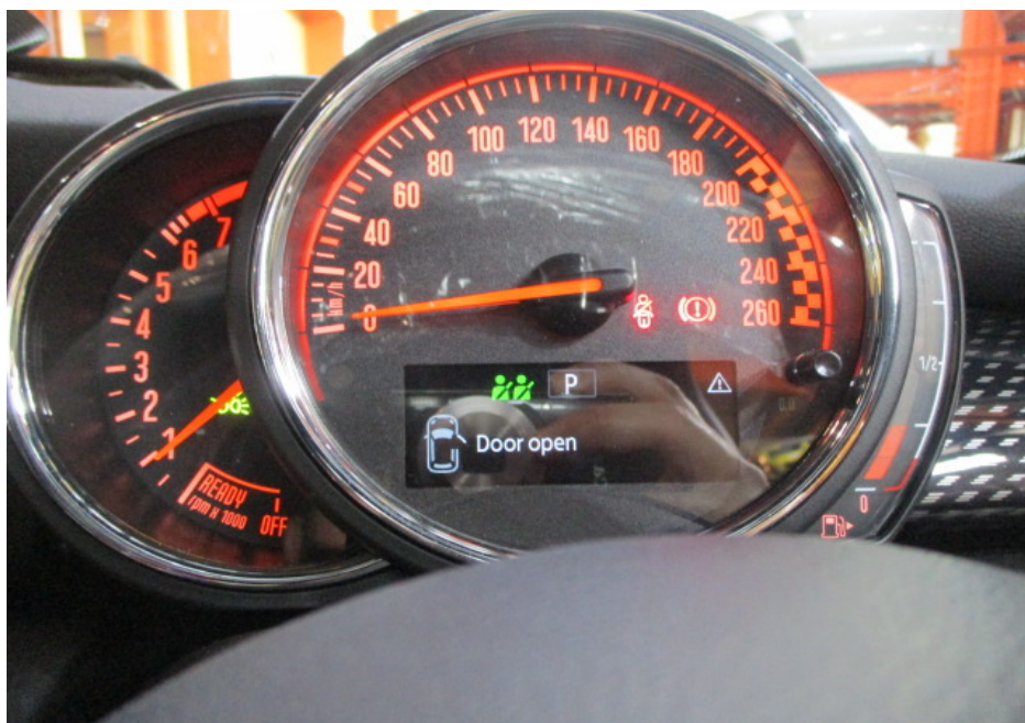
Photo 13 shows the respective warning lights no longer illuminated, indicating that there is no fault detected to the ABS, SRS, PAS, TPM and DSC systems of the Motor Car during the self-test. These electronic systems were hence in working condition at the time of my inspection.
