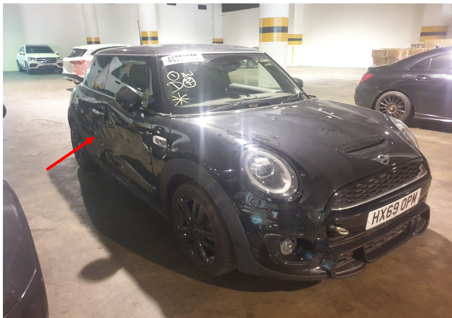
Photo 1 shows the front right body of the Motor Car (photograph provided to me). The Motor Car was observed to have sustained damage at its right side centre portion (arrowed). The front right door, right side rocker panel garnish and rear right body panel were amongst the body parts that were observed to have been damaged.
