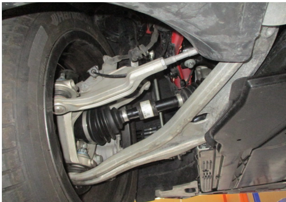
Photo 13 shows the various undercarriage components at the front left wheel of the Motor Car. The mechanical components, control arms and linkages were all found to be intact and secured in an appropriate manner.
