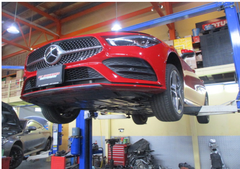
Photo 11 shows the Motor Car hoisted up for checks on its undercarriage. There was no sign(s) or indication(s) of fluid leakage and/or fluid stain(s) on the underside of the Motor Car. The undercarriage components of the Motor Car were also all observed to be intact and secured in an appropriate manner.
