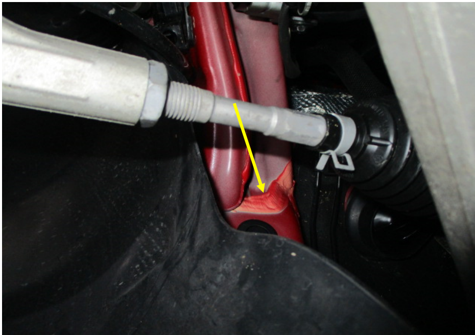
Photo 16 shows the chassis/structural body at the underside front right of the Motor Car. I did not find any weld marks other than original spot weld marks on the chassis/structural body of the Motor Car. The original factory sealant (arrowed) at the joints along the chassis/structural body was untouched, indicating no work was done on the chassis/structural body of the Motor Car and that the chassis/structural body was originally fitted.
