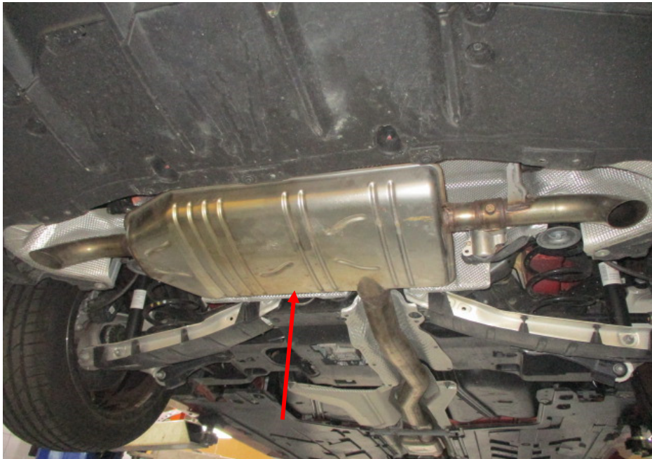
Photo 15 shows the Motor Car's rear muffler (arrowed). My examination of the Motor Car's exhaust system revealed no sign(s) or indication(s) of any cut or weld marks along its exhaust pipes and on its catalytic converter.
