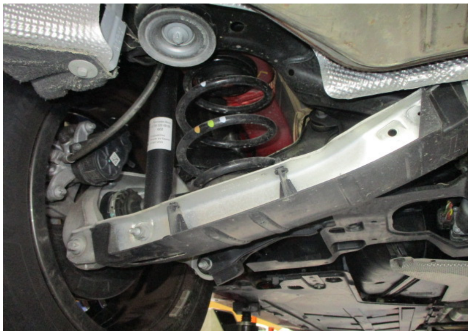
Photo 12 shows a general view of the control arms and linkages at the rear left wheel of the Motor Car. I did not observe any fluid leak and/or fluid stain on the underside of the Motor Car. All of the Motor Car's undercarriage components were observed to be intact and secured in an appropriate manner.
