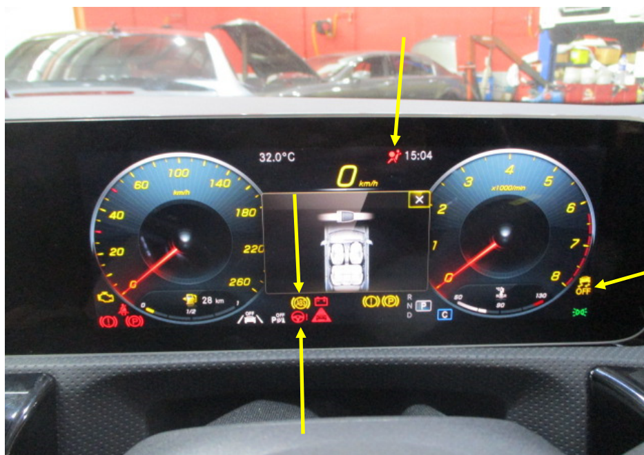
Photo 9 shows the warning lights for the various electronic safety features appearing on the instrument panel of the Motor Car during its self-test when the engine is cranked, in particular the ABS, SRS, EPS and TCS lights (arrowed).
