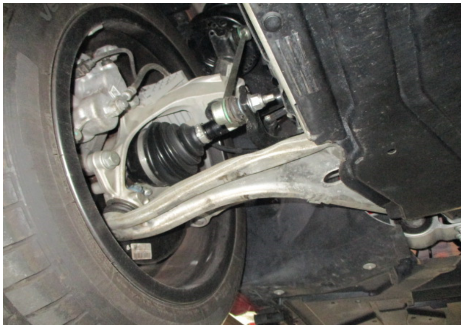
Photo 14 shows the various undercarriage components at the front right wheel of the Motor Car. The mechanical components, control arms and linkages were all found to be intact and secured in an appropriate manner. I also did not observe any fluid leak and/or fluid stain on the underside of the Motor Car.
