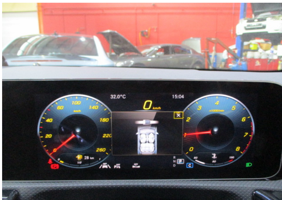
Photo 10 shows the respective warning lights no longer illuminated, indicating that there is no fault detected to the ABS, SRS, EPS and TCS systems of the Motor Car during the self-test. These electronic systems were hence in working condition at the time of my inspection.
