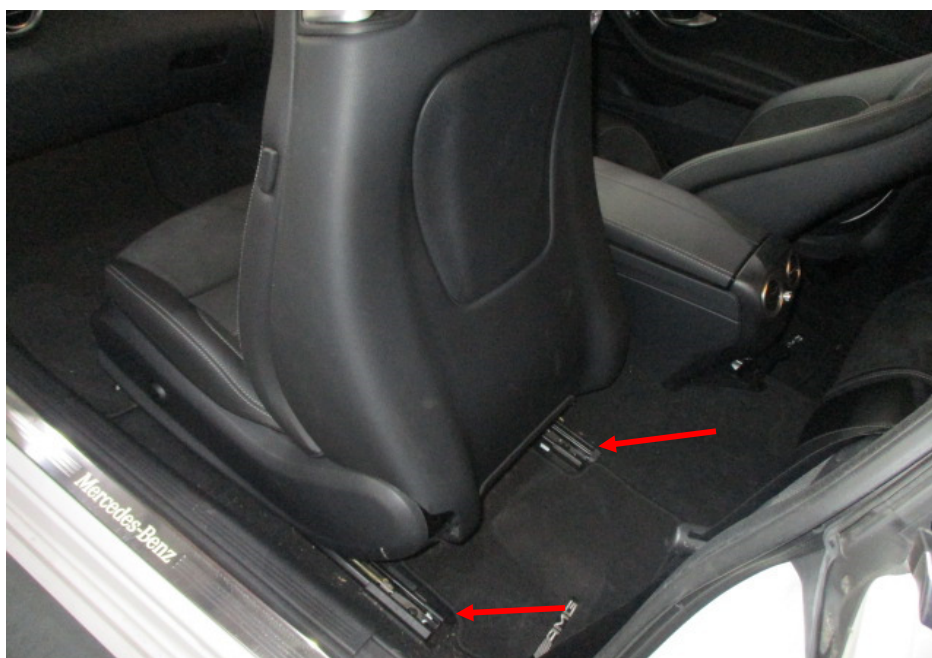
Photo 12 shows the front left seat of the Motor Car. All the seats of the Motor Car were secured via seat rails (arrowed) to the floorboard and were fitted with a retractable seat belt reel and pre-tensioner. The seat belts were tested and were able to be fastened into the respective pre-tensions that were fitted on the side of each individual seat.
