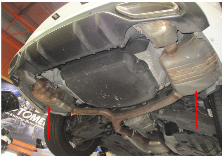
Photo 19 shows the Motor Car's rear mufflers (arrowed). My examination of the Motor Car's exhaust system revealed no sign(s) or indication(s) of any cut or weld marks along its exhaust pipes and on its catalytic converter.
