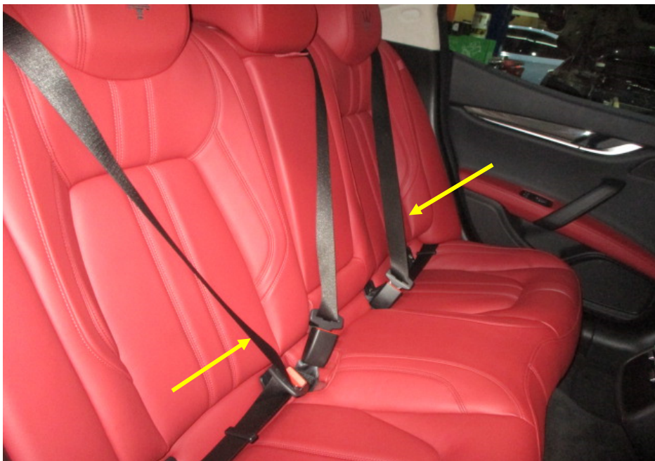
Photo 12 shows the rear seats of the Motor Car. All the seats of the Motor Car were secured via seat rails to the floorboard. They were also fitted with a retractable seat belt reel and a pre-tensioner. The seat belts (arrowed) were tested and were able to be fastened into the respective pre-tensions that were fitted on the side of each individual seat.
