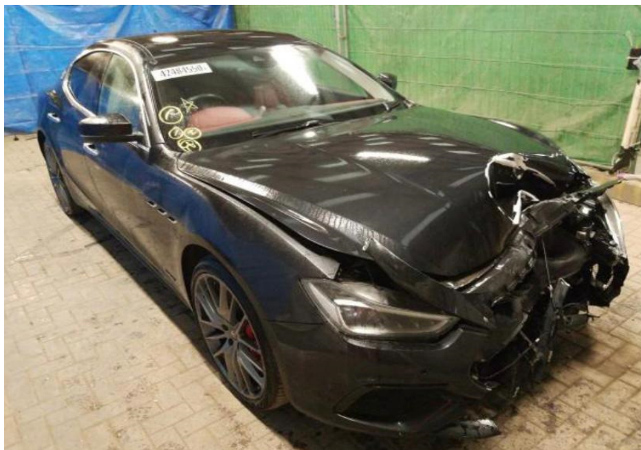
Photo 1 shows the front right body of the Motor Car (photograph provided to me). The Motor Car was observed to have sustained damage at its frontal portion. The front bumper, front right headlamp, front radiator grille, front bumper centre lower grille and front bonnet were amongst the body parts that were observed to have been damaged.
