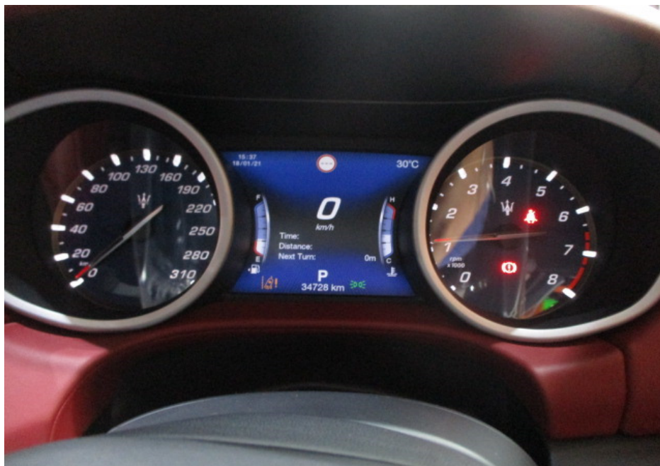
Photo 14 shows the respective warning lights no longer illuminated, indicating that there is no fault detected to the ABS, SRS, TPM and TC systems of the Motor Car during the self-test. These electronic systems were hence in working condition at the time of my inspection.
