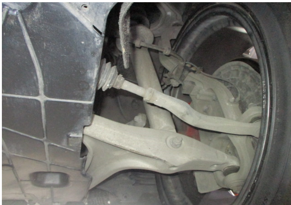
Photo 17 shows the various undercarriage components at the front right wheel of the Motor Car. The mechanical components, control arms and linkages were all found to be intact and secured in an appropriate manner.
