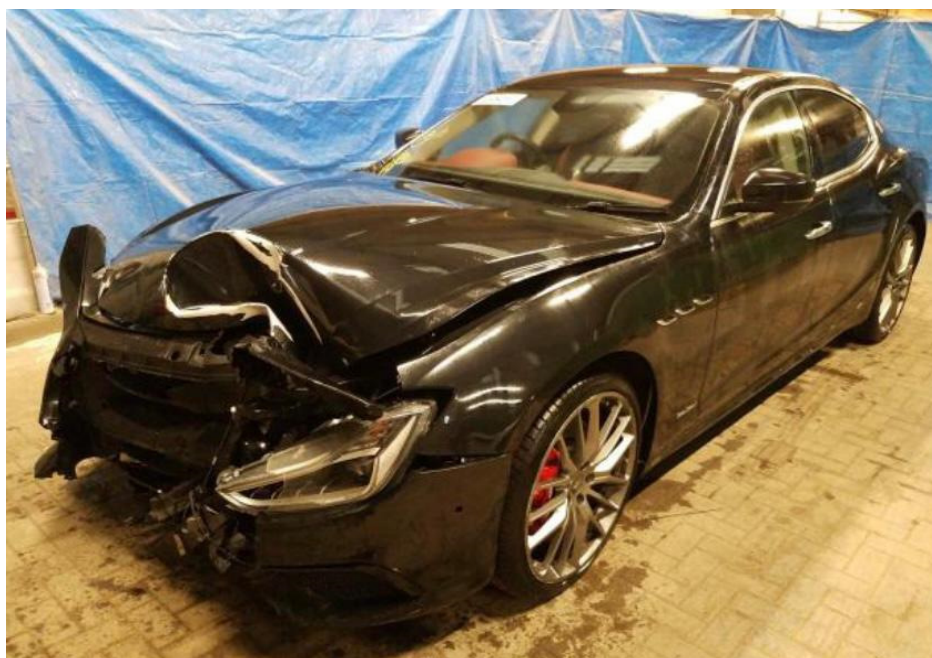
Photo 2 shows the front left body of the Motor Car (photograph provided to me). The Motor Car was observed to have sustained damage at its frontal portion. The front bumper, front left headlamp, front radiator grille, front bumper centre lower grille, front left fender and front bonnet were amongst the body parts that were observed to have been damaged.
