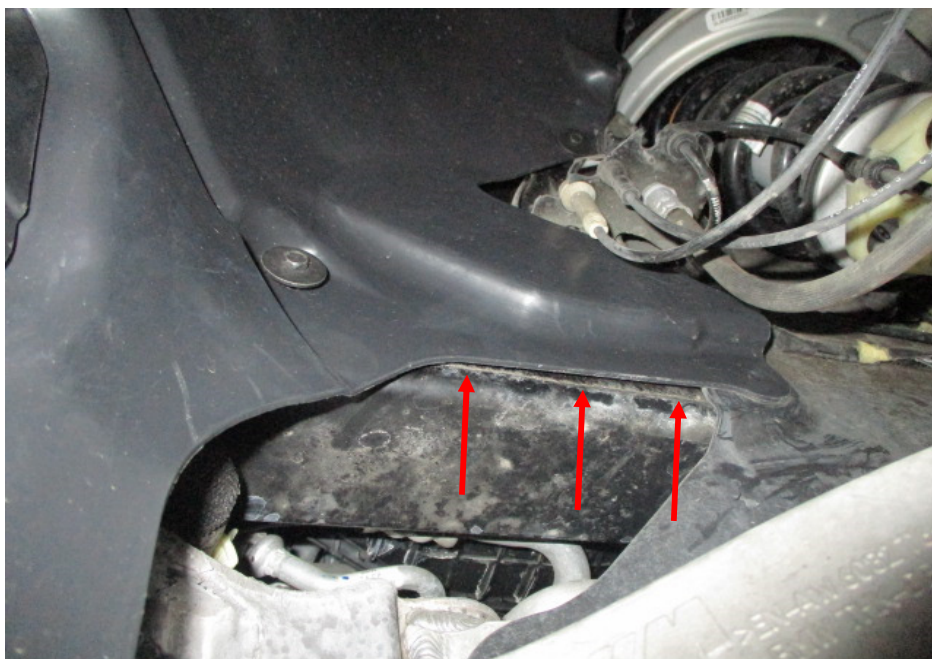
Photo 22 shows the chassis/structural body at the underside front left of the Motor Car. The original factory sealant (arrowed) at the joints along the chassis/structural body was observed to be untouched. In general, I had found no work was carried out on the chassis/structural body of the Motor Car. The chassis/structural body of the Motor Car was originally fitted.
