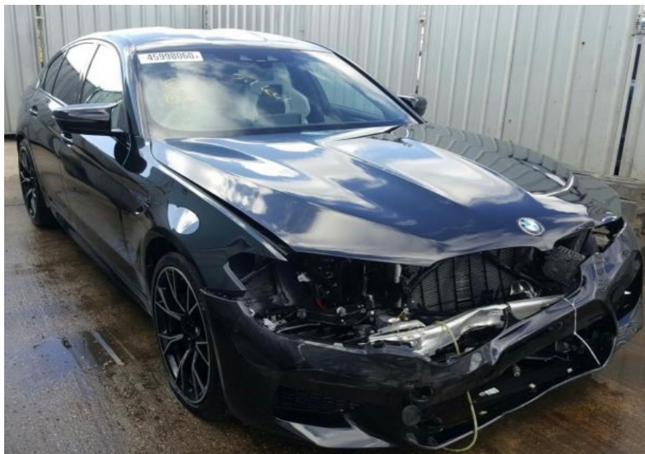
Photo 1 shows the front right body of the Motor Car (photograph provided to me). The Motor Car was observed to have sustained damage at its frontal portion. The front bumper, front right headlamp, front grilles, front bumper reinforcement and front bonnet were amongst the body parts that were observed to have been damaged.
