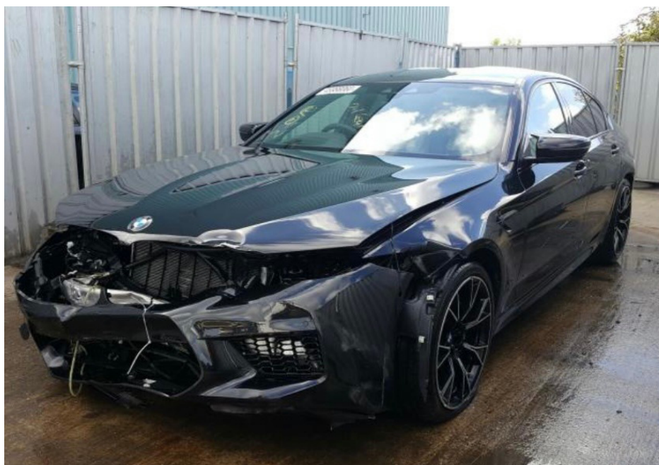
Photo 2 shows the front left body of the Motor Car (photograph provided to me). The Motor Car was observed to have sustained damage at its frontal portion. The front bumper, front left headlamp, front grilles, front bumper centre lower grille, front brace panel, aircon condenser, front left fender and front bonnet were amongst the body parts that were observed to have been damaged.
