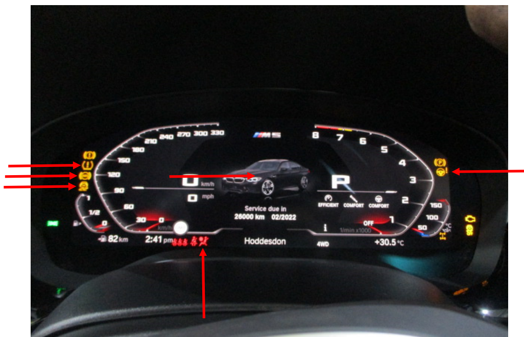
Photo 13 shows the warning lights for the various electronic safety features appearing on the instrument panel of the Motor Car during its self-test when the engine is cranked, in particular the ABS, SRS, IAS, TPM and DSC lights (arrowed).
