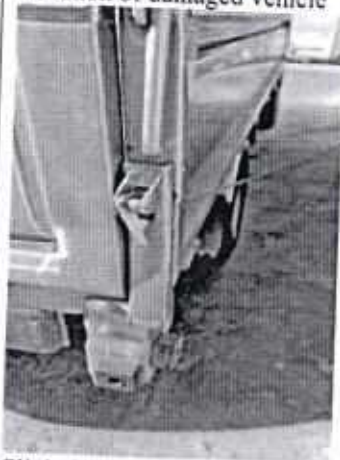
Slight bending of loading bed door lever
