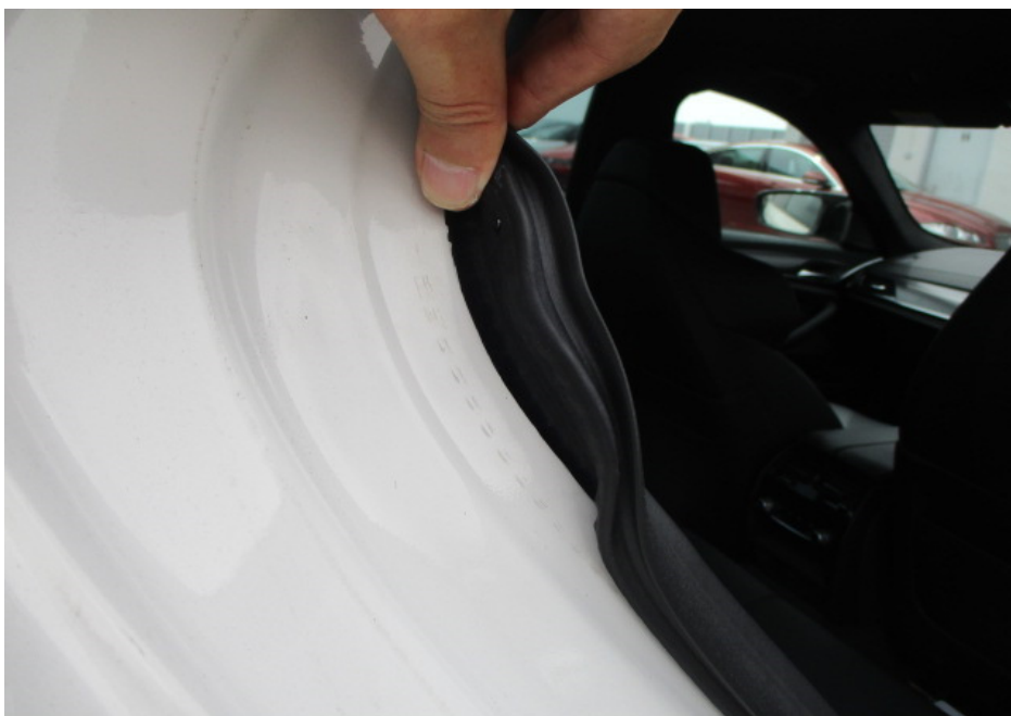
Photo 22 shows the right side "C" pillar of the Motor Car. I did not find any original weld marks at the right side "C" pillar of the Motor Car, indicating that the rear right fender of the Motor Car was replaced. The lack of original weld marks seen was due to replacement work when the replaced rear right fender was re-welded onto the Motor Car and smoothen for re-spraying work.
