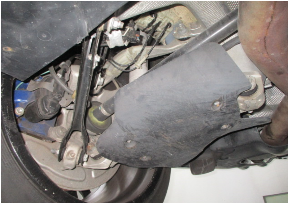
Photo 15 shows a general view of the control arms and linkages at the rear right wheel of the Motor Car. I did not observe any fluid leak and/or fluid stain on the underside of the Motor Car. All of the Motor Car's undercarriage components were observed to be intact and secured in an appropriate manner.
