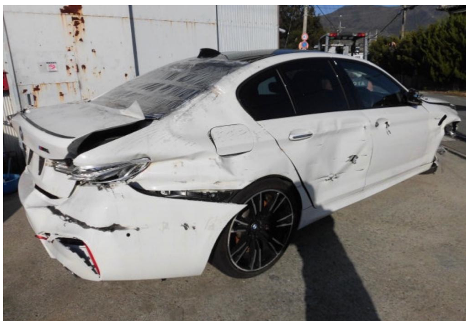
Photo 2 shows the rear right body of the Motor Car prior to any repairs being carried out (photograph provided to me). Apart for the frontal portion, the Motor Car had also sustained damage at its rear portion and along its right side portion. The rear windscreen of the Motor Car was also observed to be shattered. Body parts damaged include the rear bumper, rear bootlid, rear right fender and rear right door amongst others.
