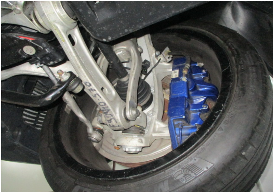
Photo 17 shows the various undercarriage components at the front right wheel of the Motor Car. The mechanical components, control arms and linkages were all found to be intact and secured in an appropriate manner. I did not observe any fluid leak and/or fluid stain on the underside of the Motor Car.
