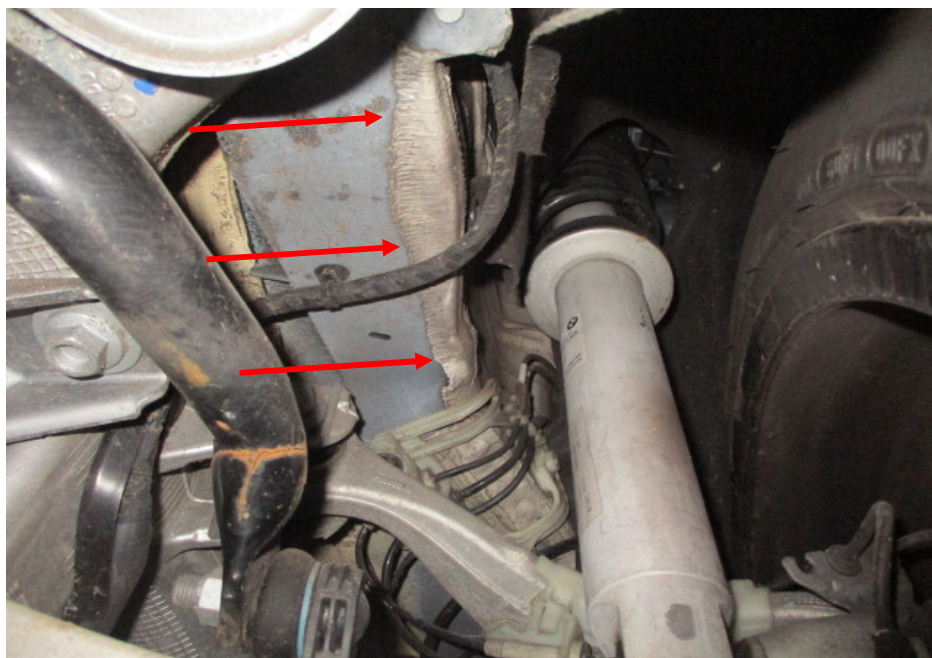
Photo 20 shows the chassis/structural body at the underside rear right of the Motor Car. Visually, I did not find any weld marks other than original spot weld marks on the chassis/structural body of the Motor Car. The original factory sealant (arrowed) at the joints along the chassis/structural body was also untouched, indicating no work was done on the chassis/structural body of the Motor Car and that the chassis/structural body was originally fitted.
