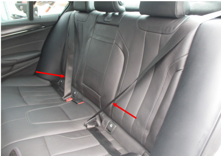
Photo 11 shows the rear seats of the Motor Car. All the seats of the Motor Car were secured via seat rails to the floorboard. They were also fitted with a retractable seat belt reel and a pre-tensioner. The seat belts (arrowed) were tested and were able to be fastened into the respective pre-tensions that were fitted on the side of each individual seat.
