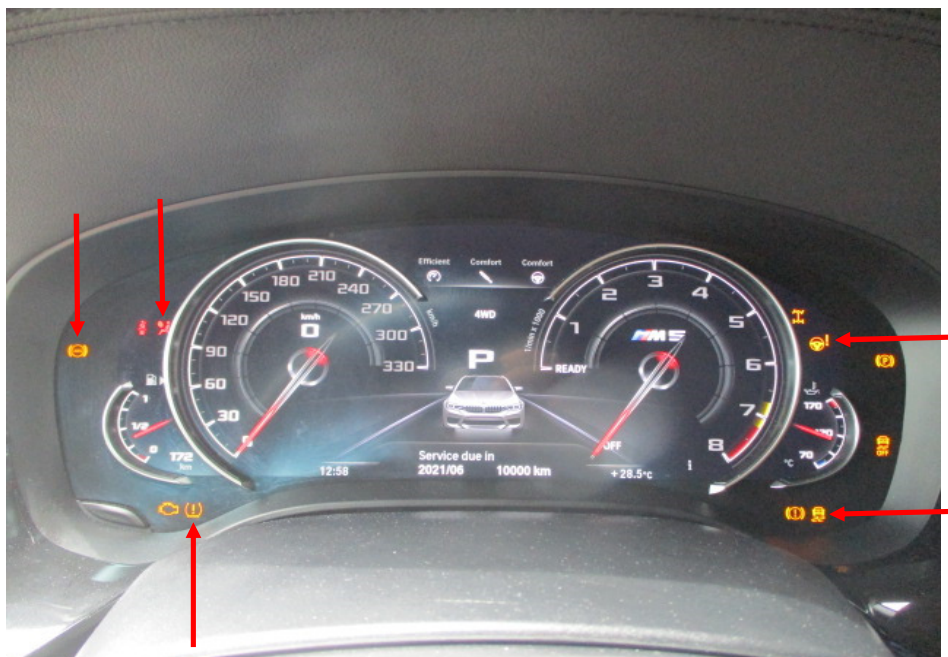
Photo 12 shows the warning lights for the various electronic safety features appearing on the instrument panel of the Motor Car during its self-test when the engine is cranked, in particular the ABS, SRS, IAS, TPM and DSC lights (arrowed).
