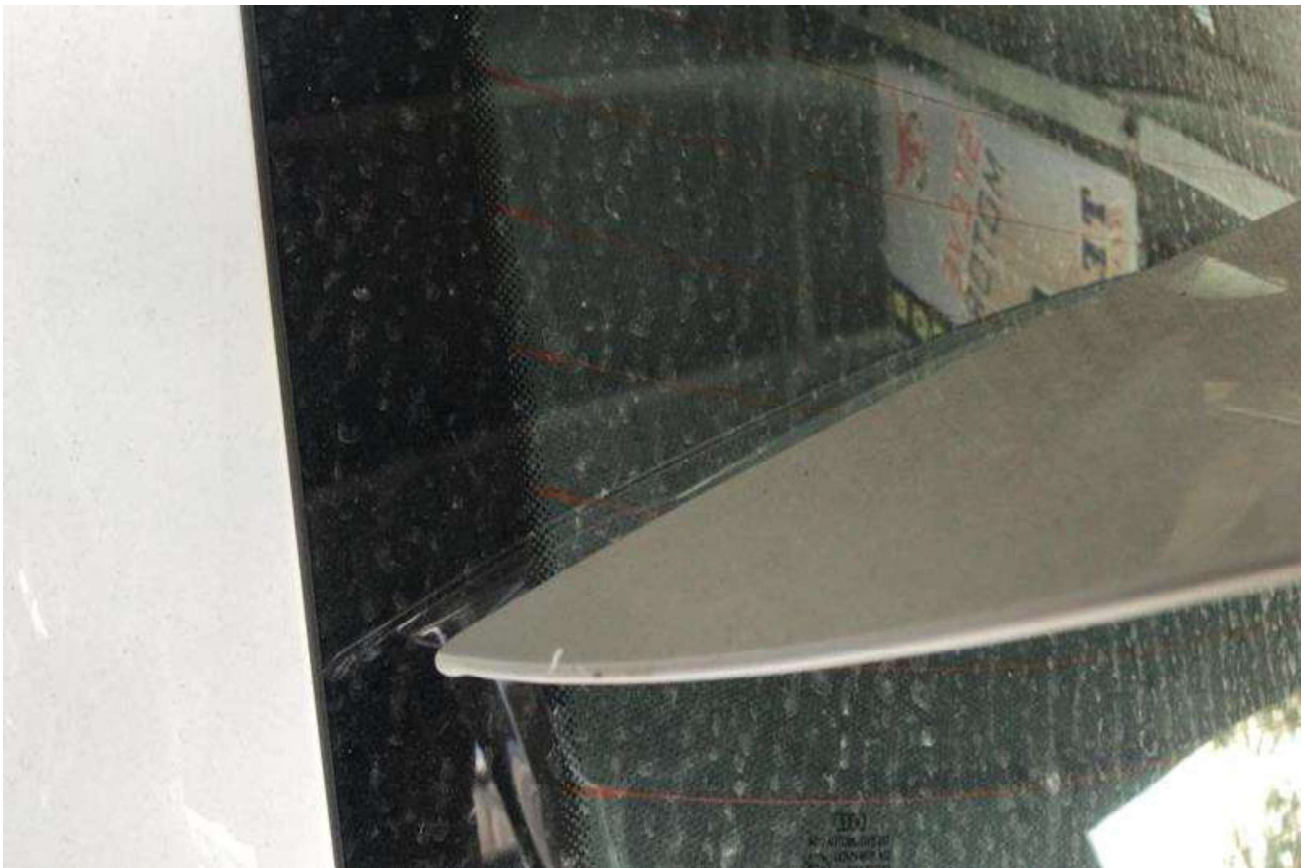
Photo 16 REAR BOOTLID PANEL CUT/SCRATCHED - REPAIR
