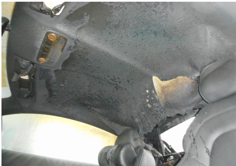
Photo 8 shows the close up interior view from the left side of the Insured Vehicle at the time of our inspection. The rear sight glass, rear seat compartment fittings and the seats material of the Insured Vehicle were observed to suffer smoke and heat damage as a result of the fire.
