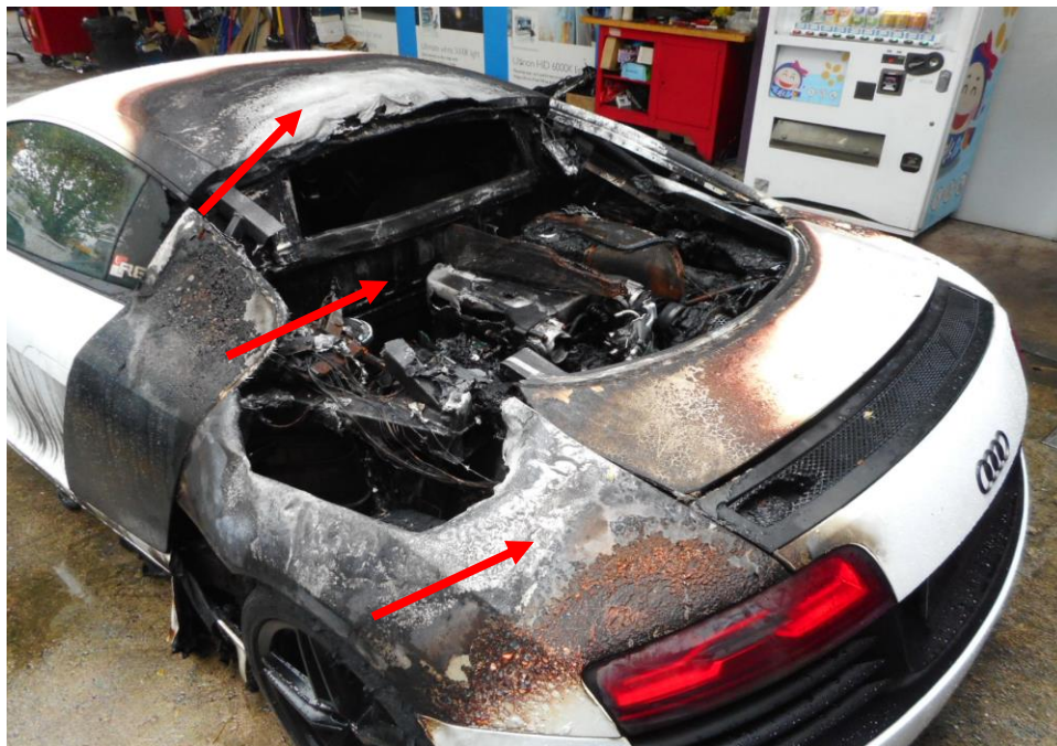
Photo 10 shows the roof and the surrounding of the middle portion (arrowed) of the Insured Vehicle at the time of our inspection. The high heat intensity burn marks (whitish burn marks) and rust that had development found on the exterior surface of the roof metal body and the surrounding area indicates that the fire had originated from the engine compartment of the Insured Vehicle.
