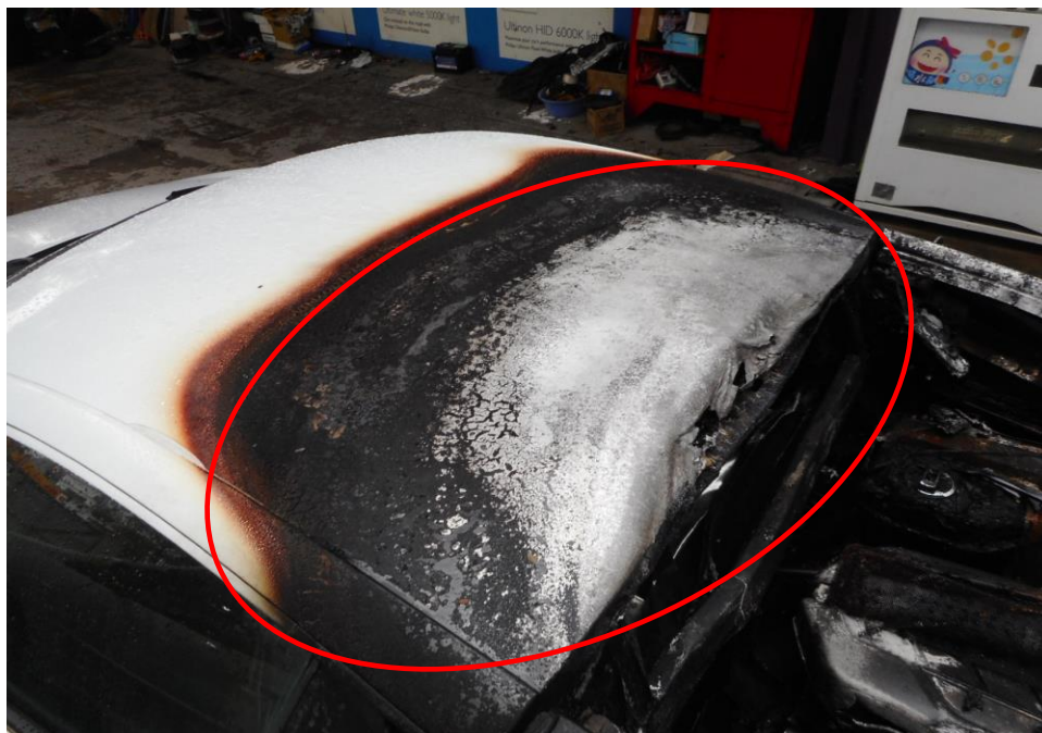
Photo 11 shows the roof and the surrounding of the middle portion (circled) of the Insured Vehicle at the time of our inspection. The high heat intensity burn marks (whitish burn marks) and rust that had development found on the exterior surface of the roof metal body and the surrounding area indicates that the fire had originated from the engine compartment of the Insured Vehicle.
