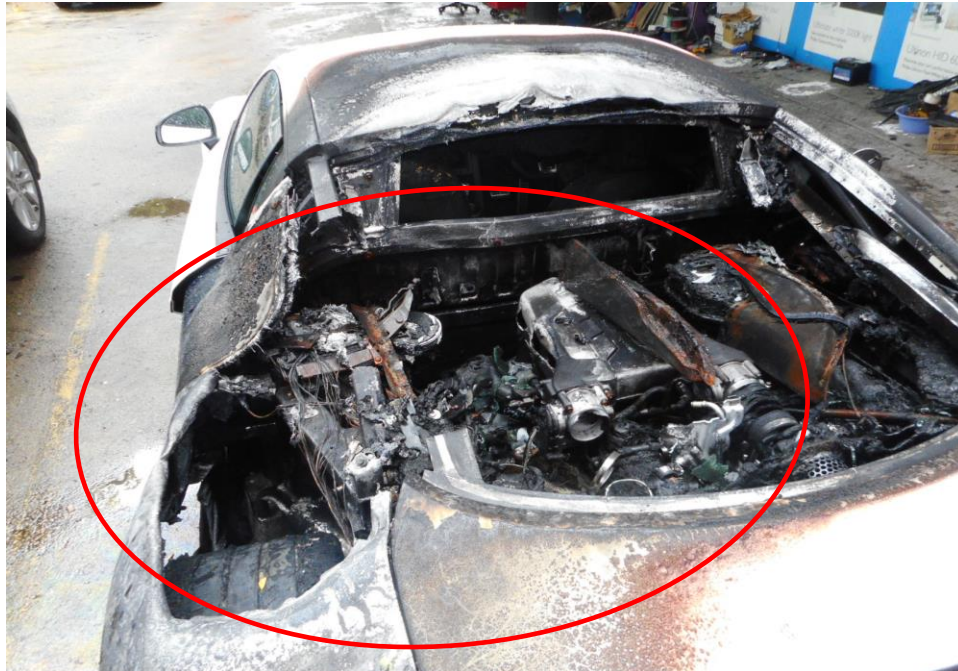
Photo 12 shows the general view of the rear left engine compartment portion of the Insured Vehicle where the fire had likely started. The engine cover and the surrounding area had whitish burn marks due to high heat intensity burn on the Insured vehicle (circled)
