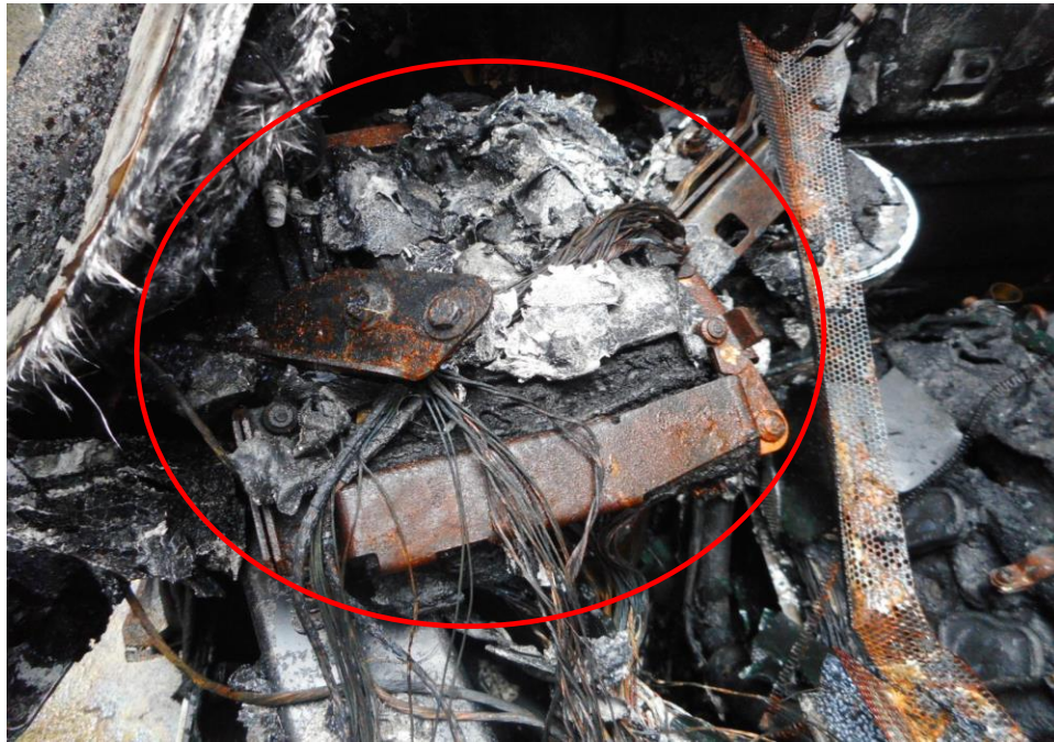
Photo 5 shows the engine compartment of the Insured Vehicle at the time of our inspection. The engine ecu (circled) was observed to be severely burnt. Most of the parts inside the engine compartment were found to be burnt and/or melted as a result of the fire.
