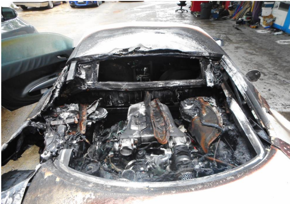
Photo 4 shows the general view of the engine compartment of the Insured Vehicle at the time of our inspection. The Insured Vehicle was observed to have sustained severe fire damage. Its engine cover and engine compartment was completely burnt. Rust had accumulated around the engine compartment of the Insured Vehicle as a result of exposure to environmental condition for a period of time.
