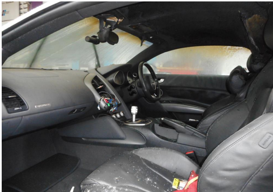
Photo 7 shows the interior view from the right side of the Insured Vehicle at the time of our inspection. The interior fittings of the Insured Vehicle were observed to suffer smoke and heat damage as a result of the fire.
