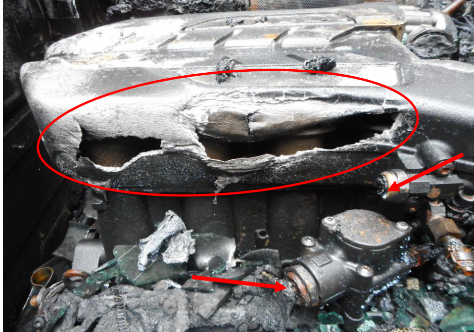
Photo 14 shows the close up view of the left rear engine compartment area where the fire had likely started and spread around the engine compartment. Observed was a broken fuel hose (red arrow) from the high pressure fuel pump which had likely caused a fuel leakage onto and around the hot surface of the running engine components which was likely the cause of fire. The fire's high heat intensity burn from this area had also resulted in whitish burn marks and cracks to the engine cover) (red circle) of the Insured Vehicle.
