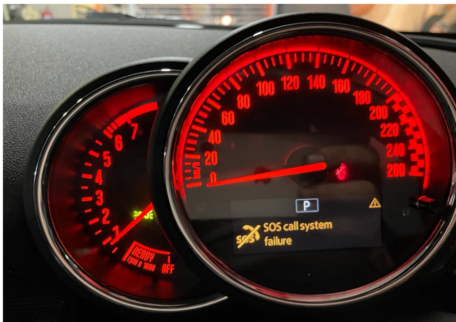
Photo 14 shows the respective warning lights no longer illuminated, indicating that there is no fault detected to the ABS, SRS, PAS, TPM and DSC systems of the Motor Car during the self-test. These electronic systems were hence in working condition at the time of my inspection.
