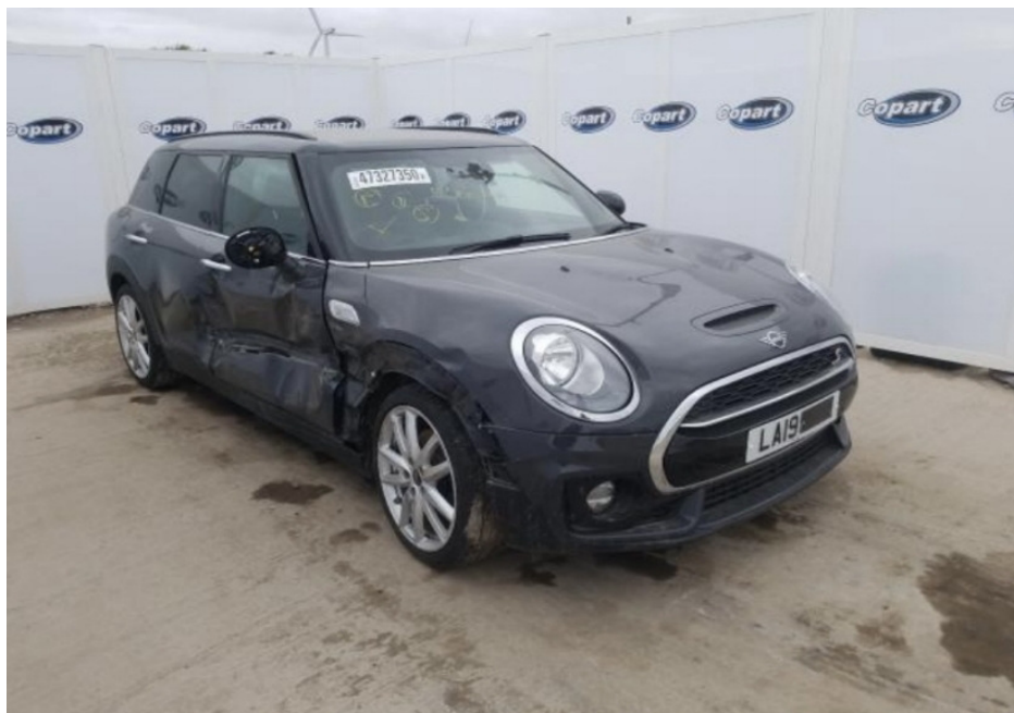
Photo 1 shows the front right body of the Motor Car (photograph provided to me). The Motor Car was observed to have sustained damage along its right side portion. The front bumper, front bonnet, front right fender, front right wheel arc garnish, front right door and right side wing mirror were amongst the body parts that were observed to have been damaged.
