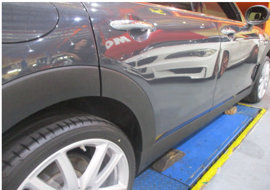
Photo 9 shows a closer view of the rear right door and right side rocker panel garnish of the Motor Car at the time of my inspection. The body parts along the right side portion of the Motor Car were visually examined and it was observed that the repair/restoration works carried out to the damaged area of the Motor Car (refer to photograph 1 & 2 above) were reasonably adequate and in order.
