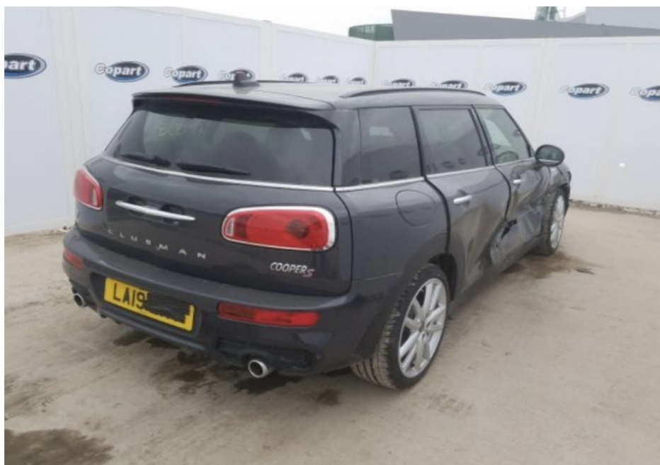
Photo 2 shows the rear right body of the Motor Car (photograph provided to me). The Motor Car was observed to have sustained damage along its right side portion. The front right door, rear right door and right side rocker panel garnish were amongst the body parts that were observed to have been damaged.
