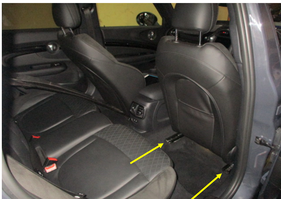
Photo 12 shows the seats of the Motor Car, which were secured via seat rails (arrowed) to the floorboard. All the seats of the Motor Car were fitted with a retractable seat belt reel and pre-tensioner. The seat belts were tested and were able to be fastened into the respective pre-tensions that were fitted on the side of each individual seat.
