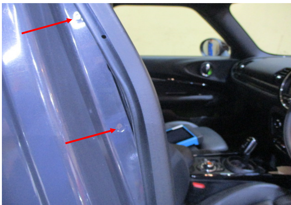
Photo 22 shows the right side "B" pillar of the Motor Car. I did not find any weld marks other than original spot weld marks (arrowed) on the right side "B" pillar of the Motor Car which, indicates that there was no re-welding works carried out. In general, I had found all the non-detachable body panels of the Motor Car to be originally fitted at the time of my inspection.
