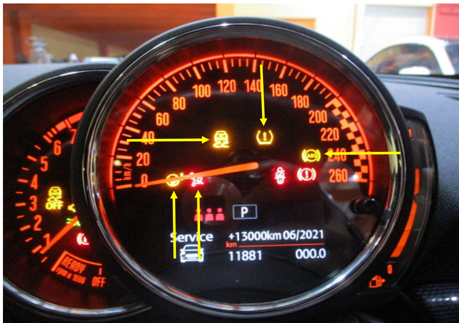
Photo 13 shows the warning lights for the various electronic safety features appearing on the instrument panel of the Motor Car during its self-test when the engine is cranked, in particular the ABS, SRS, PAS, TPM and DSC lights (arrowed).
