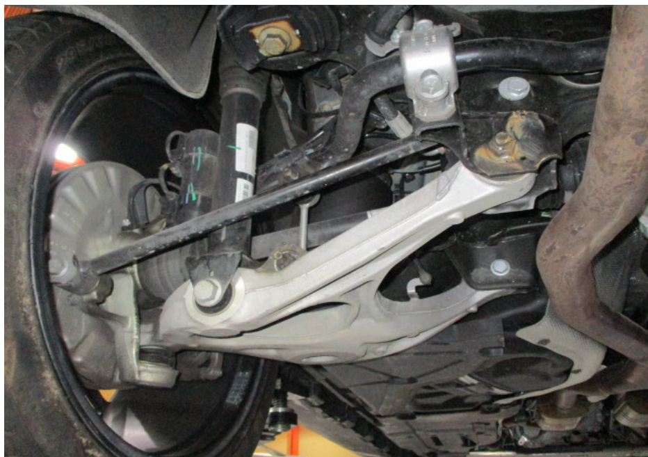
Photo 15 shows a general view of the control arms and linkages at the rear left wheel of the Motor Car. I did not observe any fluid leak and/or fluid stain on the underside of the Motor Car. All of the Motor Car's undercarriage components were observed to be intact and secured in an appropriate manner.
