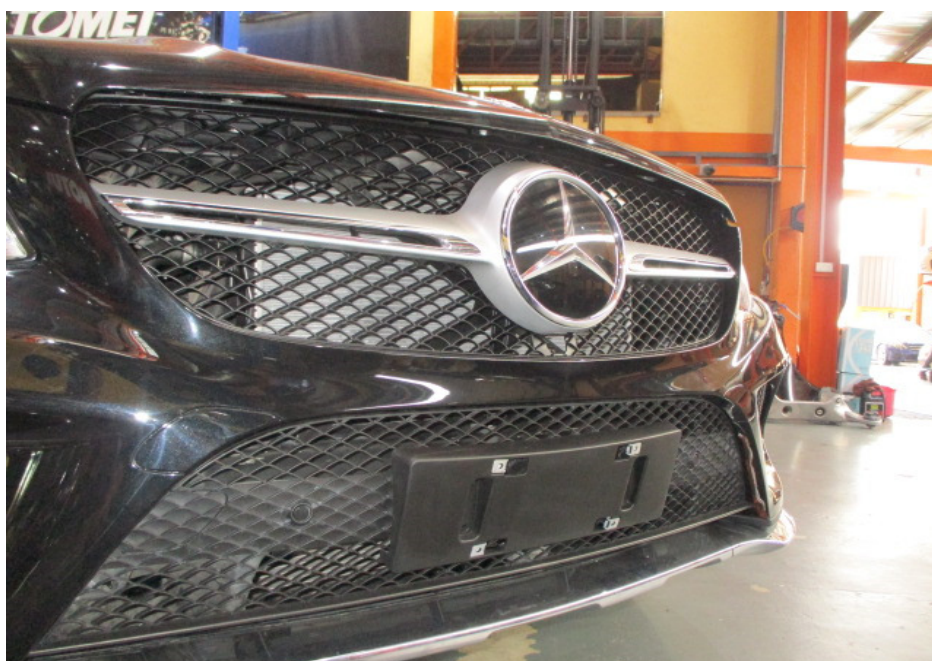
Photo 6 shows a closer view of the front bumper, radiator grille and front bumper centre lower grille of the Motor Car at the time of my inspection. The body parts at the frontal portion of the Motor Car were visually examined and it was observed that the repair/restoration works carried out to the damaged area of the Motor Car (refer to photograph 1 & 2 above) were reasonably adequate and in order.
