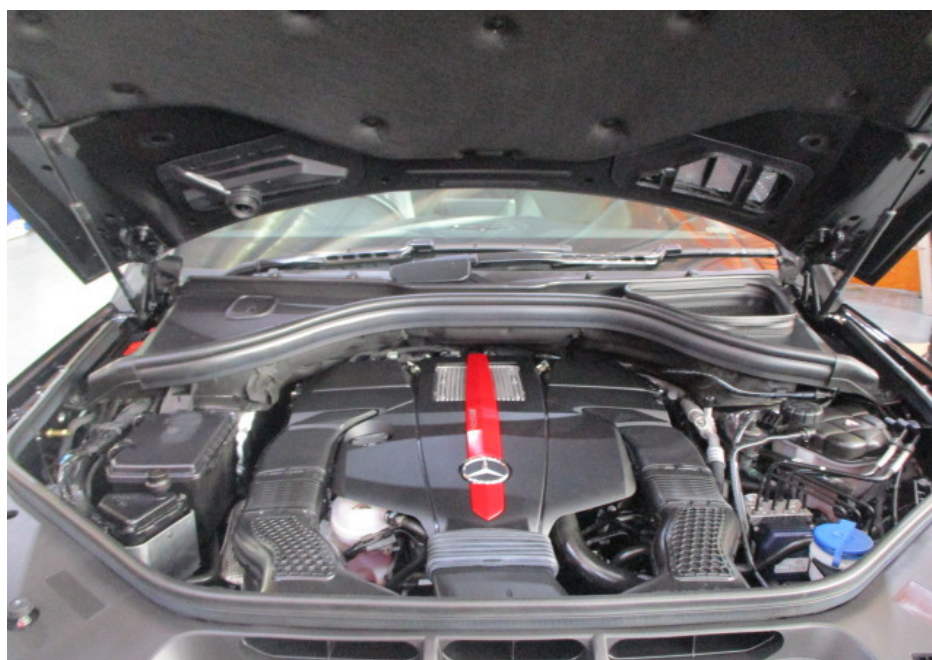
Photo 10 shows a general view of the engine compartment of the Motor Car at the time of my inspection. The various parts and components inside the engine compartment were all observed to be intact and properly fitted. There was also no sign(s) or indication(s) of fluid leak and/or fluid stain found inside the engine compartment.
