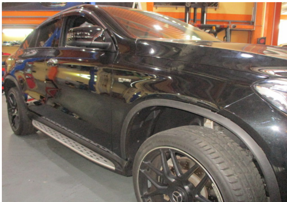
Photo 5 shows a closer view of the front right fender and front right wheel arc garnish of the Motor Car at the time of my inspection. The body parts at the frontal portion of the Motor Car were visually examined and it was observed that the repair/restoration works carried out to the damaged area of the Motor Car (refer to photograph 1 above) were reasonably adequate and in order.
