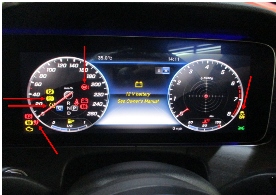
Photo 12 shows the warning lights for the various electronic safety features appearing on the instrument panel of the Motor Car during its self-test when the engine is cranked, in particular the ABS, SRS, EPS, TPM and TCS lights (arrowed).
