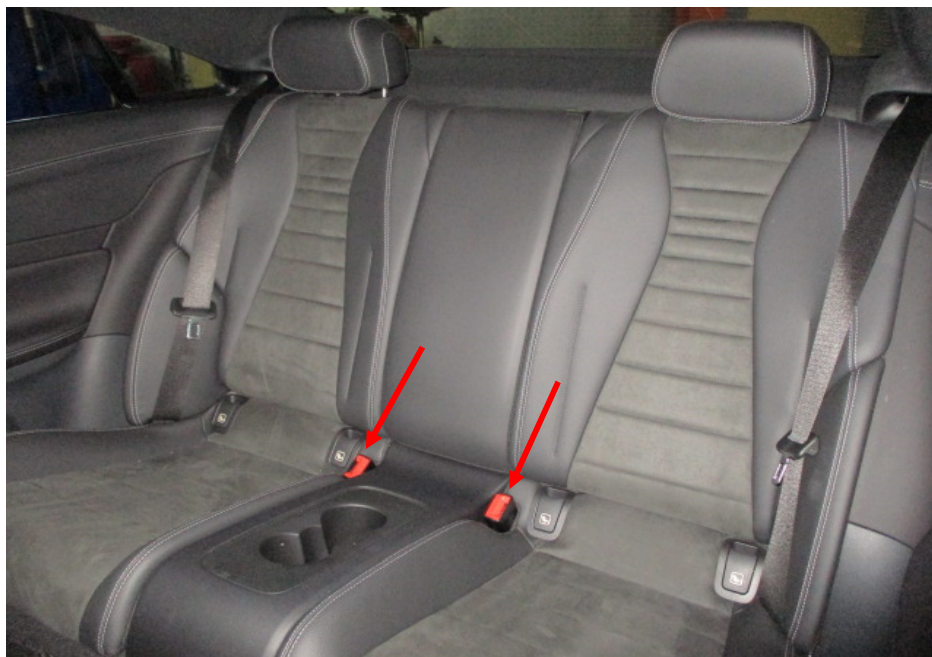
Photo 11 shows the rear seats of the Motor Car. All the seats of the Motor Car were secured via seat rails to the floorboard. They were also fitted with a retractable seat belt reel and a pre-tensioner (arrowed). The seat belts were tested and were able to be fastened into the respective pre-tensions that were fitted on the side of each individual seat.
