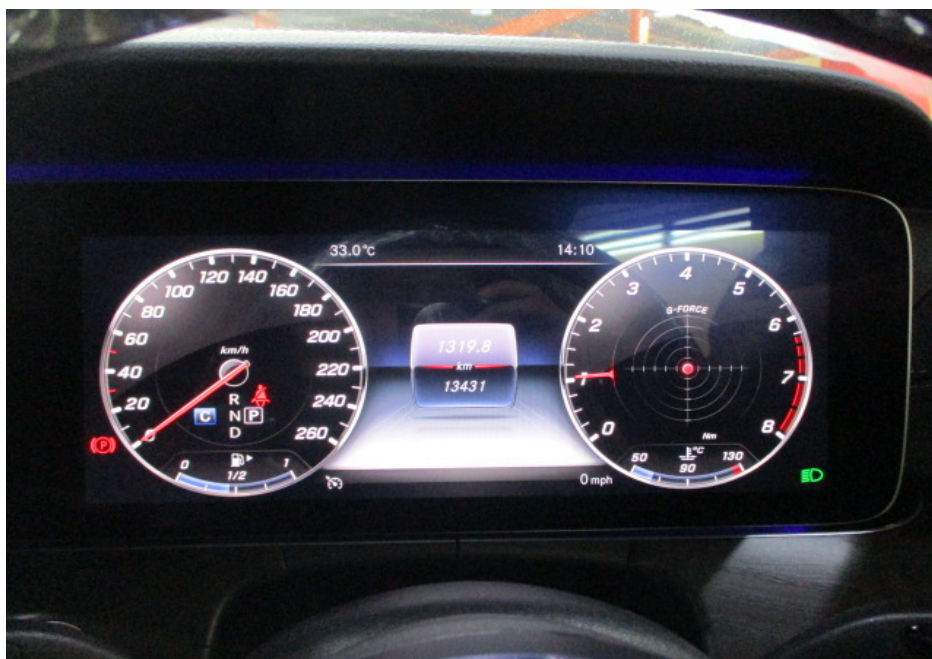
Photo 13 shows the respective warning lights no longer illuminated, indicating that there is no fault detected to the ABS, SRS, EPS, TPM and TCS systems of the Motor Car during the self-test. These electronic systems were hence in working condition at the time of my inspection.
