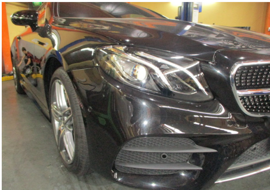
Photo 5 shows a closer view of the front bumper, front bumper right lower grille, front grille, front right headlamp and front bonnet of the Motor Car at the time of my inspection. The body parts at the front right portion of the Motor Car were visually examined and it was observed that the repair/restoration works carried out to the damaged area of the Motor Car (refer to photograph 1 above) were reasonably adequate and in order.
