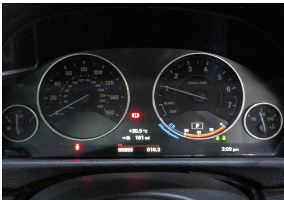
Photo 14 shows the respective warning lights no longer illuminated, indicating that there is no fault detected to the ABS, SRS, IAS, TPM and DSC systems of the Motor Car during the self-test. These electronic systems were hence in working condition at the time of inspection.
