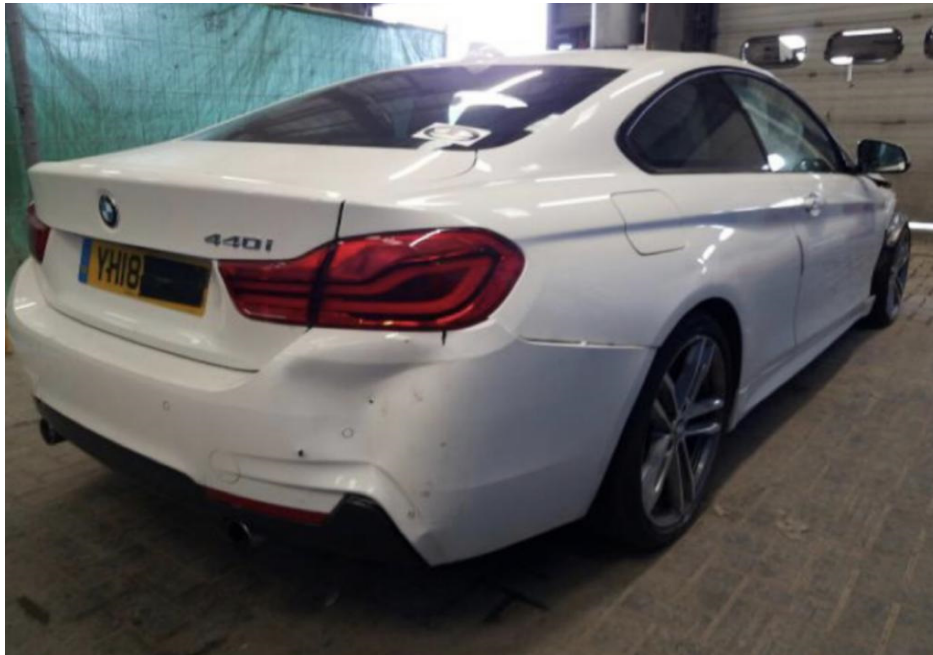
Photo 3 shows the rear right body of the Motor Car (photograph provided to me). Apart for the front right portion, I had also observed damage to the rear right portion of the Motor Car. The rear bumper and rear bumper lower garnish were observed to be damaged.
