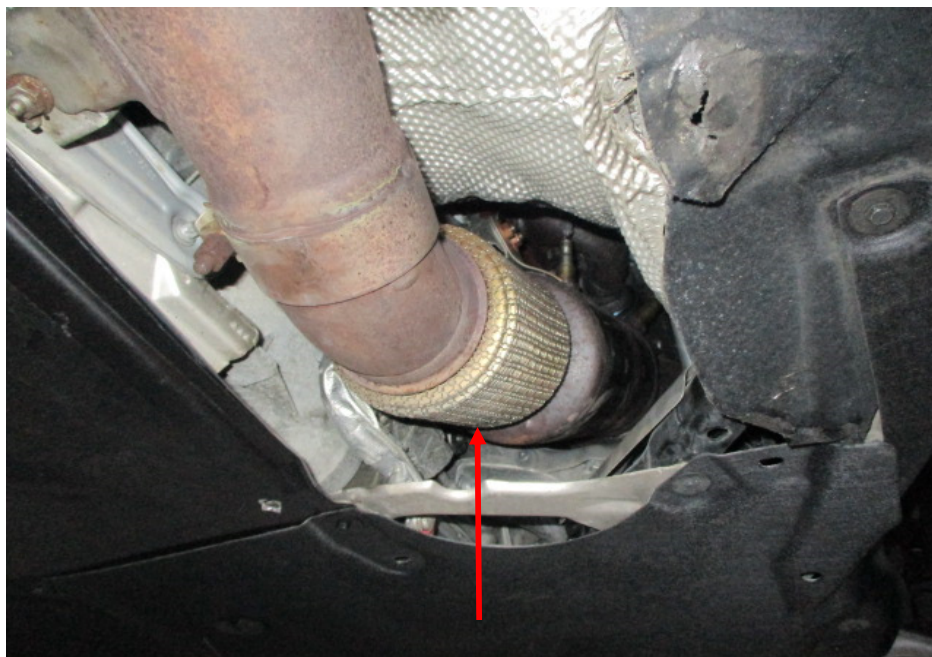
Photo 19 shows the Motor Car's catalytic converter (arrowed). My examination of the Motor Car's exhaust system revealed no sign(s) or indication(s) of any cut or weld marks along its exhaust pipes and on its rear muffler.
