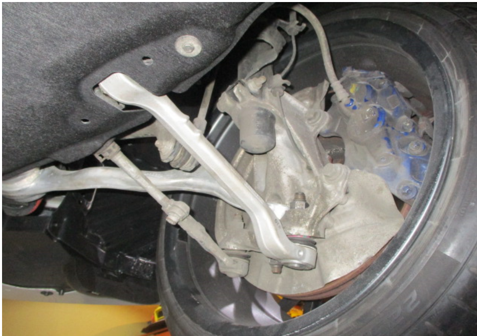
Photo 18 shows the various undercarriage components at the front right wheel of the Motor Car. The mechanical components, control arms and linkages were all found to be intact and secured in an appropriate manner. I also did not observe any fluid leak and/or fluid stain on the underside of the Motor Car.
