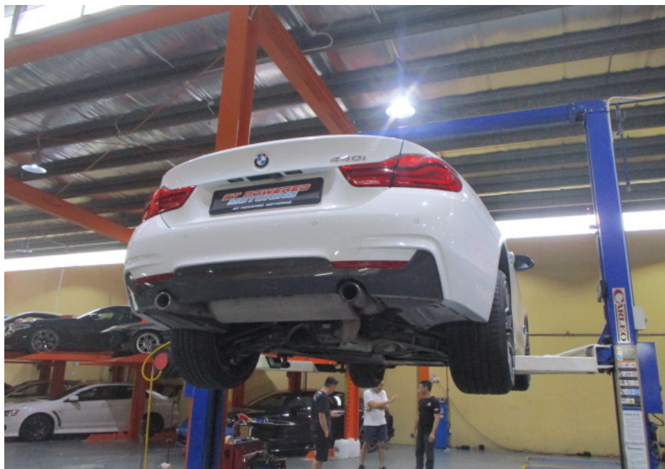
Photo 15 shows the Motor Car hoisted up for checks on its undercarriage. There was no sign(s) or indication(s) of fluid leakage and/or fluid stain(s) on the underside of the Motor Car. The undercarriage components of the Motor Car were also all observed to be intact and secured in an appropriate manner.
