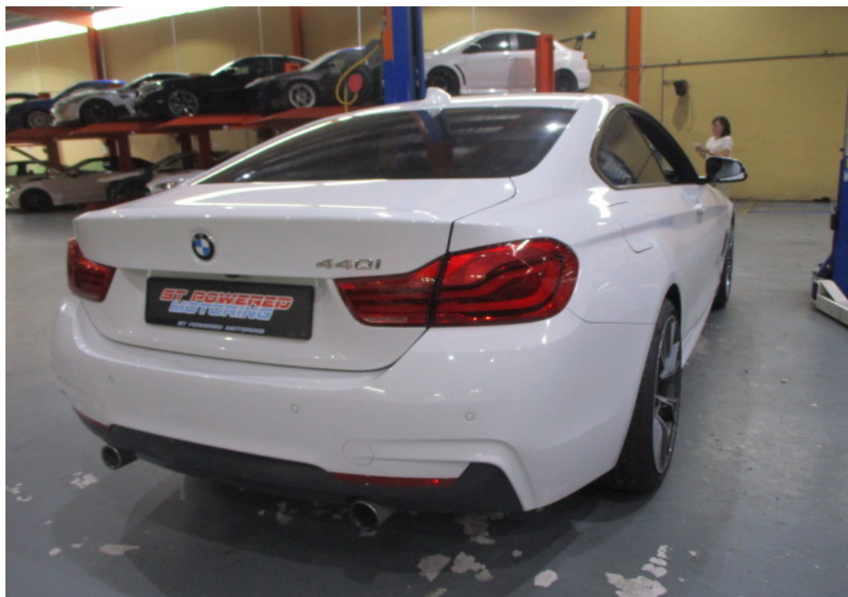
Photo 8 shows a general view of the rear right body of the Motor Car at the time of my inspection. The Motor Car was observed to be in a relatively good general condition with no loose exterior fittings observed. The body parts at the rear right portion of the Motor Car were visually examined and it was observed that the repair/restoration works carried out to the damaged area of the Motor Car (refer to photograph 3 above) were reasonably adequate and in order.
