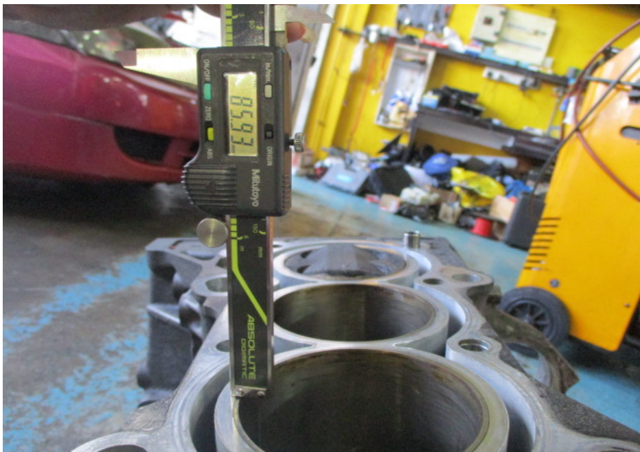
Photo 14 shows the stroke measurement of cylinder 2, which was recorded to be 85.93mm.
