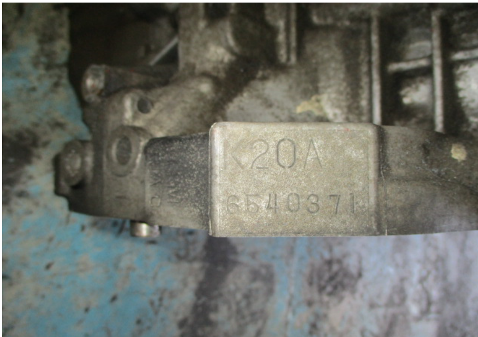
Photo 4 shows the engine number engraved on the housing of the Honda engine that I had inspected. The engine number was K20A6540371.
