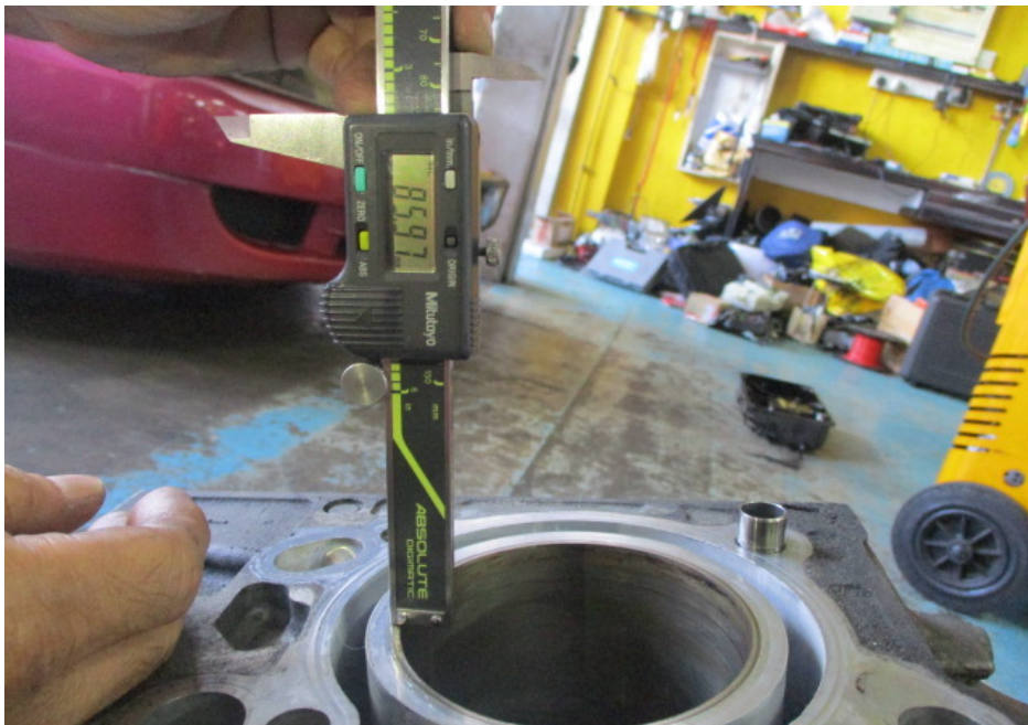
Photo 22 shows the stroke measurement of cylinder 4, which was recorded to be 85.97mm.
