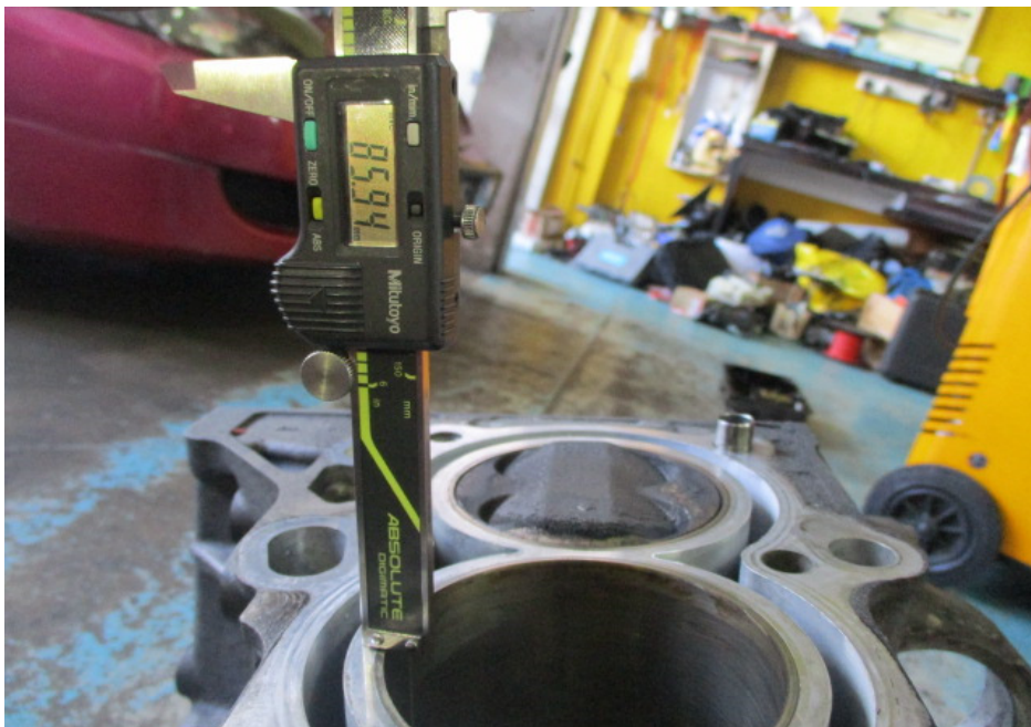
Photo 18 shows the stroke measurement of cylinder 3, which was recorded to be 85.94mm.
