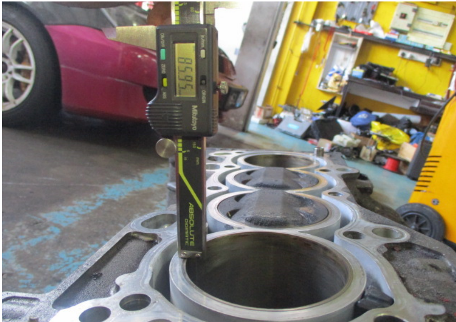
Photo 11 shows the stroke measurement of cylinder 1, which was recorded to be 85.95mm.
