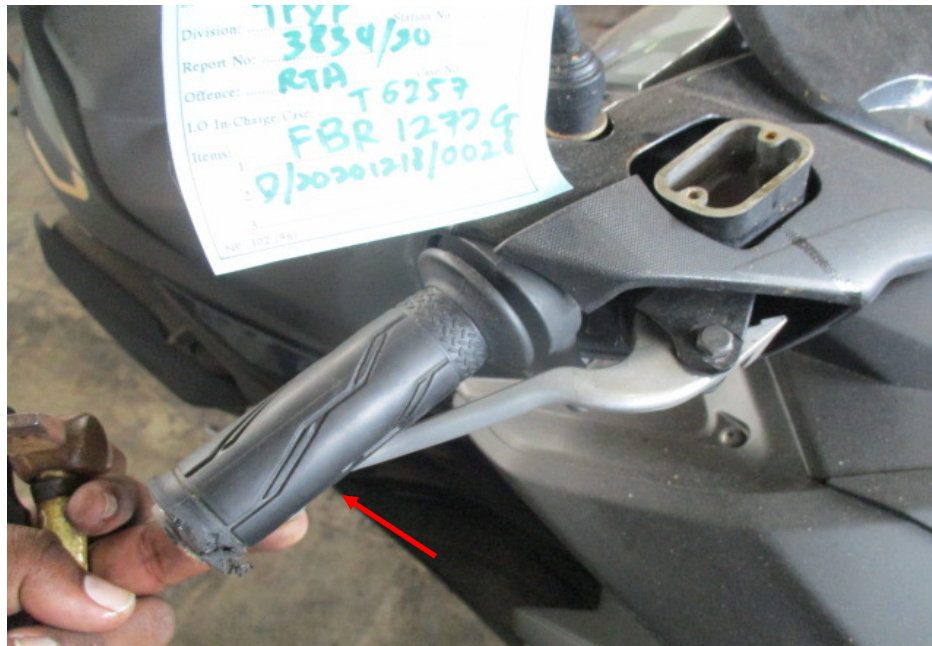
Photo 26 shows the broken right hand brake lever as a result of the accident (arrowed). We were unable to conduct static brake tests on the front braking system of the Motorcycle due to the broken right hand lever. Hence we were unable to indicate if there was any leakage of pressure/vacuum in the front brake system.
