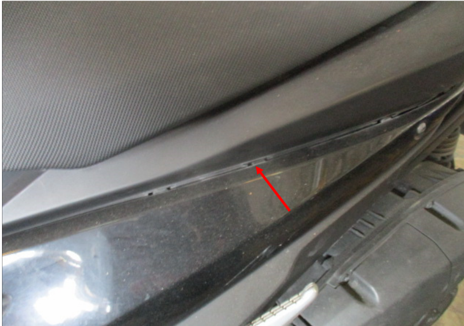
Photo 9 shows a closer view of the deformed left rear side cover (circled) of the Motorcycle at the time of our inspection.
