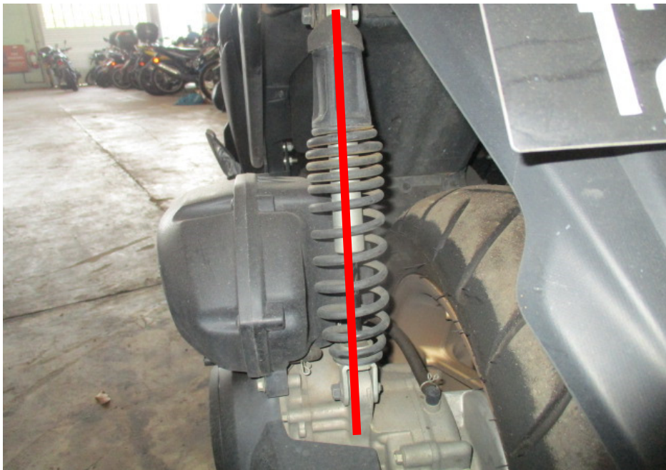
Photo 19 shows the left shock absorber of the Motorcycle which was found to be intact without any misalignment.
