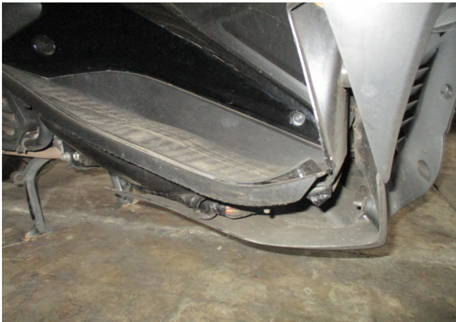
Photo 8 shows a closer view of the cracked right bottom cowling of the Motorcycle as a result of the accident.
