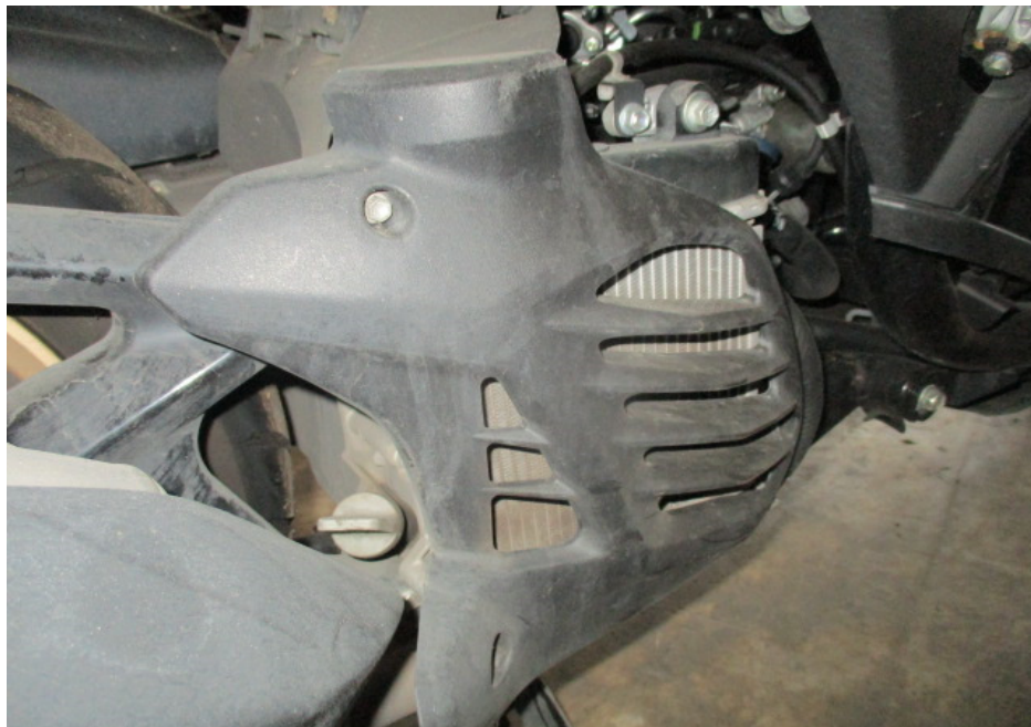
Photo 17 shows the radiator of the Motorcycle at the time of our inspection. The radiator was found to be intact with no visible damage. There was also no sign(s) or indication(s) of fluid leak observed around the radiator of the Motorcycle.
