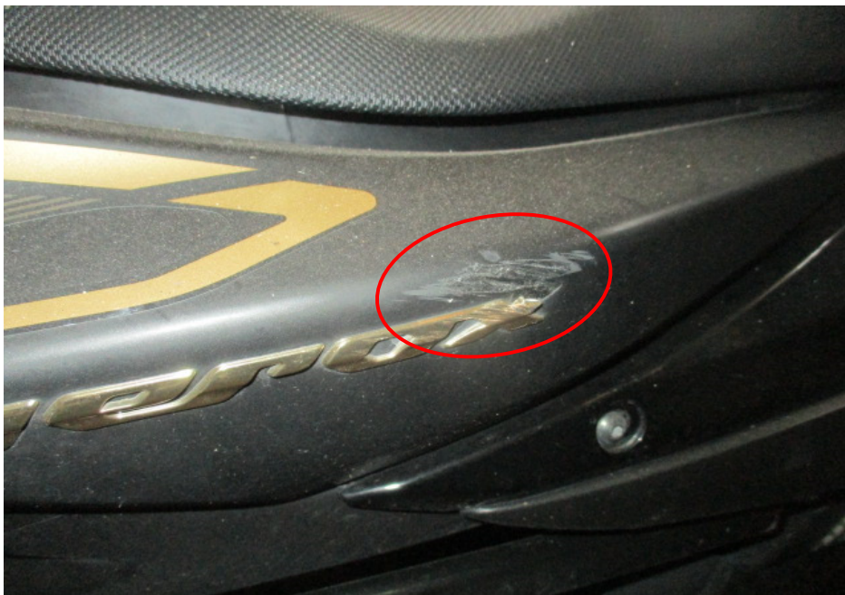
Photo 14 shows a closer view of the grazed right rear side cover (circled) of the Motorcycle at the time of our inspection.
