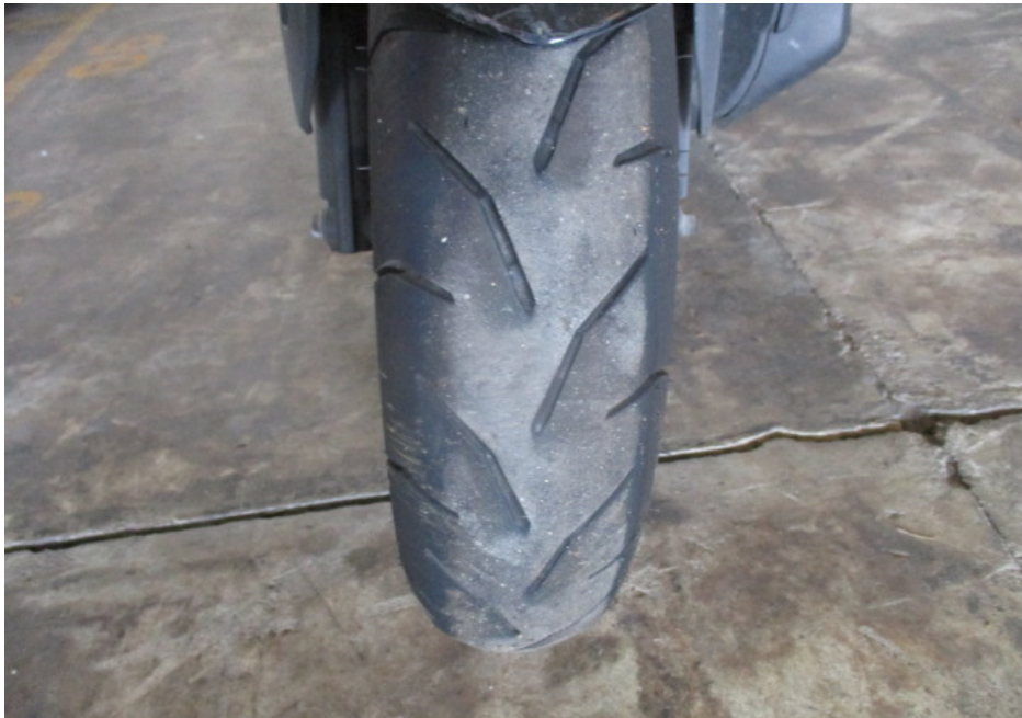
Photo 15 shows the condition of the Motorcycle's front tyre. The front tyre was observed to be in serviceable condition with remaining tread depth of approximately 3mm. There was no tear, burst mark(s) and/or punctured hole(s) on the sidewalls as well as across the tread of the front tyre.
