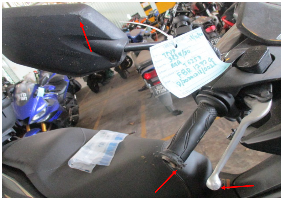
Photo 6 shows a closer view of the front brake lever, right side mirror and right handlebar end of the Motorcycle which were observed to be damaged due to the accident (arrowed).
