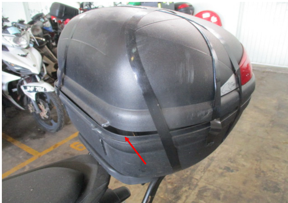
Photo 12 shows the broken top box of the Motorcycle as a result of the accident (arrowed).
