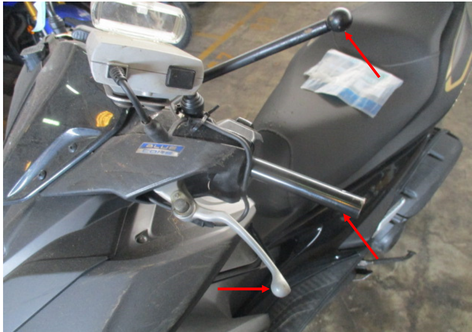
Photo 11 shows a closer view of the rear brake lever, left side mirror and left handlebar grip of the Motorcycle which were observed to be damaged due to the accident (arrowed).
