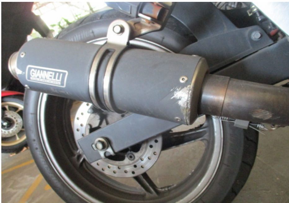
Photo 15 shows a closer view of the exhaust muffler of the Motorcycle that had sustained damages of grazing nature as a result of the accident.
