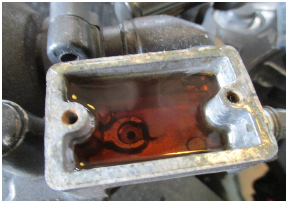
Photo 26 shows the brake fluid reservoir for the front brake of the Motorcycle. The brake fluid was observed to be of sufficient level for operational purposes and without contamination.
