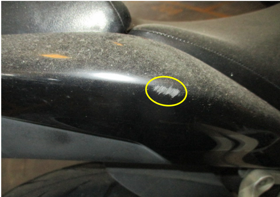
Photo 12 shows the right rear side cover of the Motorcycle that had sustained damages of grazing nature as a result of the accident (circled).
