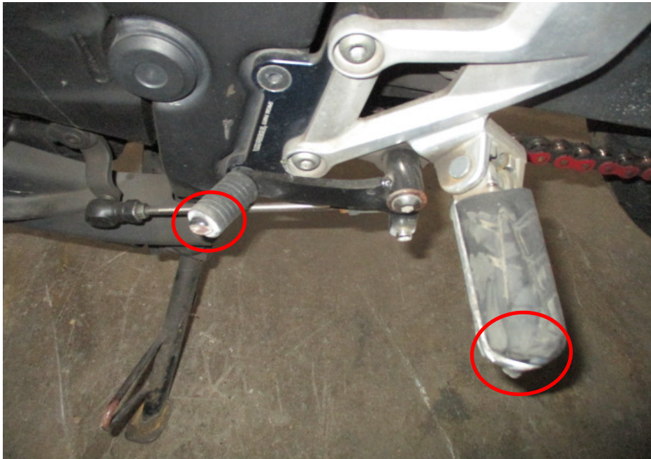
Photo 14 shows a closer view of the gear shift pedal and left front footrest which were amongst the body parts of the Motorcycle that had sustained damage as a result of the accident (circled).
