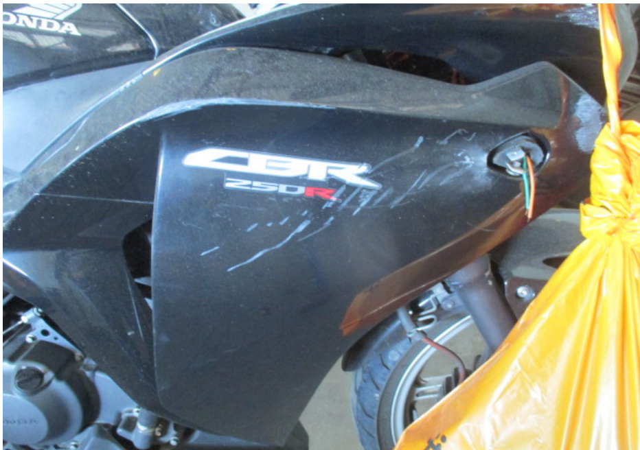
Photo 7 shows a closer view of the right cowl of the Motorcycle that had sustained damages of grazing nature as a result of the accident.
