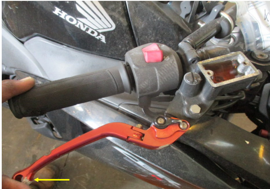
Photo 27 shows the front brake lever being depressed. There was some resistance felt (spongy like feel) upon pressing the front brake lever (arrowed). This would indicate that there is no leakage of pressure/vacuum in the brake system.
