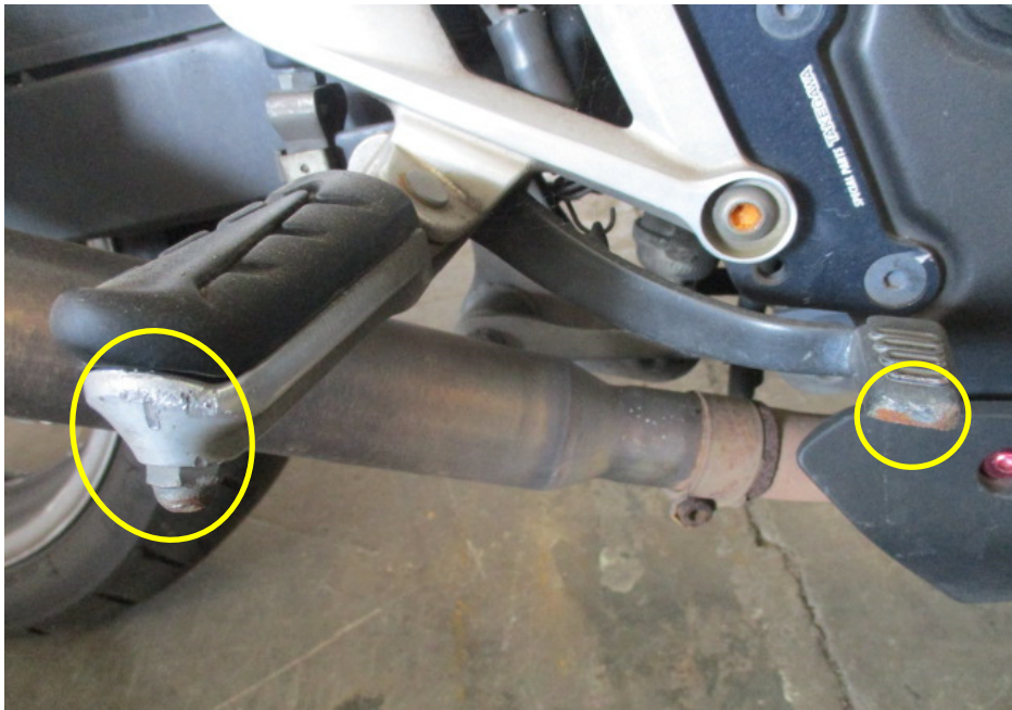
Photo 11 shows a closer view of the rear brake pedal and right front footrest which were amongst the body parts of the Motorcycle that had sustained damage as a result of the accident (circled).
