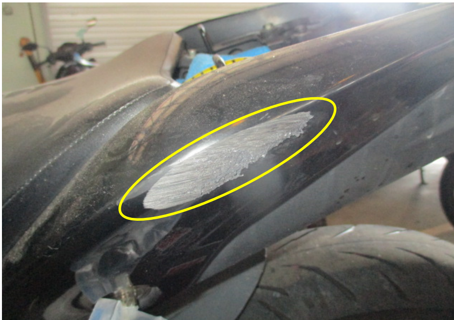
Photo 13 shows the left rear side cover of the Motorcycle that had sustained damages of grazing nature as a result of the accident (circled).
