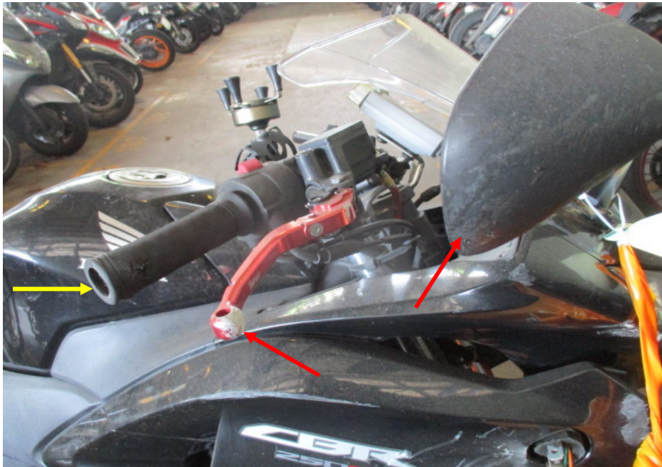
Photo 10 shows a closer view of the missing right handlebar end (yellow arrow), front brake lever and right side mirror (red arrows) which were amongst the body parts of the Motorcycle that had sustained damage as a result of the accident.
