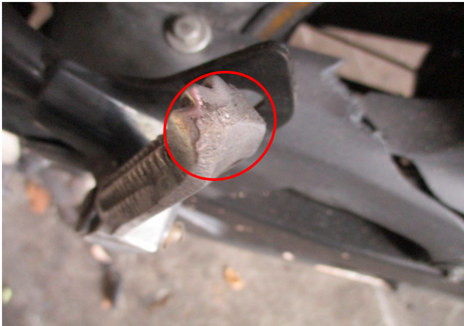
Photo 11 shows a closer view of the left pillion foot peg which was amongst the body parts of the Motorcycle that had sustained damages of grazing nature as a result of the accident (circled).
