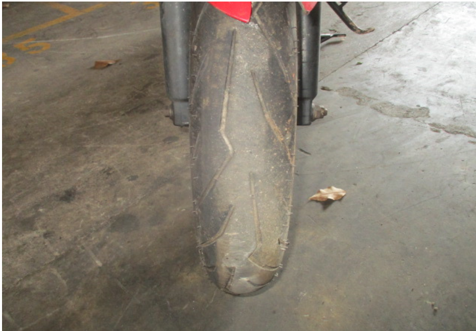
Photo 16 shows the front tyre of the Motorcycle at the time of our inspection. The front tyre was observed to be in serviceable condition with remaining tread depth of approximately 3mm. The pattern of the tread was also clearly visible. There was no tear, burst mark(s) and/or punctured hole(s) on the sidewalls as well as across the tread of the front tyre.
