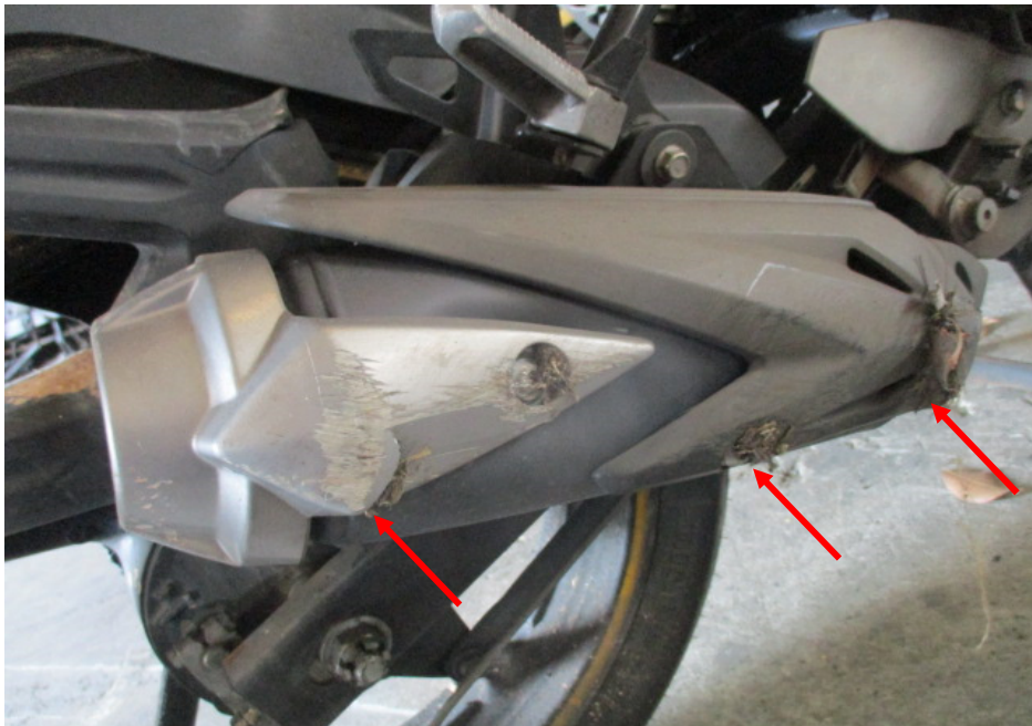
Photo 15 shows a closer view of the exhaust muffler and exhaust muffler heat shield which were amongst the body parts of the Motorcycle that had sustained damages of grazing nature as a result of the accident (circled).
