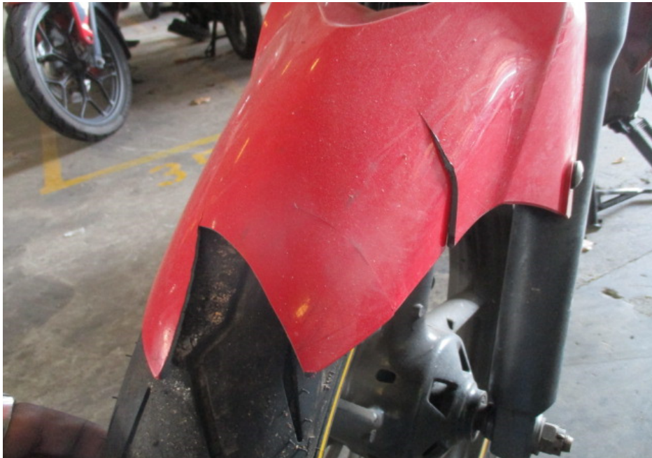
Photo 5 shows a closer view of the cracked front mudguard of the Motorcycle as a result of the accident.
