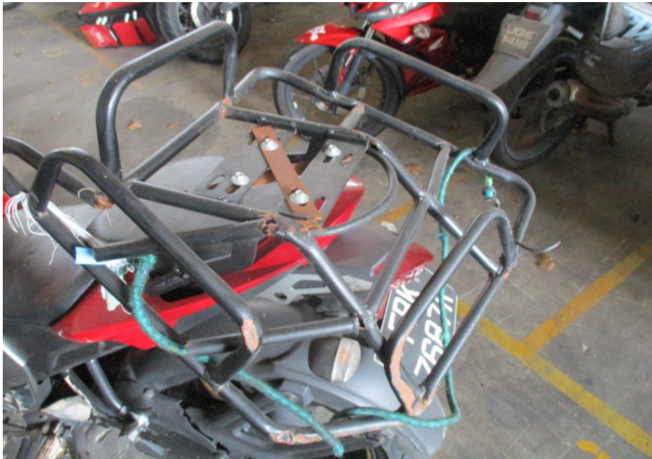
Photo 14 shows the top box rack of the Motorcycle that had sustained extensive damage as a result of the accident.
