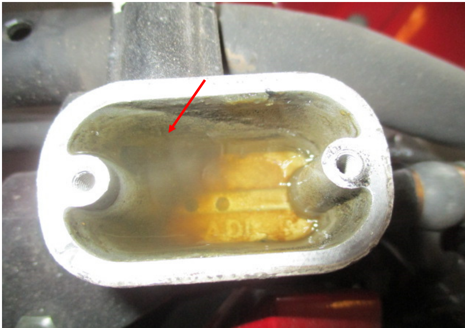
Photo 24 shows the brake fluid reservoir for the front brake of the Motorcycle. The brake fluid was found to be of sufficient level for operating purposes. However the brake fluid was found to be slightly contaminated (arrowed).
