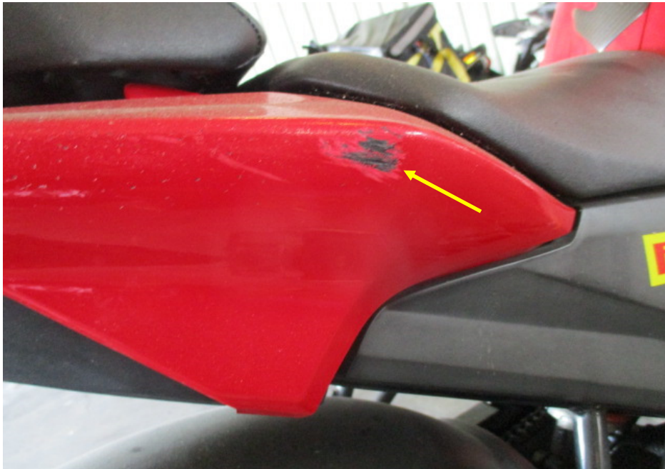
Photo 10 shows a closer view of the right rear side cover which was amongst the body parts of the Motorcycle that had sustained damages of grazing nature as a result of the accident (arrowed).
