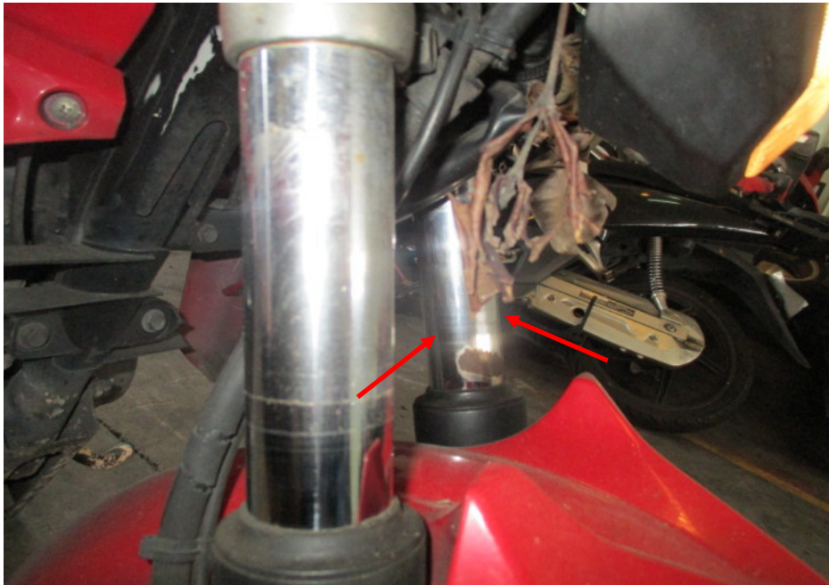
Photo 22 shows the front forks of the Motorcycle. The left front fork was found to be bent inwards as a result of the accident (arrowed).
