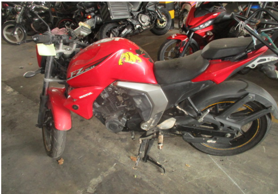
Photo 3 shows a general view of the left body of the Motorcycle at the time of our inspection. The Motorcycle was observed to have sustained damages all around. Amongst the body parts that were found to have been damaged include its windshield, front mudguard, left cowling, clutch lever, side mirrors, handlebar, fuel tank, left pillion foot peg, rear side covers, right front footrest, exhaust muffler, exhaust muffler heat shield, top box rack and rear mudguard, amongst others.
