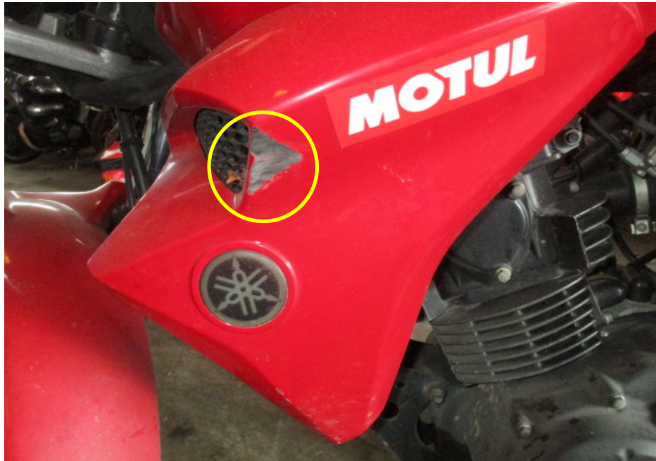
Photo 6 shows a closer view of the left cowling which was amongst the body parts of the Motorcycle that had sustained damage as a result of the accident (circled).
