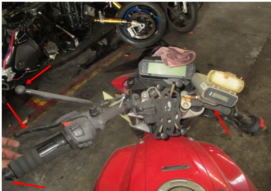
Photo 7 shows the clutch lever, left handlebar end, side mirrors and handlebar (arrowed), which were amongst the body parts of the Motorcycle that had sustained damage as a result of the accident.
