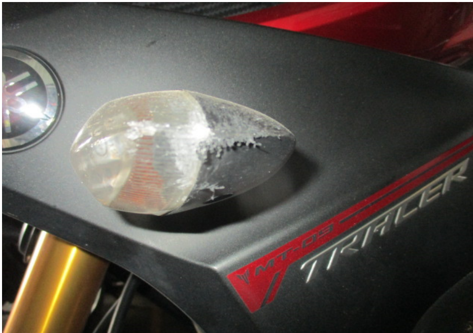
Photo 7 shows a closer view of the left front signal lamp of the Motorcycle that had sustained damages of grazing nature as a result of the accident.
