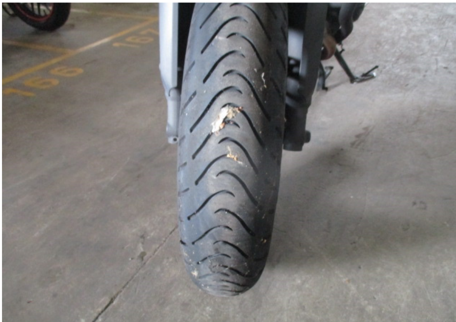
Photo 13 shows the condition of the Motorcycle's front tyre. The front tyre was observed to be in serviceable condition with remaining tread depth of approximately 4mm. There was no tear, burst mark(s) and/or punctured hole(s) on the sidewalls as well as across the tread of the front tyre.
