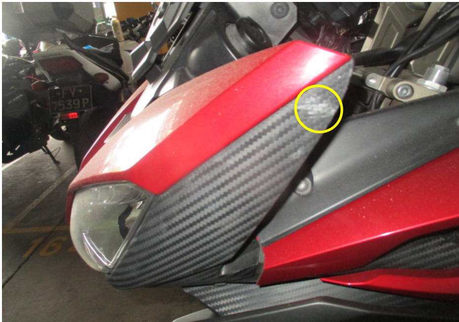
Photo 5 shows a close up view of the head cowlings was amongst the body parts of the Motorcycle that had sustained damage as a result of the accident (circled).
