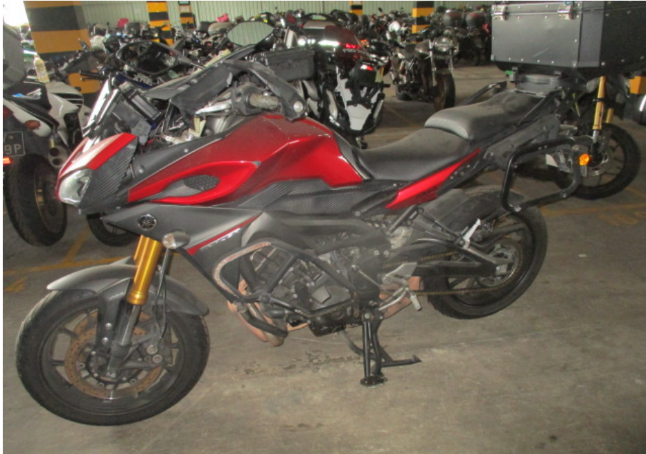
Photo 4 shows a general view of the left body of the Motorcycle at the time of our inspection. The Motorcycle was observed to have sustained damages all around. The body parts that were found to have been damaged include its head cowlings, side cowlings, front signal lamps, left tank cover, clutch lever guard, clutch lever, left side mirror, gear shift pedal, left front footrest, left engine crashbar and top box, amongst others.
