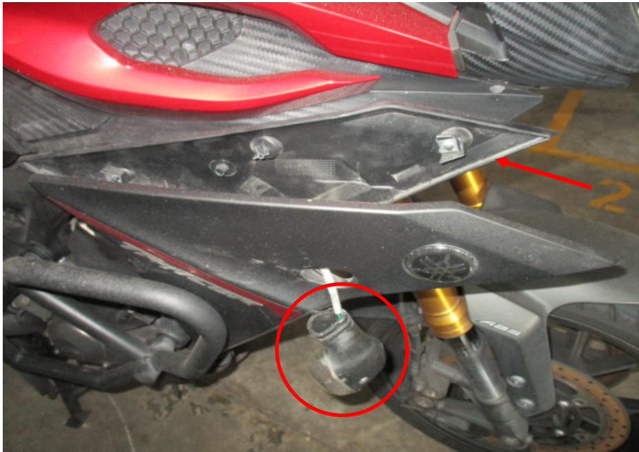
Photo 12 shows a closer view of the dislodged right cowling and right front signal lamp of the Motorcycle as a result of the accident (arrowed) (circled).
