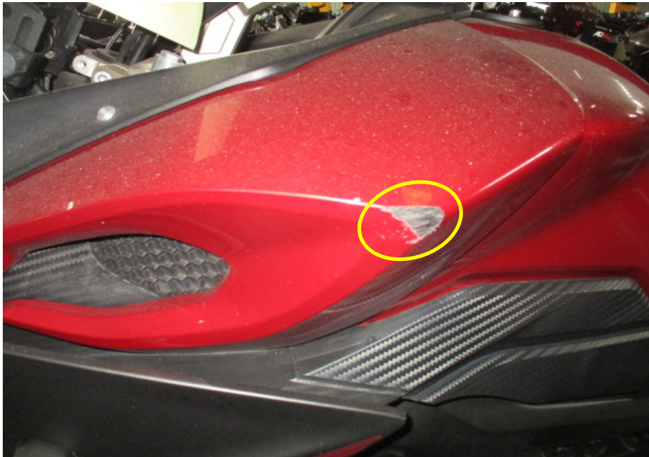
Photo 6 shows a closer view of the left tank cover which was amongst the body parts at the front body of the Motorcycle that had sustained damage as a result of the accident (circled).
