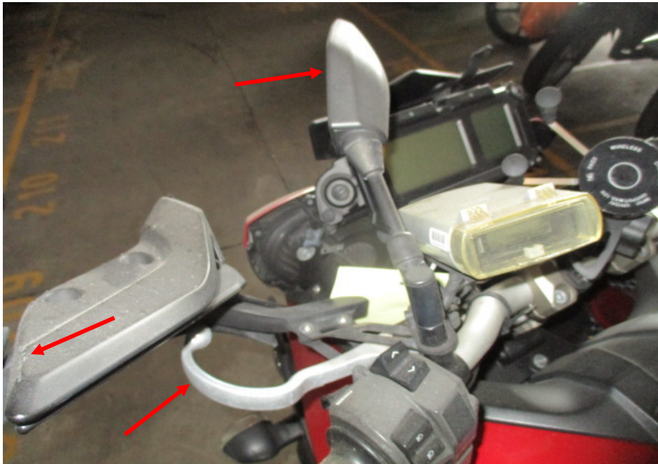
Photo 8 shows a closer view of the clutch lever guard, clutch lever and left side mirror (arrowed) which were amongst the body parts of the Motorcycle that had sustained damage as a result of the accident.
