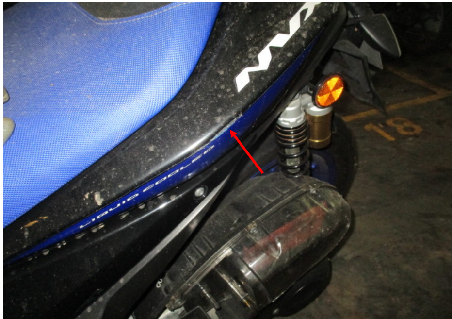
Photo 13 show a closer view of the left rear side cover of the Motorcycle which was observed to be damaged due to the accident (arrowed).
