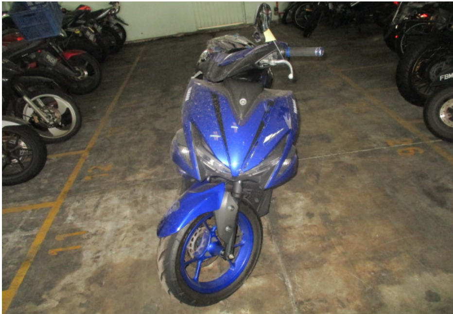
Photo 22 shows the front wheel of the Motorcycle turned towards its full right. Turning the Motorcycle's handle bar towards the left and right did not produce any abnormal free play and/or resistance. This would indicate that the steering system of the Motorcycle was in serviceable condition at the time of our inspection.
