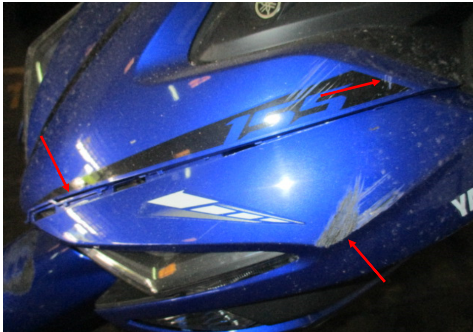
Photo 6 shows a closer view of the front cowling of the Motorcycle which was observed to be damaged due to the accident (arrowed).
