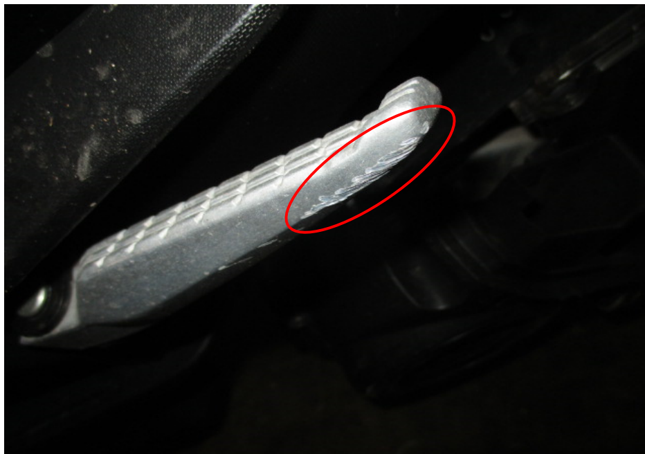
Photo 14 shows a closer view of the grazed left pillion foot peg (circled) of the Motorcycle at the time of our inspection.
