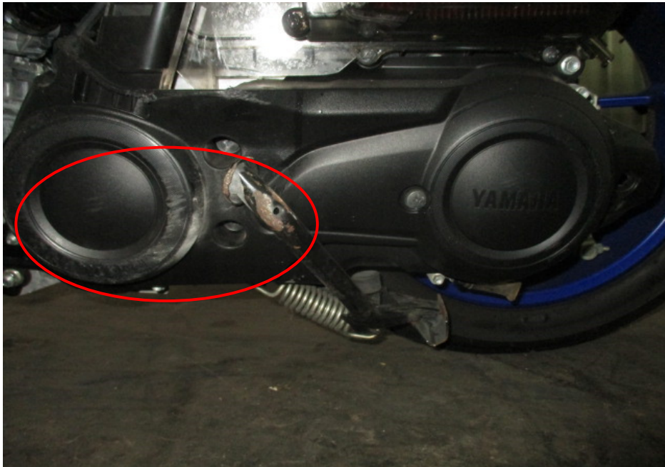
Photo 18 shows the drive train cover of the Motorcycle which had sustained damages of grazing nature as a result of the accident (circled) however the engine components were still intact.
