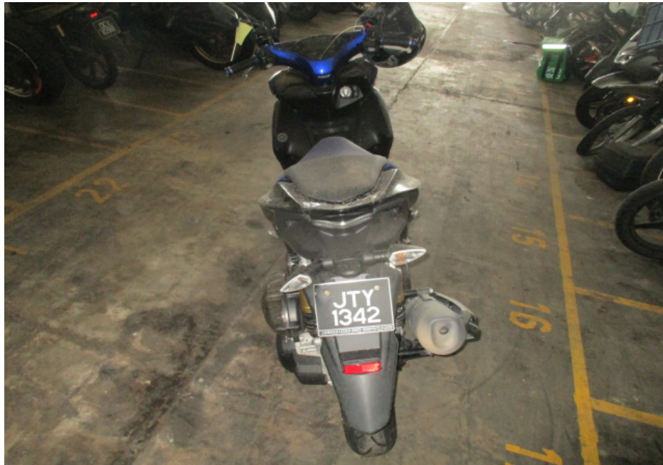
Photo 1 shows a general view of the rear portion of the Motorcycle at the time of our inspection. The Motorcycle was observed to have sustained damages all around. The mileage of the Motorcycle could not be recorded at the time of our inspection despite several attempts to jump start the battery
