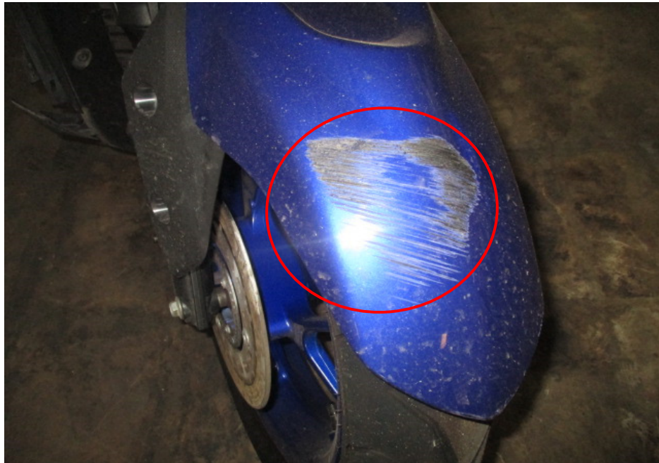
Photo 5 shows a closer view of the front mudguard (circled) which was amongst the body parts at the front body of the Motorcycle that had sustained damage as a result of the accident.
