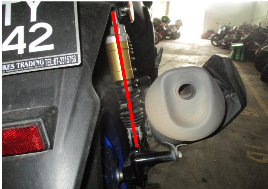
Photo 20 shows the right shock absorber of the Motorcycle which was found to be intact without any misalignment.
