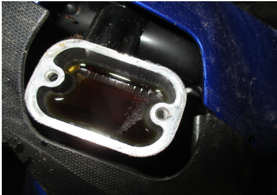
Photo 25 shows a close up view of the brake fluid reservoir for the front brake of the Motorcycle. The brake fluid was observed to be of sufficient level and without contamination for operational purposes.
