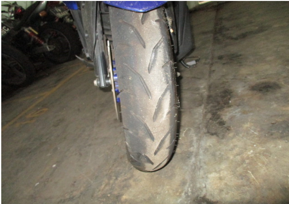
Photo 15 shows the condition of the Motorcycle's front tyre. The front tyre was observed to be in serviceable condition with remaining tread depth of approximately 4mm. There was no tear, burst mark(s) and/or punctured hole(s) on the sidewalls as well as across the tread of the front tyre.
