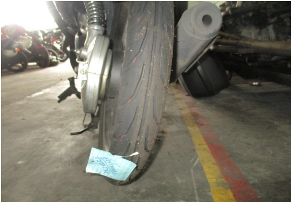
Photo 15 shows the condition of the Motorcycle's rear tyre. The rear tyre was observed to be in serviceable condition with remaining tread depth of approximately 4mm. The tyre was also observed to be sufficiently inflated for vehicular operation. We did not observe any tear, burst mark(s) and/or punctured hole(s) on the sidewalls as well as across the tread of the rear tyre.
