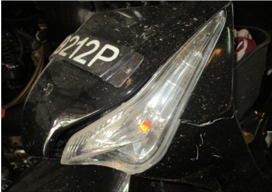
Photo 4 shows a close up view of the headlight assembly which was amongst the body parts at the front of the Motorcycle that had sustained damage as a result of the accident.
