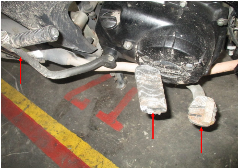
Photo 12 shows the bent rear brake pedal, kickstarter pedal and right front footrest of the Motorcycle as a result of the accident (arrowed).
