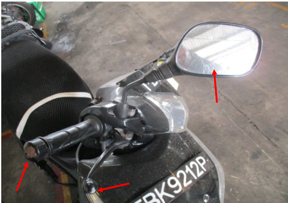
Photo 9 shows the right handlebar end, right side mirror and front brake lever (arrowed), which were amongst the body parts of the Motorcycle that had sustained damage as a result of the accident.
