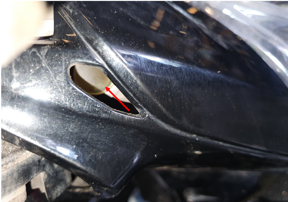
Photo 24 shows the brake fluid reservoir for the front brake of the Motorcycle. The brake fluid was found to be without contamination and of sufficient level for operating purposes (arrowed).
