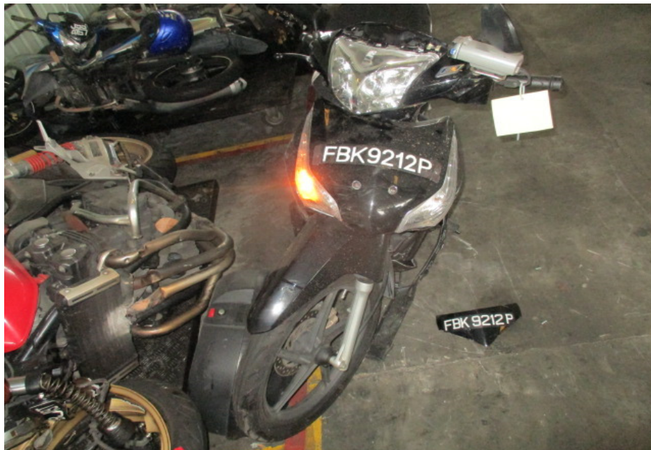
Photo 22 shows the front wheel of the Motorcycle turned towards its full right. Turning the Motorcycle's handle bar towards the right did not produce any abnormal free play and/or resistance. This would indicate that the steering system of the Motorcycle was in serviceable condition at the time of our inspection.
