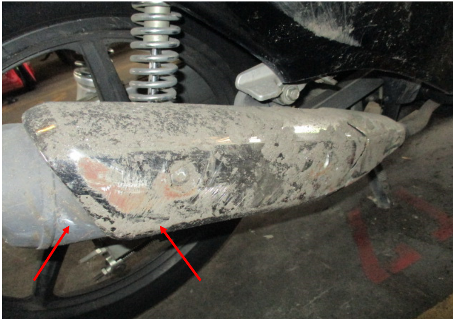
Photo 10 shows a closer view of the exhaust muffler and exhaust muffler heat shield which was amongst the body parts of the Motorcycle that had sustained damages of grazing nature as a result of the accident (arrowed).
