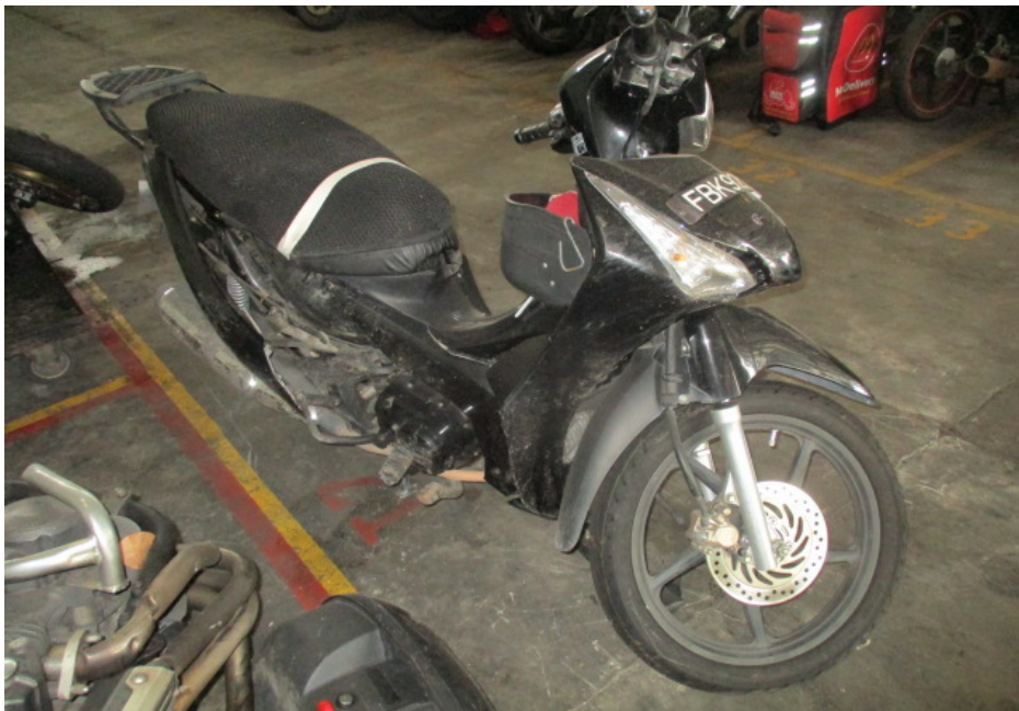
Photo 3 shows a general view of the right body of the Motorcycle at the time of our inspection. The Motorcycle was observed to have sustained damages all around. The body parts that were found to have been damaged include its headlight assembly, front mudguard, front cowling, side cowlings, right side mirror, right handlebar end, front brake lever, rear brake pedal, right front footrest, kickstarter pedal, exhaust muffler, exhaust muffler heat shield, right rear side cover and top box rack, amongst others.
