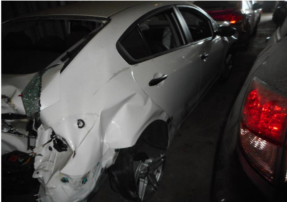
Photo 9 shows the general view of the Motor Car's right body at the time of my inspection. The Motor car was observed to have sustained damage at its right portion. Its right body panel was damaged as a result of the accident.
