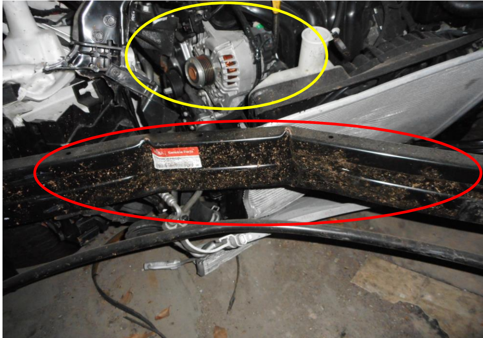
Photo 7 shows the close up view of the Motor Car's front body at the time of my inspection. The Motor car was observed to have sustained damage at its front portion. Its alternator (yellow circle) and body reinforcement panel (red circle) was amongst the various components in the engine compartments were also damaged as a result of the accident.
