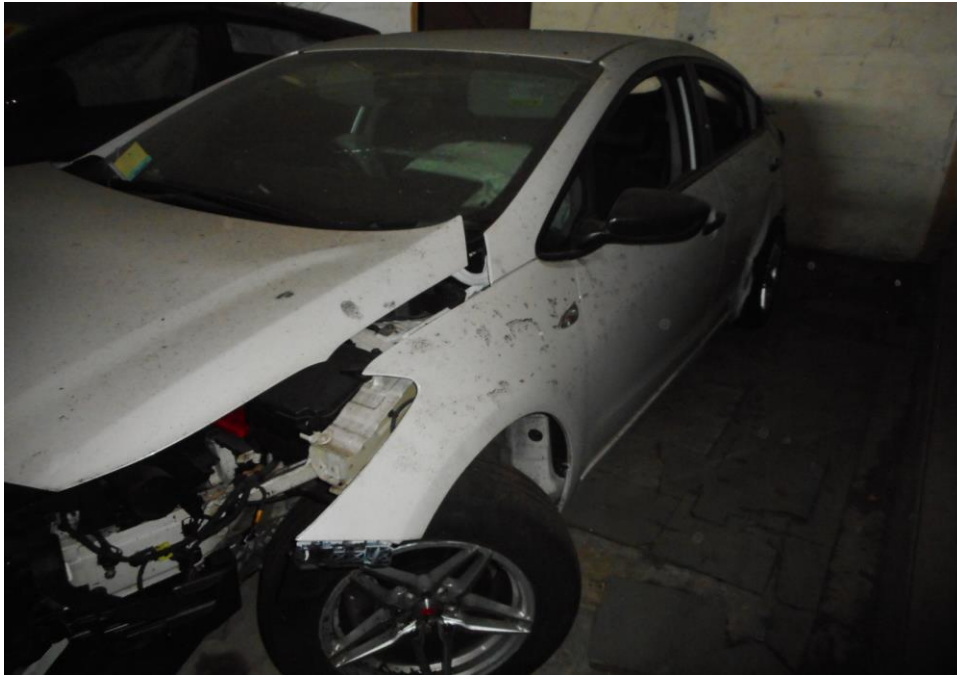
Photo 11 shows the general view of the Motor Car's left body at the time of my inspection. The Motor car was observed to have sustained damage at its left portion. Its left body panel was damaged as a result of the accident.
