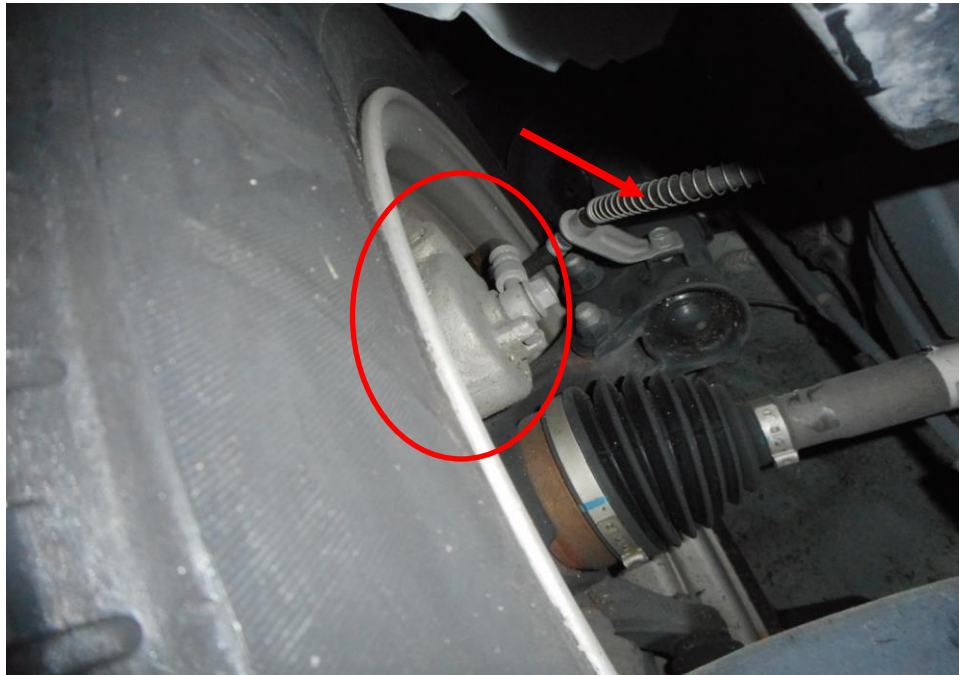
Photo 21 shows the brake hose/pipe (arrowed) at the front right wheel of the Motor Car. No leakage of brake fluid was observed. Visual examination of the various components of the braking system like the brake caliper (circled) brake pedal etc had revealed all to be intact and without visible damage at the time of accident. There was also no sign of fluid stain(s) observed on the various undercarriage components.
