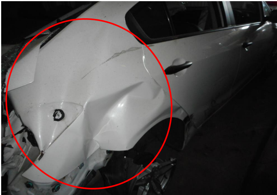
Photo 10 shows the close up view of the Motor Car's right body at the time of my inspection. The Motor car was observed to have sustained damage at its right portion. Its right body panel (circled) was damaged as a result of the accident.
