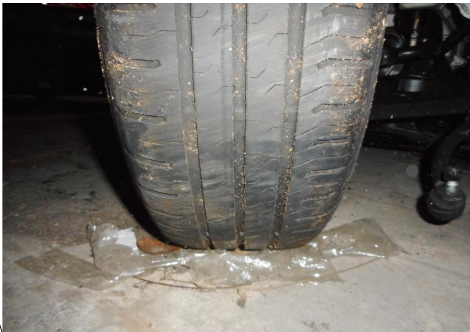
Photo 16 shows the condition of the front left tyre of the Motor Car, which was observed to be in serviceable condition with remaining tread depth of approximately 4.7mm. The tyre was also observed to be sufficiently inflated for vehicular operation with no tear, cut or burst mark(s).
