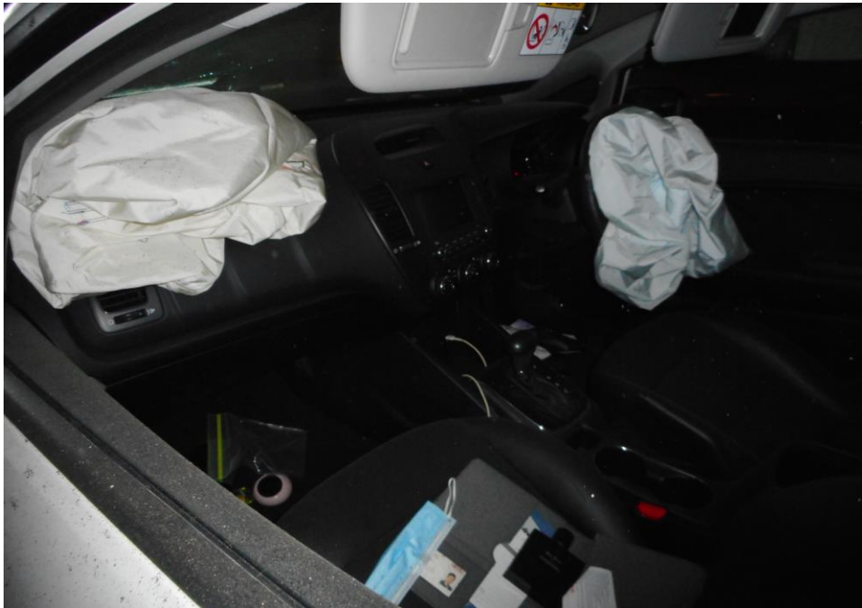
Photo 17 shows the deployment of the Supplemental Restraint System (SRS) airbag in the Motor Car as a result of the accident.
