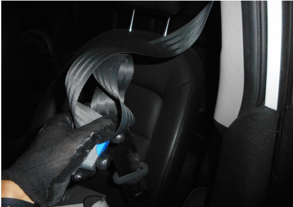
Photo 26 shows that that the seat belt on the left seat was worn at the material time of accident as the safety pre-tensioners was activated at the moment of impact and caused the seat belt to be locked into the last position.
