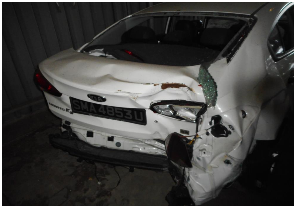
Photo 2 shows a general view of the Motor Car's rear body at the time of my inspection. Its rear windscreen and rear bonnet (red circle), rear bumper (yellow circle) and its rear right brake lamp (arrowed) was amongst the body parts that were also damaged as a result of the accident.
