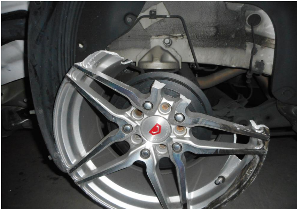
Photo 14 shows the condition of the rear right tyre and rim of the Motor Car, the wheel rim was observed to be broken off as a result of the accident
