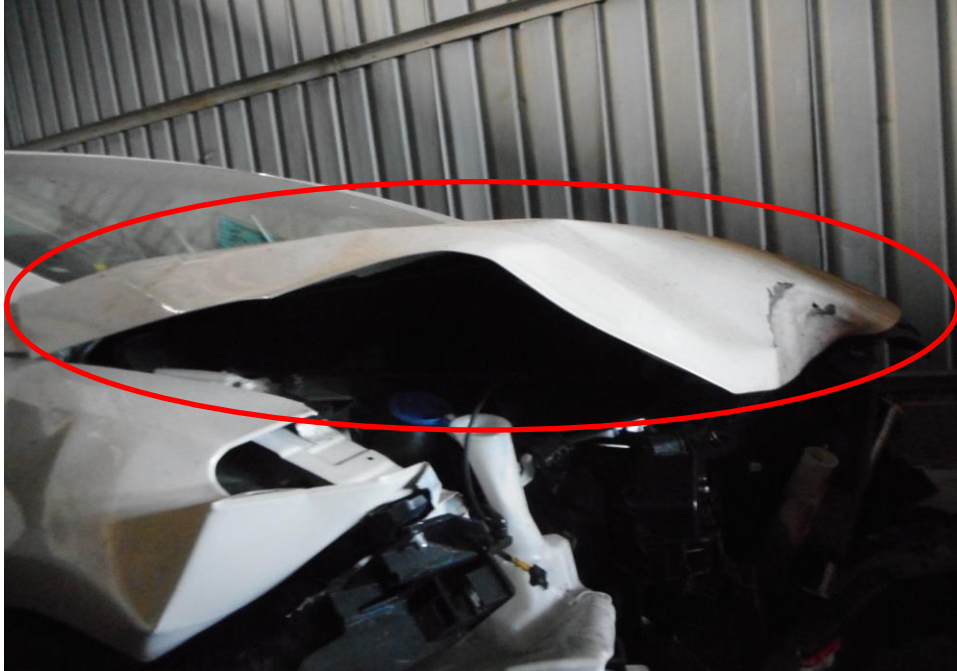
Photo 18 shows a close up view of the damaged front bonnet lock mechanism and the structure of the engine compartment of the Motor Car at the time of my inspection resulting it unable to open a result of the accident (circled) (Unable to open)
