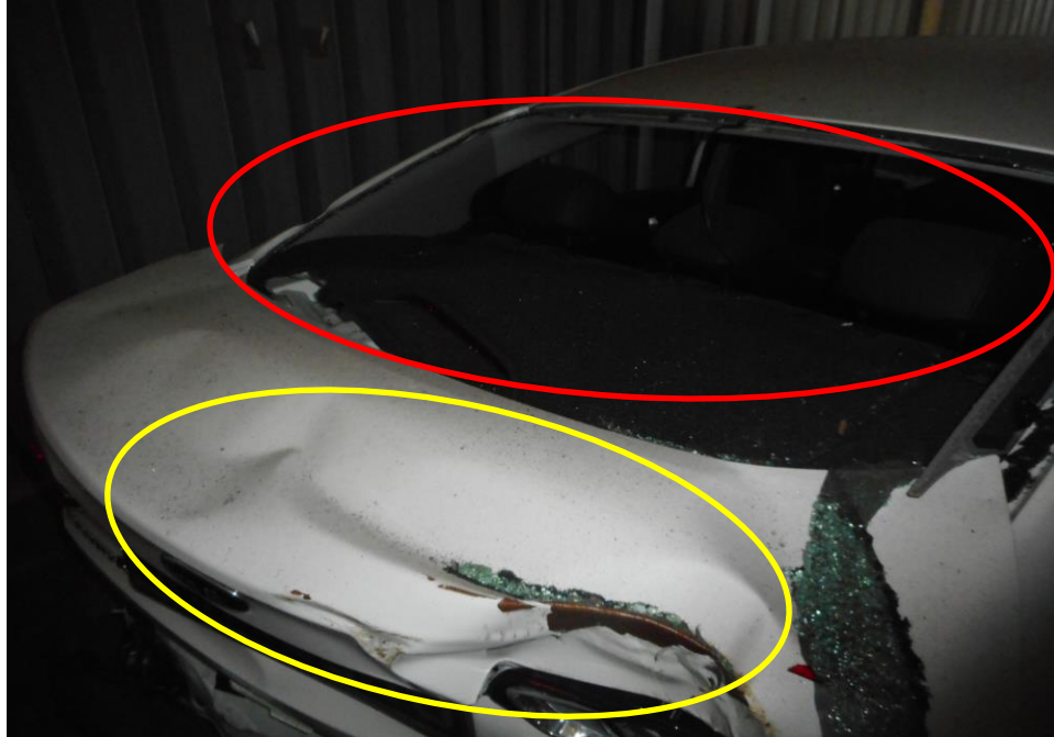
Photo 3 shows a close up view of the Motor Car's rear body at the time of my inspection. Its rear windscreen (red circle) and rear bonnet (yellow circle) was amongst the body parts that were also damaged as a result of the accident.
