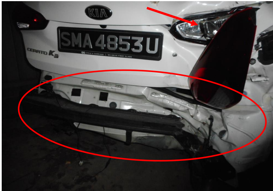
Photo 4 shows a close up view of the Motor Car's rear body at the time of my inspection. Its rear bumper (circled) and its rear right brake lamp (arrowed) was amongst the body parts that were also damaged as a result of the accident.
