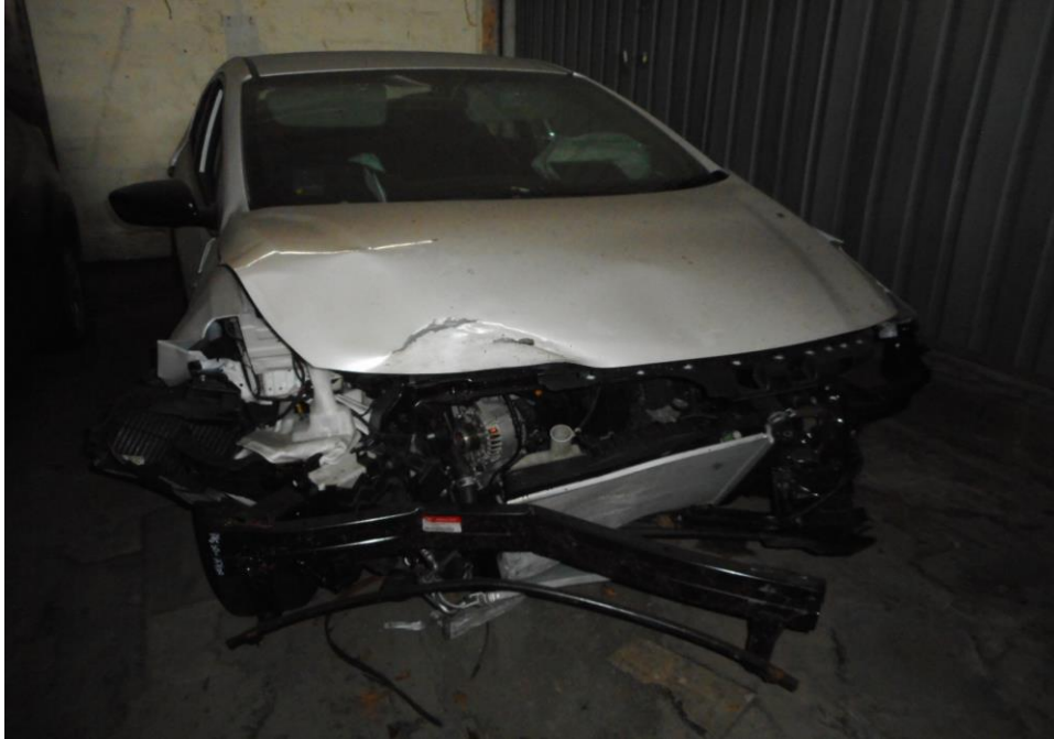
Photo 5 shows a general view of the Motor Car's front body at the time of my inspection. Its front bonnet and front bumper was amongst the body parts and various components in the engine compartments were also damaged as a result of the accident. The Supplemental Restraint System (SRS) was activated as a result of the accident.
