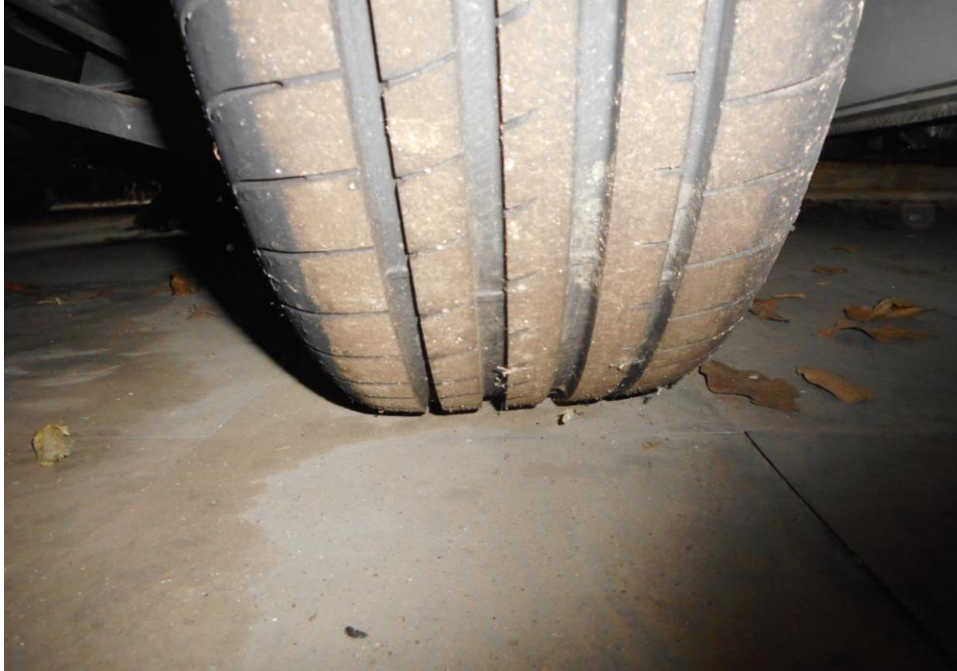
Photo 13 shows the condition of the front right tyre of the Motor Car, which was observed to be in serviceable condition with remaining tread depth of approximately 5.1mm. The tyre was also observed to be sufficiently inflated for vehicular operation with no tear, cut or burst mark(s).
