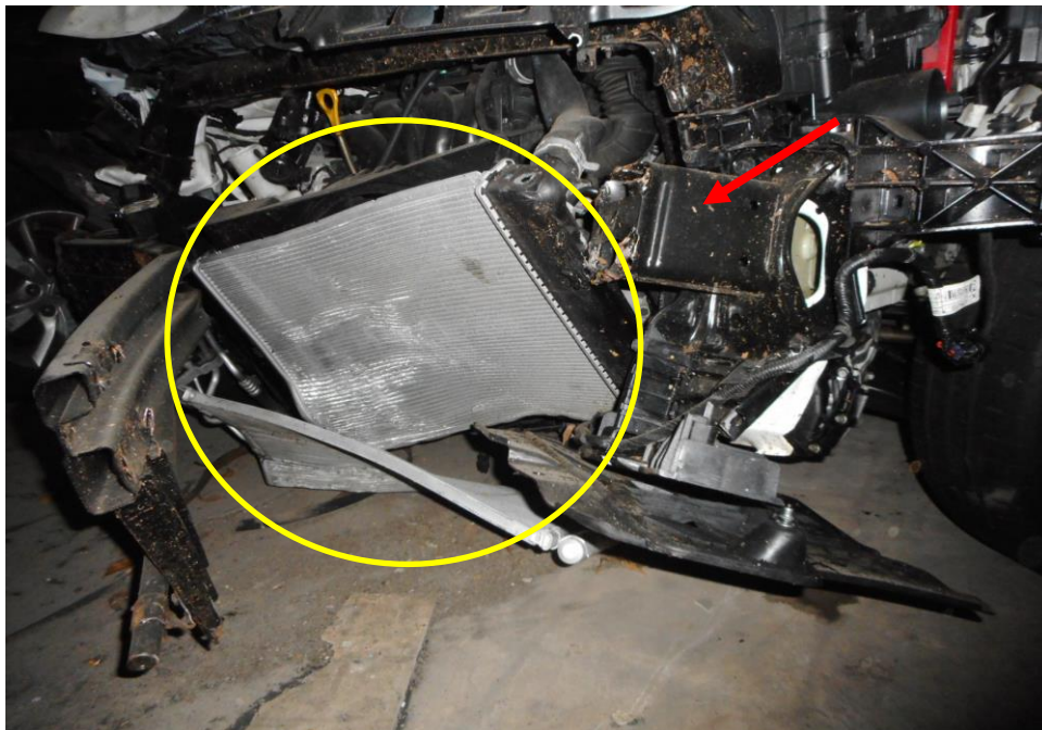
Photo 8 shows the close up view of the Motor Car's front body at the time of my inspection. The Motor car was observed to have sustained damage at its front portion. Its engine radiator (circled) and air filter box (red arrow) was amongst the various components in the engine compartments were also damaged as a result of the accident.
