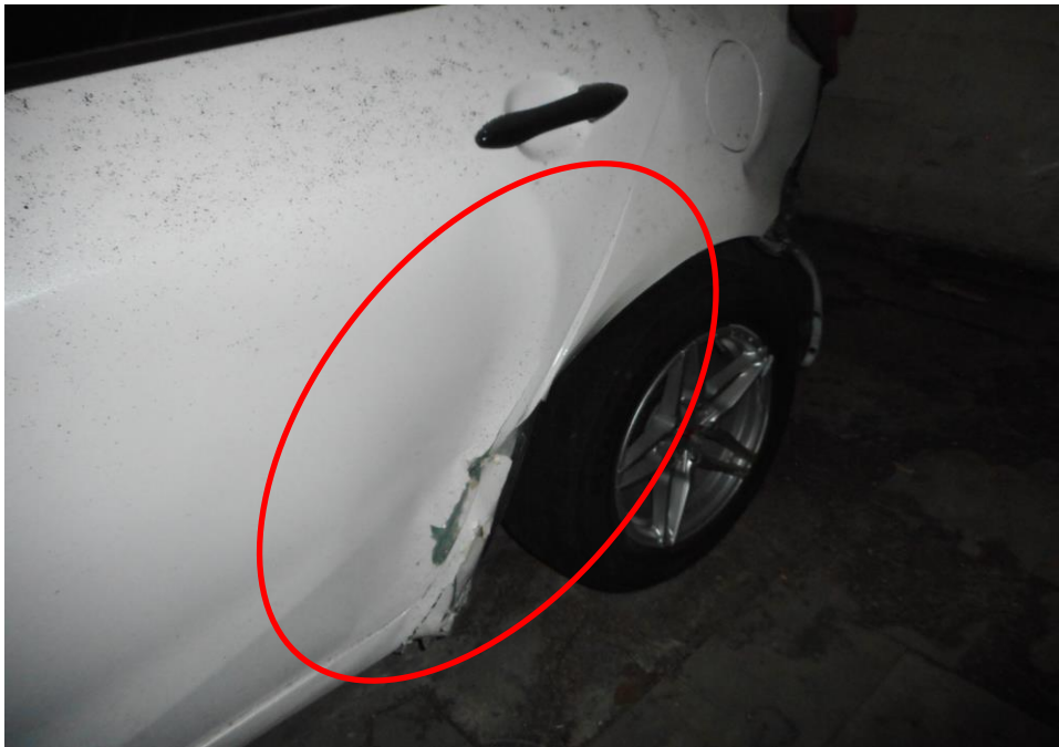
Photo 12 shows the close up view of the Motor Car's left body at the time of my inspection. The Motor car was observed to have sustained damage at its left portion. Its left body panel (circled) was damaged as a result of the accident.
