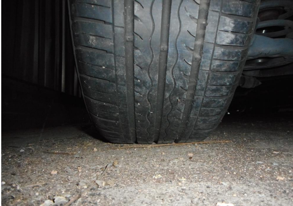
Photo 15 shows the condition of the rear left tyre of the Motor Car, which was observed to be in serviceable condition with remaining tread depth of approximately 4.6mm. The tyre was also observed to be sufficiently inflated for vehicular operation with no tear, cut or burst mark(s).
