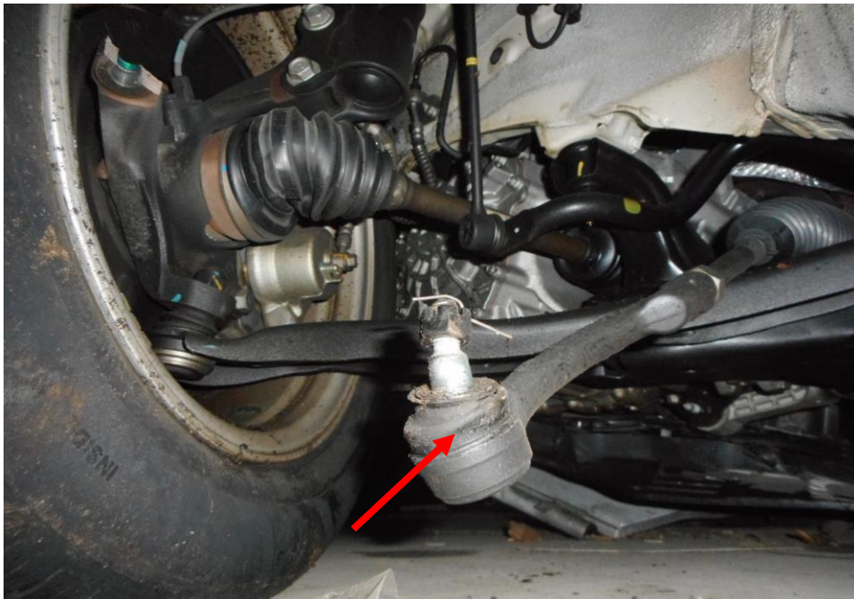
Photo 24 shows the various undercarriage components at the front left wheel of the Motor Car, in particular the steering tie rod end (arrow) was observed to be damaged as a result of the accident.
