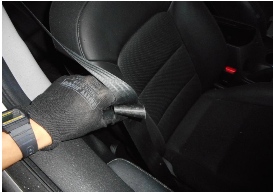
Photo 25 shows that that the seat belt on the right seat was worn at the material time of accident as the safety pre-tensioners was activated at the moment of impact and caused the seat belt to be locked into the last position.
