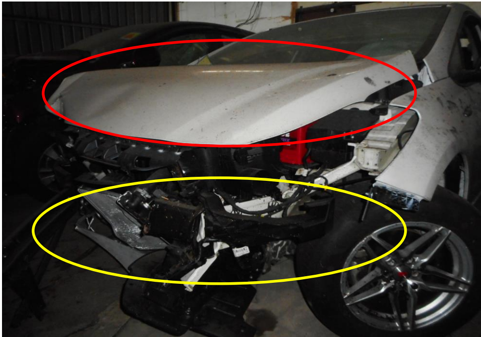
Photo 6 shows the close up view of the Motor Car's front body at the time of my inspection. Its front bonnet (red circle) and front bumper (yellow circle) was amongst the body parts and various components in the engine compartments were also damaged as a result of the accident.
